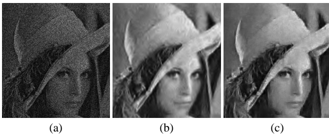
Fig. 3: Results on Lena image with peak intensity 10 and simulated Poisson noise. Close-up of: (a) Noisy image (PSNR=12.96). (b) HF-SureShrink result (PSNR=26.29). (c) Our PH-HMT result (PSNR=27.21).
