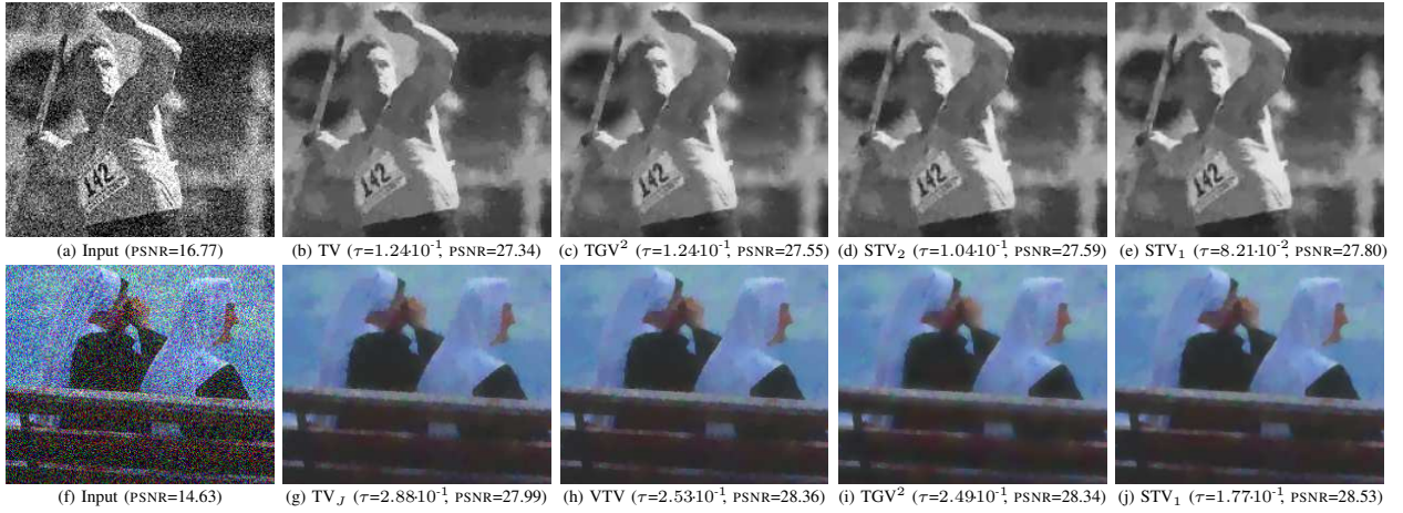
Figure 4. Image denoising examples: close-ups of inputs and optimum results. Top row: grayscale denoising of an input with noise level \sigma_w = 0.15 . The ground truth corresponds to the grayscale version of the image in row 1, column 4 of Fig. 2. Bottom row: color denoising of an input with noise level \sigma_w = 0.2 . The ground truth corresponds to the image in row 3, column 7 of Fig. 2. For each result, the individualized regularization parameter \tau and corresponding optimum PSNR are reported. .
