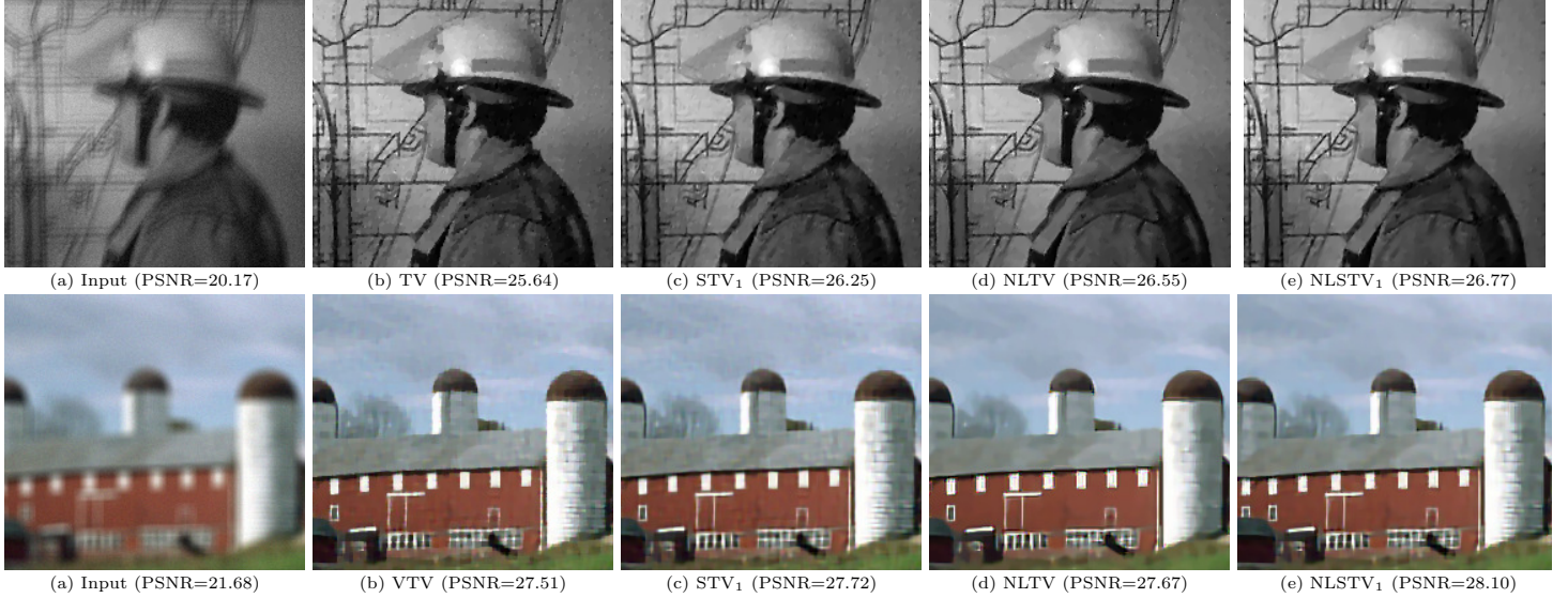
Fig. 4. Image deblurring examples. Close-ups of blurred and noisy inputs and their corresponding deblurred versions. Top row: grayscale deblurring of input image degraded by motion blur and noise level of BSNR=20 dBs. Bottom row : color deblurring of input image degraded by Gaussian blur and noise level of BSNR=25 dBs.
