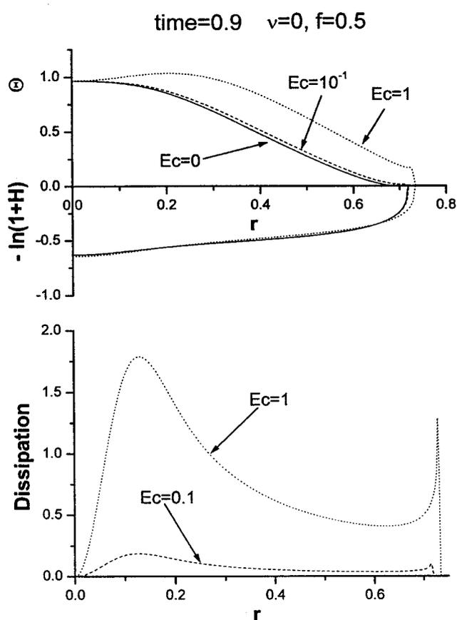
FIG. 7. The temperature, the logarithm of the height and the dimensionless shear heating as a function of the radius. The time is taken in the long time regime. Constant viscosity is used with a  $f=0.5$  (equal partitioning between thermal and compositional buoyancy). A constant flux condition is imposed. Same grid is used as in the constant volume cases.
