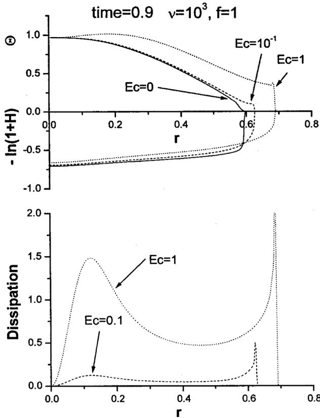
FIG. 9. Same as for Fig. 8, except a temperature-dependent viscosity with  $\nu=10^3$  and a chemically dominated flux ( $f=1$ ) is imposed.
