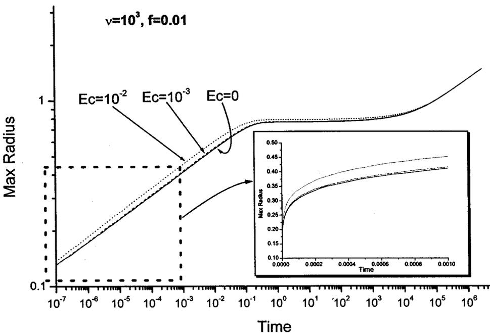
FIG. 6. The evolution of the maximum radial extent of the current with time. Viscosity is temperature-dependent with  $\nu=10^3$  and the forcing is primarily thermal,  $f$  being 0.01. Inset shows the initial stages. Constant volume condition is employed.
