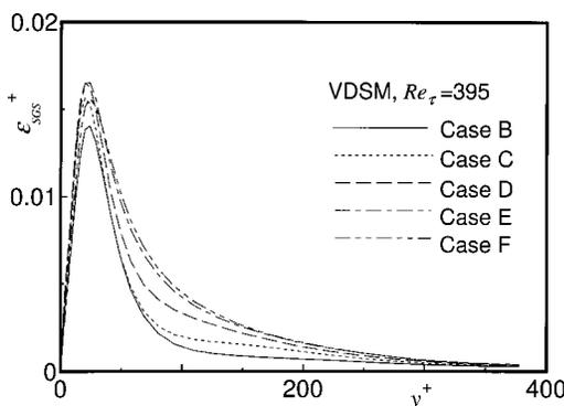
FIG. 11. The effect of grid resolution on the SGS dissipation of the GS turbulence energy for the channel flow at  $Re_\tau = 395$  using VDSM.
