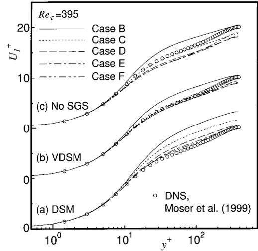
FIG. 5. The effect of grid resolution on the mean streamwise velocity profile for the channel flow at  $Re_\tau=395$  using DSM, VDSM, and No SGS.
