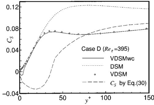
FIG. 3. The profiles of the model parameter  $C_s$  for the channel flow simulation at  $Re_\tau=395$  (case D) using VDSMwc, DSM, and VDSM. The  $C_s$  value computed by Eq. (30) is also plotted.
