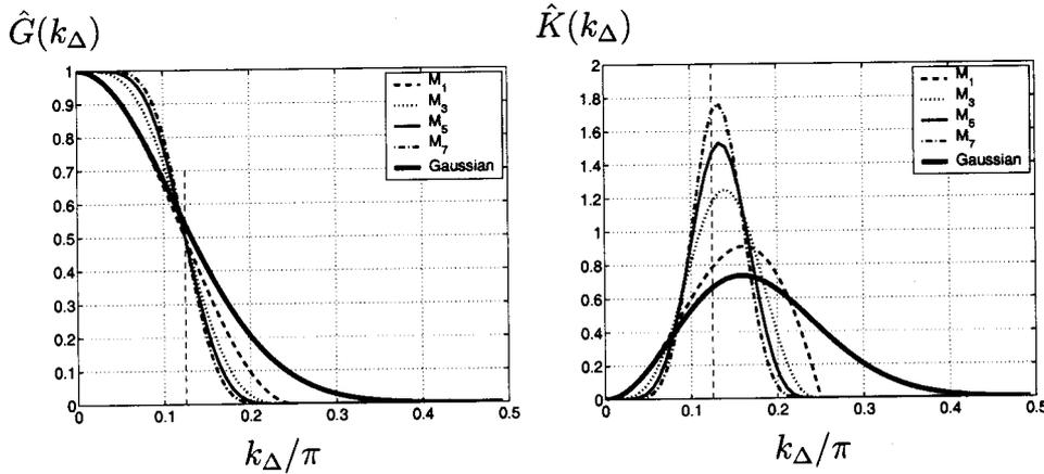
FIG. 1. Transfer functions  $\hat{G}(k_\Delta)$  and  $\hat{K}(k_\Delta)$  for a variety of filters.  $M_n$  denotes the discrete filter with  $n$  vanishing moments.
