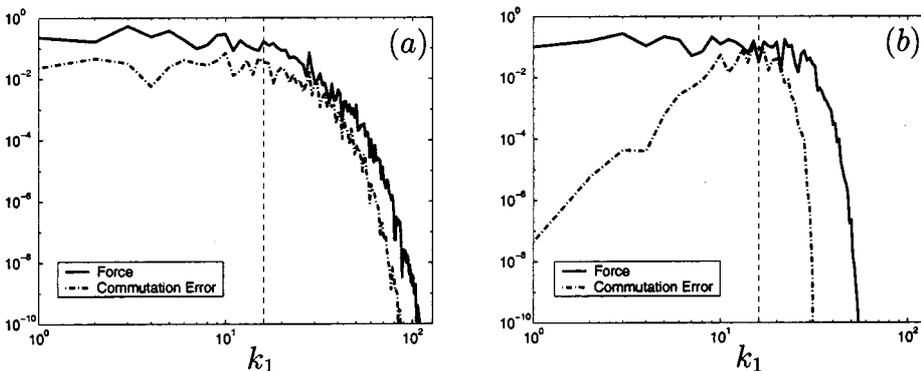
FIG. 2. Global one-dimensional spectrum of the exact SGS force,  $\partial\tau_{11}/\partial x_1$ , and *local* one-dimensional spectrum of the commutation error,  $[\partial u_1^2/\partial x_1]$ , for forced isotropic turbulence at  $Re_\lambda=168$  for (a) Gaussian and (b)  $M_7$  filters.
