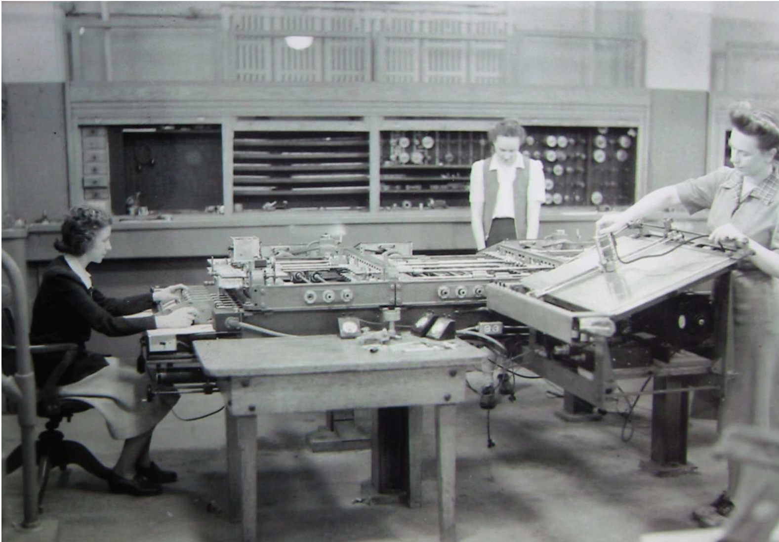
Figure 1: Differential analyzer operated by 3 ladies at the Moore school of Electrical Engineering, University of Pennsylvania, circa 1942 (see wikipedia).
