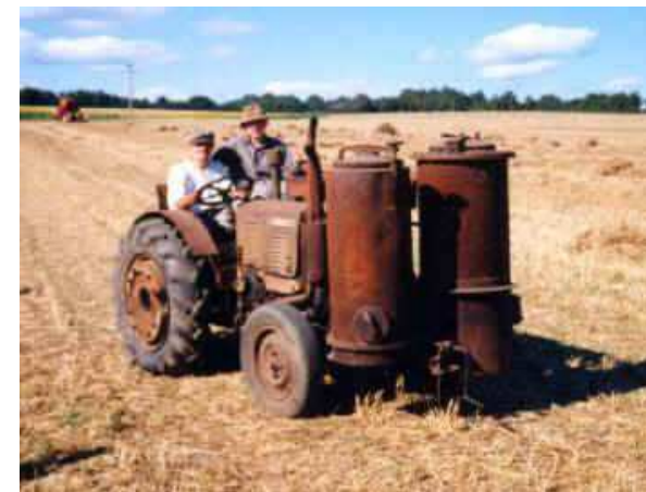
Renault AFVH with a Gasifier Imbert [1941-45]. This tractor was started with gasoline.
