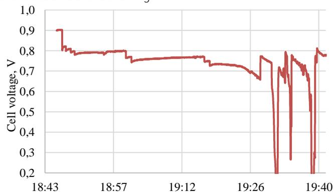
Fig. 4. Typical behavior of the last cell in case of flooding
