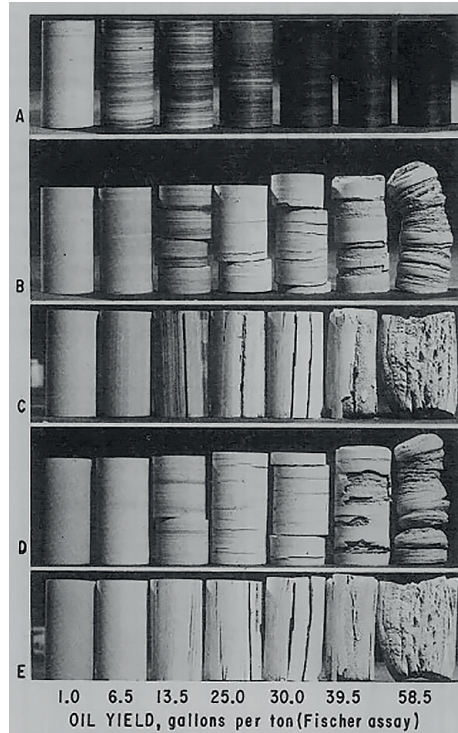
Fig. 1. Structural alterations of samples before and after experiment [7]. A – raw samples; B-C – samples heated to 400° C; D-E – samples heated to 815° C.
