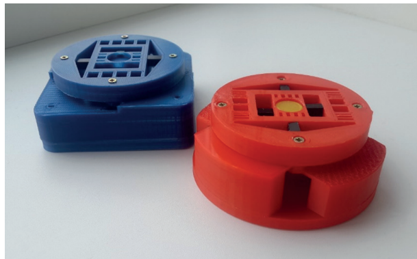
Fig. 9. Photograph of printed and assembled prototypes of the Nanopositioner. Left – semi-finalized design; right – the final design of a Nanopositioner.
