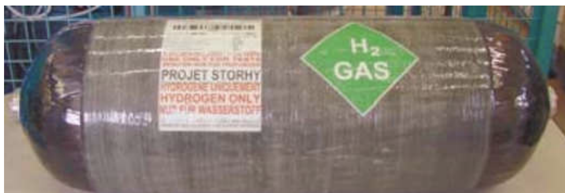
Figure 8. 700 bar hydrogen storage type IV vessel; mass: 28 kg, storage capacity 5.2%wt (21°C)
