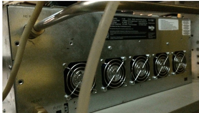
Figure 39. The view of 1 kW Hoppecke 1100 PEM FC with five cooling fans on the back
