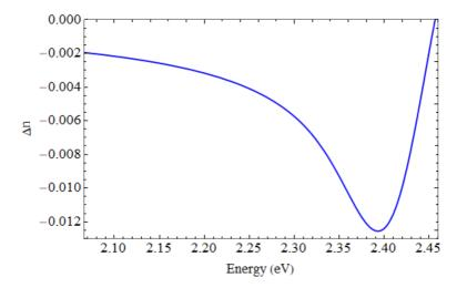
Figure S3. The change in the real part of refractive index  $\Delta n$  versus energy. The induced difference caused by the saturation of molecular optical transitions for 10% of the initial value ( $\xi = 0.1$ ).
