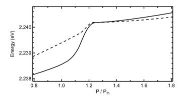
**Figure S5**. The ground polariton state energy versus relative pump power (P/P<sub>th</sub>) simulated numerically using the model with (solid curve) and without intermolecular energy transfer (dashed curve).
