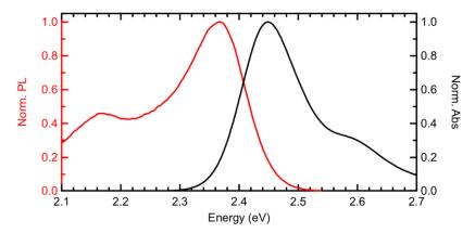
**Figure 4.1**. Normalized absorption (black) and photoluminescence (red) spectra of the bare BODIPY-G1 film of 172 nm thickness.
