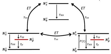
**Figure 4.13**. Schematic of the molecular transitions and relaxation paths of excited states considered within the theoretical model.
