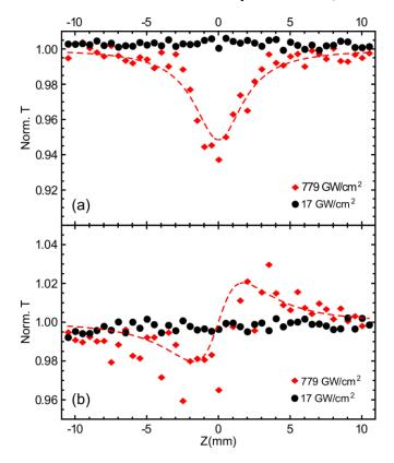
**Figure 4.8**. (a) Open- and (b) closed-aperture Z-scan data of the polystyrene film measured at two different pump energies: 9.5 nJ (black circles) and 438 nJ (red rhombs).
