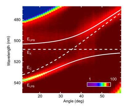
**Figure 2.5**. Angle-dependent reflectivity plot for strongly-coupled microcavity being fitted with coupled harmonic oscillator model. Color bar is the reflectivity scaling. Note, here the sides of the reflectivity stopband are seen in the corners.
