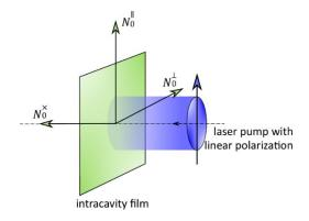
**Figure 4.12**. Schematical representation of the molecules' optical dipole moment alignment and laser polarization relation, considered in frames of the suggested model.
