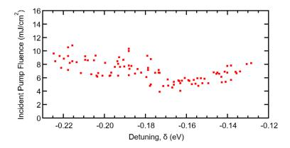
**Figure 3.11**. Polariton lasing threshold dependence versus the exciton-photon detuning. Nearly constant condensation threshold  $\approx (6.5\pm1.5) \text{ mJ cm}^{-2}$  observed across the entire detuning range.
