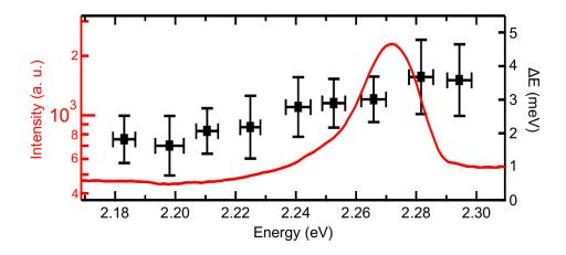
**Figure 4.6**. The ASE spectrum (red, left axes) and the blueshift,  $\Delta E$ . Blueshift was extracted from the binning of scattering plot with Sturge rule (black squares with standard deviation, right axes).
