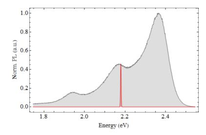
**Figure S4**. The black/grey shaded curve shows the normalized photoluminescence (PL) spectrum of the bare cavity. The red shaded curve shows the part of PL invoked to the population of polariton states in the vicinity to the ground state ( $k_{\rm II} = 0$ ).
