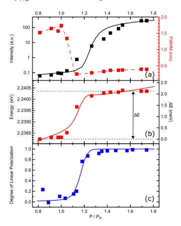
**Figure 4.14**. Solid curves are the numerical simulation for (a) time-integrated photoluminescence, (b) the ground state energy, and (c) degree of linear polarization pump power dependences compared with experimentally extracted data.
