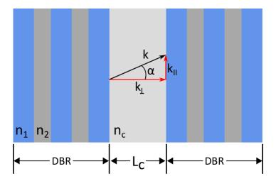
Figure 2.1. Schematic of a planar microcavity which consists of the layer with refractive index  $n_c$  and thickness  $L_c$ , placed between two DBRs. DBRs are composed of two materials of low and high refractive indexes  $n_1$  and  $n_2$ , respectively. Photons are confined inside the cavity with total wavevector  $k_0$  which is a composition of perpendicular  $k_{\perp}$  and parallel  $k_{\parallel}$  parts.
