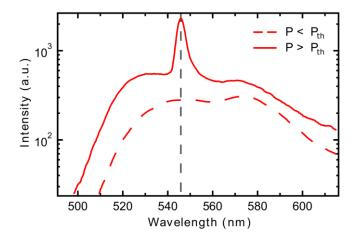
**Figure 3.3**. Emission spectra (dashed) of the bare film under stripe beam excitation. The dye molecules undergo amplified spontaneous emission (solid) at an incident excitation density of  $\approx 5$  mJ cm<sup>-2</sup>, with the maximum of the material gain occurring at 547 nm.
