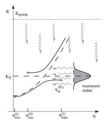
Figure 2.6. Schematic of the relaxation processes in the organic microcavity under non-resonant excitation  $E_{pump}$ . After vibronic relaxation, excitons are forming the reservoir in  $E_0$  and can contribute to the polariton state via further radiative or vibronic relaxation mechanisms. Adopted from [47].
