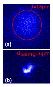
**Figure 3.12**. Real space images of the (a) linear polariton emission below and (b) polariton lasing above the condensation threshold. Red circle corresponds to the excitation pump spot of  $d = 18 \mu m$  diameter at one over  $e^2$  level. Above the threshold, polariton lasing appears from a small area with  $d_{lasing} \approx 6 \mu m$ .
