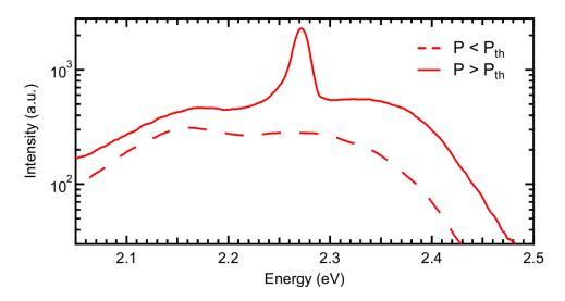
**Figure 4.2**. Amplified spontaneous emission of the neat 172 nm thin film below  $P < P_{th}$  (dashed curve) and above  $P > P_{th}$  (solid curve) amplification threshold of 5.1 mJ cm<sup>-2</sup>.
