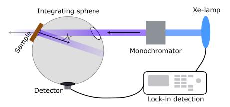
Figure S1. Schematical representation of the reflectance measurement.
