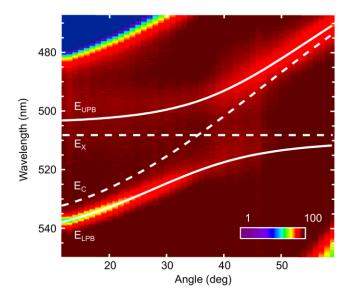
**Figure 3.5**. Angle-dependent reflectivity color plot for the BODIPY-G1 dye-filled microcavity (log scale). The solid lines show the calculated upper and lower polariton branches. The dashed lines correspond to the bare cavity and exciton modes. UPB, LPB, cavity and exciton modes were extracted from the coupled harmonic oscillator model.
