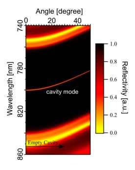
**Figure 2.2**. Angle-dependent reflectivity plot simulated for the empty microcavity. Adopted from [24].
