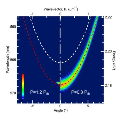
**Figure 3.7**. Normalized E,k - dispersion of polariton photoluminescence below (right) and above (left) the condensation threshold. Red and white dashed curves are attributed to the lower polariton branch and the bare cavity mode, respectively.
