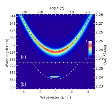
**Figure 2.7**. Polariton dispersions of non-resonantly pumped organic dye-filled microcavity taken below(a) and above(b) the condensation threshold. Above the threshold, initially distributed along the LPB polaritons (dashed line) collapse to the bottom of LPB and form the macroscopic condensate.
