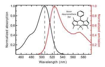
**Figure 3.1**. Normalized absorption (black) and photoluminescence spectrum (red) of a 172 nm thick film from the BODIPY-G1 dye dispersed into a polystyrene matrix. Inset is the chemical structure of BODIPY-G1.
