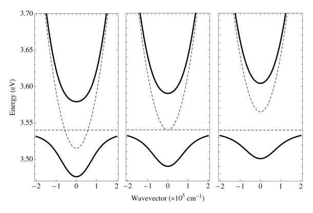
**Figure 2.4**. Energetic distribution of exciton-polariton modes at negative, zero and positive detunings (from left to right). Solid lines correspond to exciton-polariton modes dispersions, dashed – to the bare exciton and photon modes. The figure is adopted from [23].
