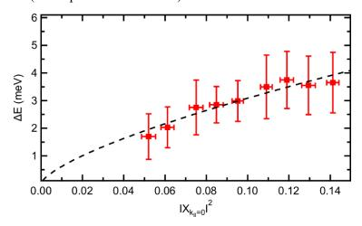
**Figure 4.10**. The blueshift,  $\Delta E$ , versus exciton fraction. The dependence of the blueshift on the exciton fraction is calculated by binning the scattering plot (section 4.3.1) and taking into account the dependence of exciton fraction on the ground polariton state energy (Figure 4.9(d)). The dashed black line is the best-fit result by power-law
