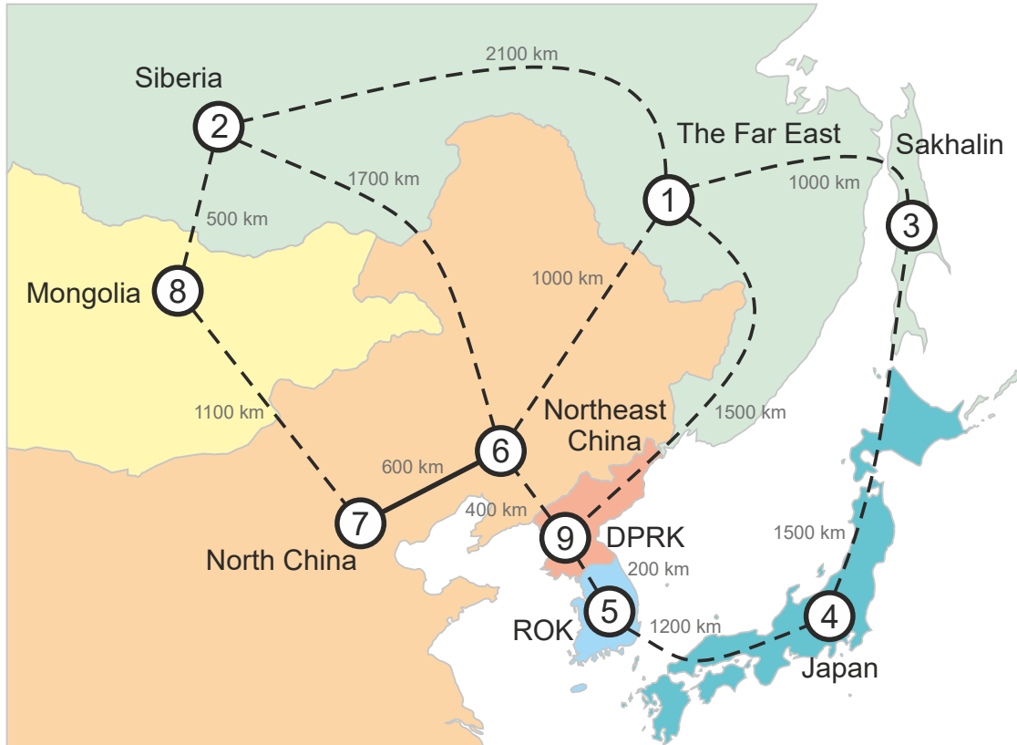
Figure 6.1: Scheme of potential cross-border power interconnections in Northeast Asia.
