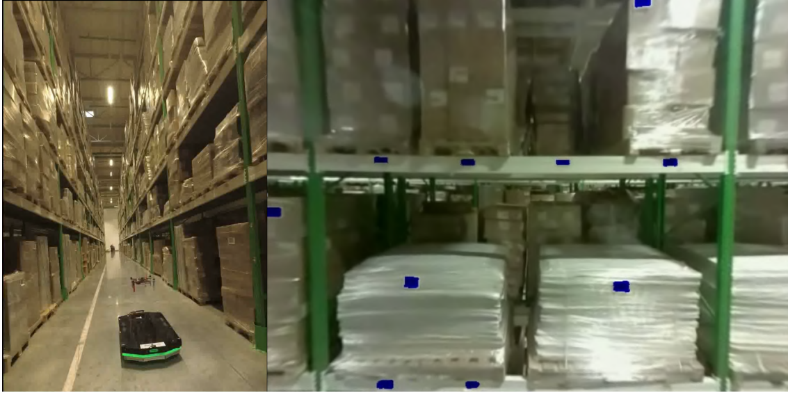
Figure 7-12: Stocktaking process with the proposed heterogeneous robotic system. At the right side is working system. At the left side is recognized image frame from the UAV camera.
