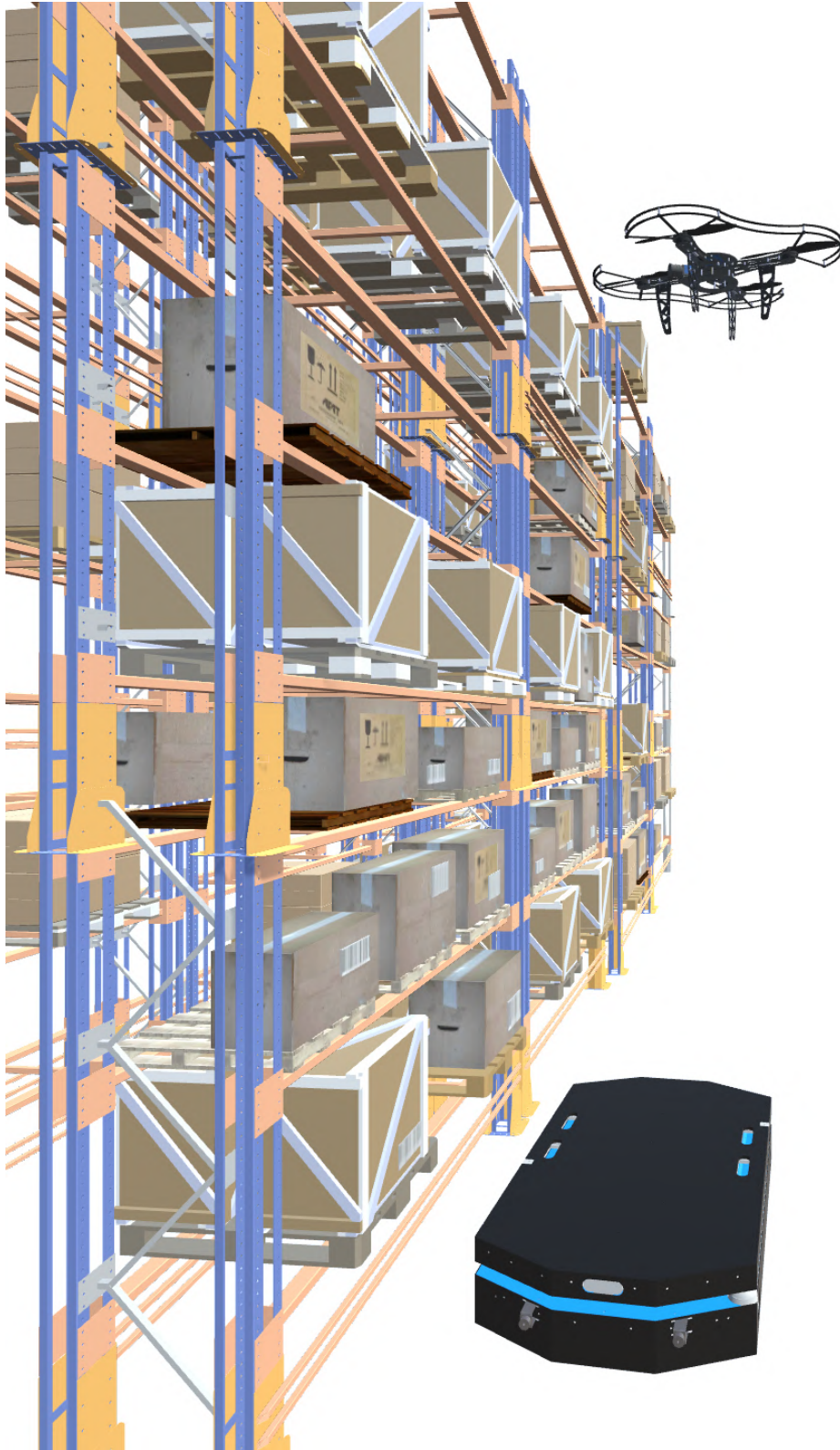
Figure 4-10: Visualisation of the UAV flight above the UGV near one rack in the warehouse digital twin.
