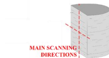
Figure 1 Scheme of the orientation of scanning lines during thermal core logging.
