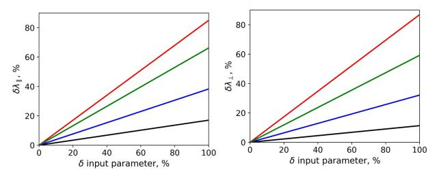
**Figure 17**. Results of assessing influence of uncertainty in thermal conductivity of rock matrix (red lines), porosity (green line), thermal conductivity of pore fluid (blue line), and correction factor (black line) on rock thermal conductivity for parallel (left panel) and perpendicular (right panel) directions to the bedding plane.
