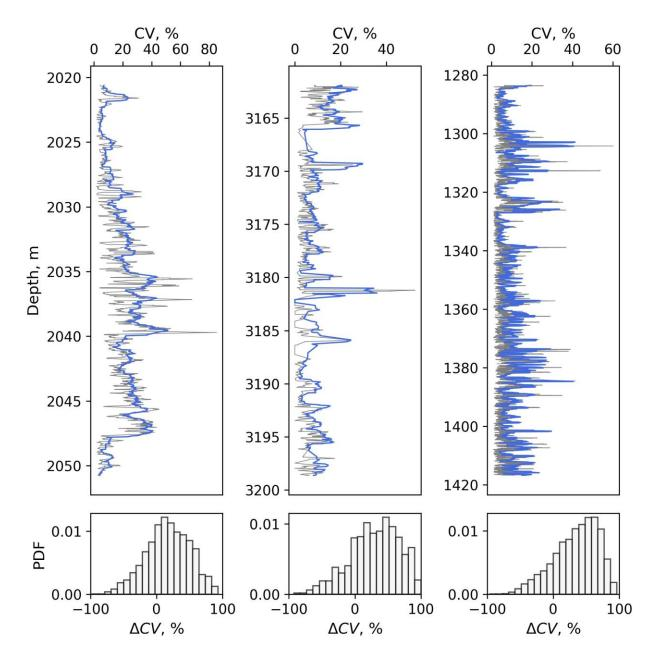
**Figure 1.** Results of calculating CV for two organic-rich shales (left and central panel) and carbonate rocks of heavy oil field (right panel) within moving windows of 0.1 m (grey coloured line) and 0.5 m (blue) coloured line. Histograms plot relative difference between CV calculated within 0.5 m and CV calculated within 0.1 m.
