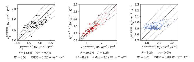
**Figure 6.** Results of prediction of thermal conductivity for parallel (left panel) and perpendicular (central panel) direction to the bedding plane from sonic velocity and rock volumetric heat capacity from photoelectric factor (right panel).
