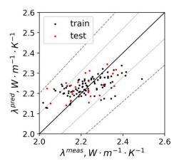
**Figure 35**. The cross-plot of measured and predicted values of thermal conductivity parallel to the bedding plane.
