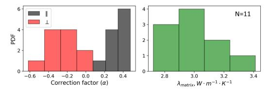
**Figure 33**. The histogram of the determined correction factors for parallel (black colour) and perpendicular (red colour) directions to the bedding plane and thermal conductivity of rock matrix (right panel).
