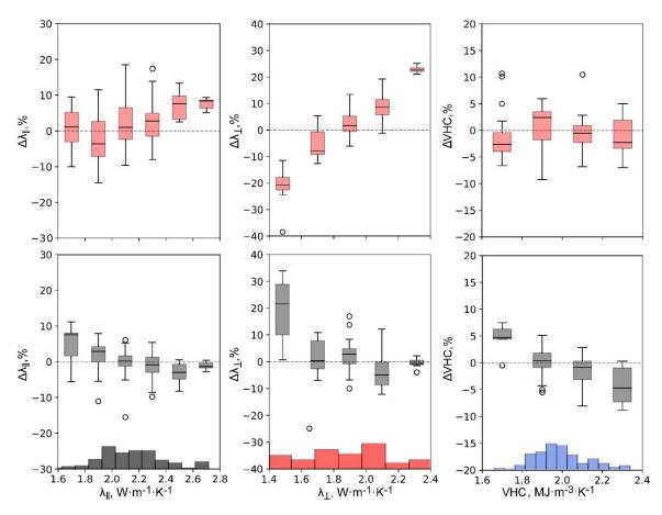
**Figure 25**. Boxplots of the relative discrepancies between the measured and predicted values of rock thermal properties for the Domanic Formation. Above, predictions based on the theoretical models; below, predictions based on the gradient boosting algorithm. Histograms of thermal properties from the test dataset are also shown.
