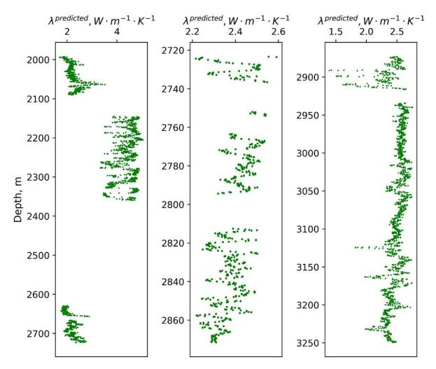
**Figure 43**. The results of predicting rock thermal conductivity within non-coring depth intervals from well-logging data via the established regression equations.
