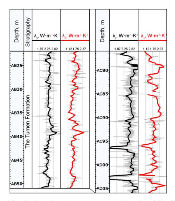
**Figure 14**. Results of rock thermal property measurements for wells A (left) and C (right).  $\lambda$  stands for rock thermal conductivity; subscripts  $\|$  and  $\bot$  stand for the thermal conductivity components in the directions parallel and perpendicular to the bedding plane, respectively; grey lines represent the original profiles of the rock thermal properties; black, red and blue lines represent averaged thermal property profiles in a moving 0.5 window.
