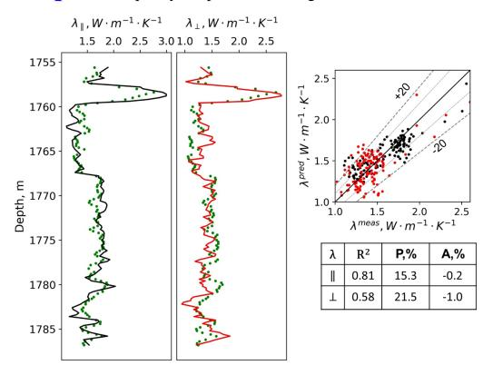
**Figure 34**. The results of predicting the thermal conductivity of rocks and assessment of prediction quality for the Vikulov Formation. Black and red curves (left panel) represent measured values of thermal conductivity for parallel and perpendicular directions to the bedding plane, respectively. Green dots represent the predicted thermal conductivity. Prediction quality is reported for a 0.95 confidence level.
