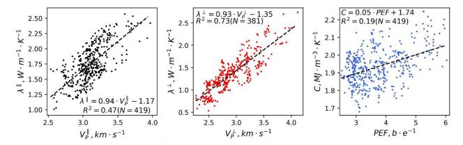
**Figure 5.** Results of correlation analysis between thermal conductivity and sonic velocity of rocks for parallel (left panel) and perpendicular (central panel) direction to the bedding plane and rock volumetric heat capacity and photoelectric factor (right panel). Dashed line represents the regression trend.
