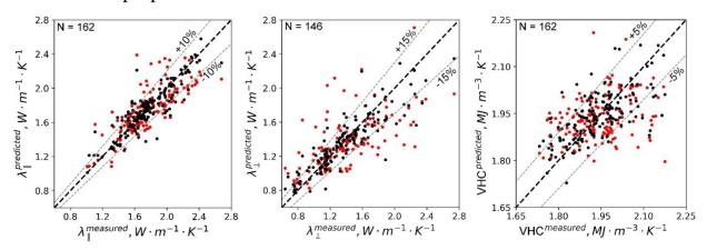
**Figure 11**. Experimental data of the rock thermal properties compared to the thermal properties predicted from well-logging data of training datasets for the Bazhenov Formation. Black dots present results with the gradient boosting method, red dots results via theoretical model. The dashed black line (y=x) shows a perfect prediction.
