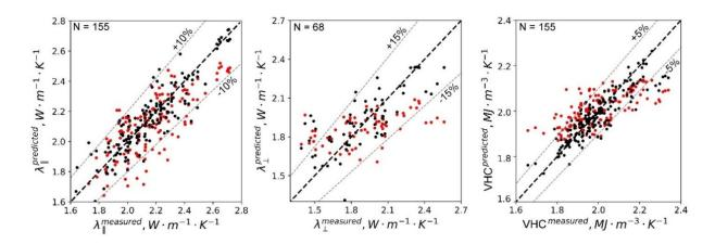
**Figure 24**. Experimental data of the rock thermal properties compared to the thermal properties predicted from well-logging data of training datasets for the Domanic Formation. Black dots present results with the gradient boosting method, red dots results via theoretical model. The dashed black line (y=x) shows a perfect prediction.
