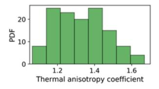
**Figure 15**. Histogram of thermal anisotropy coefficient inferred from thermal core logging for wells A and C.
