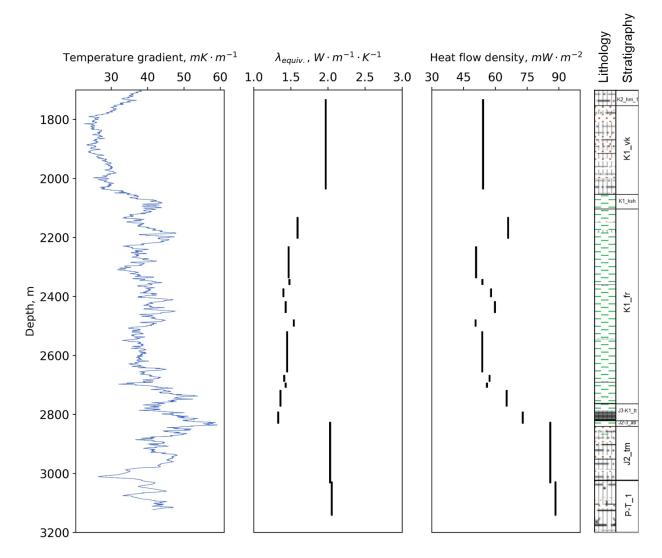
**Figure 38**. Results of determining temperature gradient, equivalent thermal conductivity of rocks and the heat flow density within 14 depth intervals. Lithology legend was given in Figure 37 (Popov et al., 2021a).
