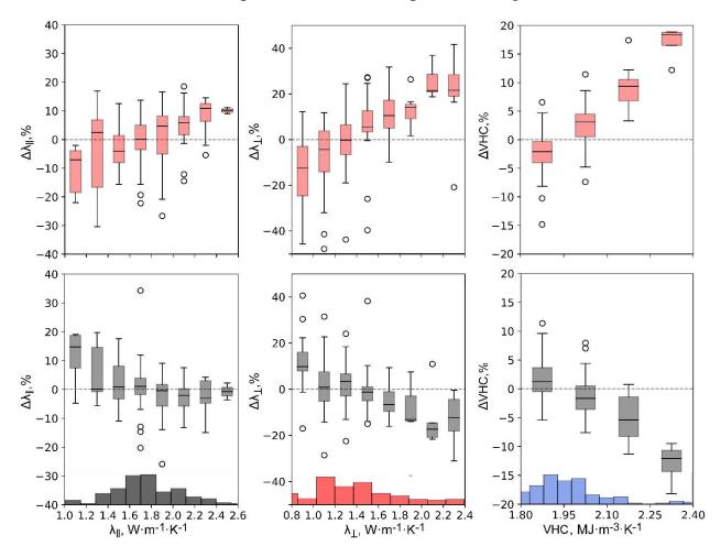
**Figure 12**. Boxplots of the relative discrepancies between the measured and predicted values of rock thermal properties for the Bazhenov Formation. Above, predictions based on the theoretical models; below, predictions based on the gradient boosting algorithm. Histograms of thermal properties from the test dataset are also shown.
