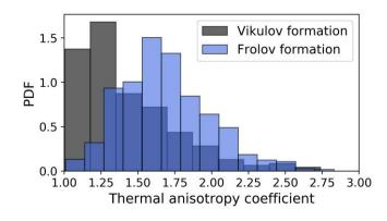
**Figure 32**. The histogram of thermal anisotropy coefficient for the Vikulov (black colour) and the Frolov (blue colour) formations.
