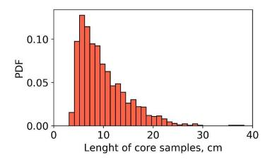
**Figure 40**. Distribution histogram for the length of full-sized cores under study (Popov et al., 2021b).
