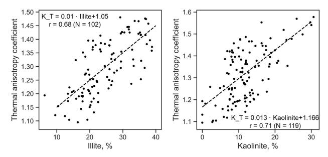
**Figure 26**. Cross-plots between thermal anisotropy coefficient and illite volume fraction (left panel) and thermal anisotropy coefficient and kaolinite volume fraction (right panel). The dashed lines represent the regression trend.
