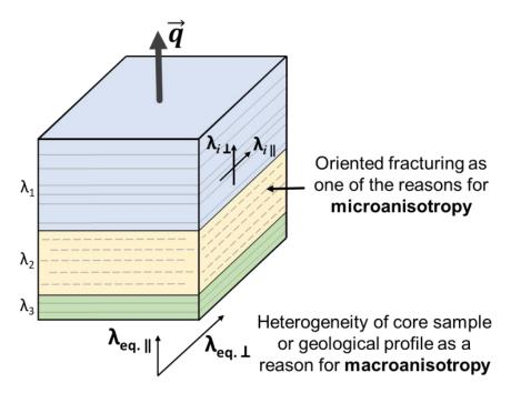
**Figure 44**. The reasons causing anisotropy of rocks that were accounted during determining equivalent thermal conductivity required for calculating heat flow density.  $\lambda$ eq. – macroanisotropy,  $\lambda_{i\perp}$  - microanisotropy (Popov et al., 2021b).
