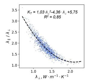
**Figure 36**. The cross-plot of thermal anisotropy coefficient and thermal conductivity perpendicular to the bedding plane.
