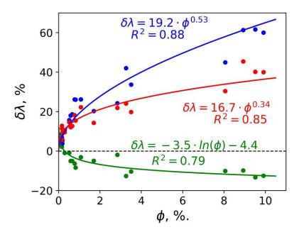
**Figure 42**. The dependence of thermal conductivity variations from porosity of core samples after drying core samples (green-coloured line) and after water saturating (under vacuum) the dried core samples (blue-coloured line) (Popov et al., 2021b). The red-coloured line characterizes the thermal conductivity change from «as received» state to «water-saturated».
