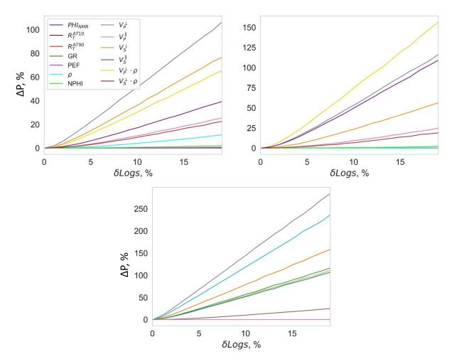
**Figure 10.** Results of sensitivity study of regression models of gradient boosting for determining thermal conductivity parallel (left panel) and perpendicular (right panel) to bedding plane and volumetric heat capacity (bottom panel) of carbonate rocks of heavy oil field.
