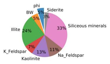
**Figure 13**. Pie chart of average volume fractions of rock-forming components of the investigating rocks inferred from high definition spectroscopy and NMR log data.
