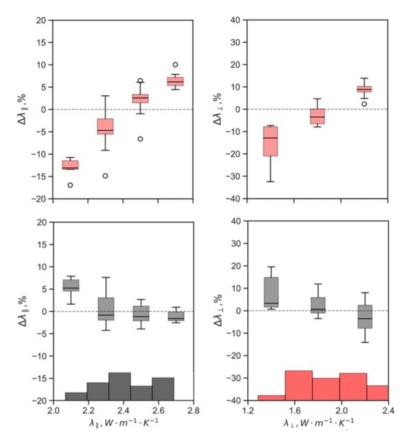
**Figure 28**. Boxplots of the relative discrepancies between the measured and predicted values of rock thermal conductivity for the investigating clayous rocks. The upper panel represents the boxplots for predictions that are made via the Deming correction approach. The lower panel represents the boxplots for predictions that are made via the gradient boosting regression models. Histograms of thermal conductivities for the test dataset are also shown.
