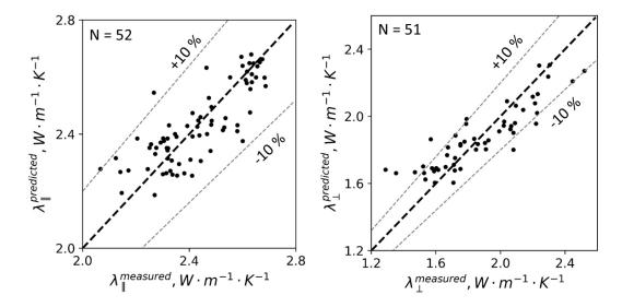
**Figure 16**. Experimental data of the rock thermal conductivity compared to the predicted thermal conductivity from well-logging data on test datasets. The dashed black line (y=x) shows perfect prediction. N stands for number of points.
