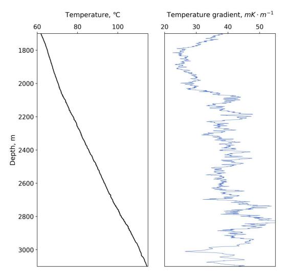
Figure 31. The temperature and temperature gradient along the well.
