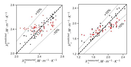
**Figure 27**. Experimental data of the rock thermal conductivity compared to the thermal conductivity predicted from well-logging data of test datasets for the investigating clayous rocks. Black dots present results with the gradient boosting method, red dots results via the Deming approach. The dashed black line (y=x) shows perfect prediction.
