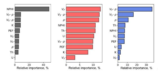
**Figure 23**. Well log importance during predicting rock thermal properties assessed via noise-based perturbation importance ranking method for the Domanic Formations. Black corresponds to thermal conductivity parallel to the bedding plane, red coloured diagram corresponds to thermal conductivity perpendicular to the bedding plane, and blue coloured diagram corresponds to rock volumetric heat capacity.
