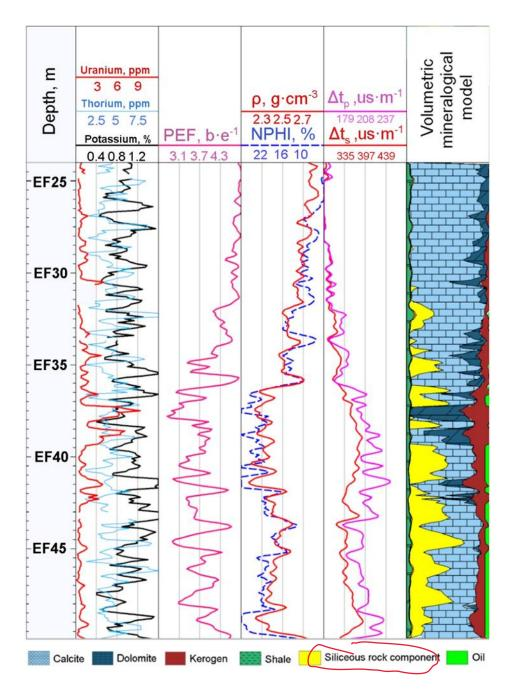
Figure 20. Results of well-logging for well G. Log symbols were defined in the text above.
