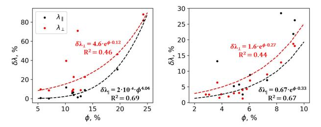
**Figure 30**. The dependency of relative increase of thermal conductivity after water saturation from porosity for the Vikulov and Frolov formations (left panel) and for the Abalak and Tyumen formations (right panel). Red colored dots and regression trend represent data for thermal conductivity perpendicular to the bedding plane. Black colored dots and regression trend represent data for thermal conductivity parallel to the bedding plane.
