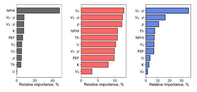
**Figure 23**. Well log importance during predicting rock thermal properties assessed via noise-based perturbation importance ranking method for the Domanic Formations. Black corresponds to thermal conductivity parallel to the bedding plane, red coloured diagram corresponds to thermal conductivity perpendicular to the bedding plane, and blue coloured diagram corresponds to rock volumetric heat capacity.
