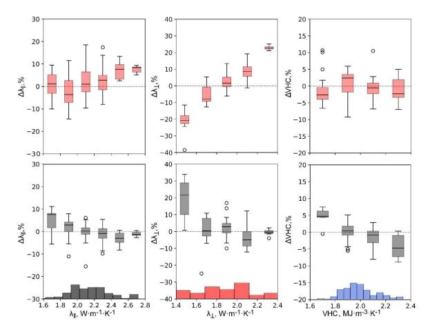
**Figure 25**. Boxplots of the relative discrepancies between the measured and predicted values of rock thermal properties for the Domanic Formation. Above, determinations based on the theoretical models; below, determinations based on the gradient boosting algorithm. Histograms of thermal properties from the test dataset are also shown.
