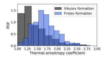
**Figure 33**. The histogram of thermal anisotropy coefficient for the Vikulov (black colour) and the Frolov (blue colour) formations.
