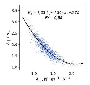
**Figure 37**. The cross-plot of thermal anisotropy coefficient and thermal conductivity perpendicular to the bedding plane.
