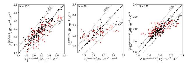
**Figure 24**. Experimental data of the rock thermal properties compared to the thermal properties predicted from well-logging data of training datasets for the Domanic Formation. Black dots present results with the gradient boosting method, red dots results via theoretical model. The dashed black line (y=x) shows a perfect determination.
