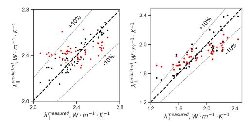
**Figure 27**. Experimental data of the rock thermal conductivity compared to the thermal conductivity predicted from well-logging data of test datasets for the investigating clayous rocks. Black dots present results with the gradient boosting method, red dots results via the Deming approach. The dashed black line (y=x) shows perfect determination.
