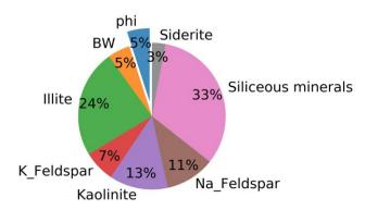
**Figure 13**. Pie chart of average volume fractions of rock-forming components of the investigating rocks inferred from high definition spectroscopy and nuclear magnetic resonance log data.
