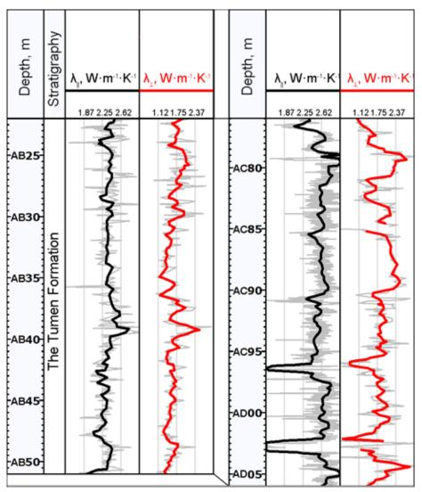
**Figure 14.** Results of rock thermal property measurements for wells A (left) and C (right).  $\lambda$  stands for rock thermal conductivity; subscripts  $\mathbb{I}$  and  $\bot$  stand for the thermal conductivity components in the directions parallel and perpendicular to the bedding plane, respectively; grey lines represent the original profiles of the rock thermal properties; black, red and blue lines represent averaged thermal property profiles in a moving 0.5 window.
