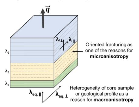
**Figure 46**. The reasons causing anisotropy of rocks that were accounted during determining equivalent thermal conductivity required for calculating heat flow density.  $\lambda$ eq. – macroanisotropy,  $\lambda$ <sub>i⊥</sub> - microanisotropy (Popov et al., 2021b).
