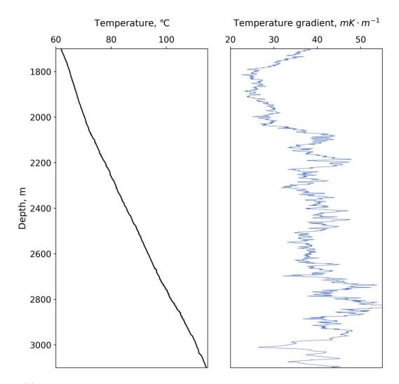
Figure 32. The temperature and temperature gradient along the well.
