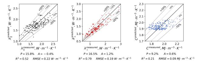
**Figure 6.** Results of determination of thermal conductivity for parallel (left panel) and perpendicular (central panel) direction to the bedding plane from sonic velocity and rock volumetric heat capacity from photoelectric factor (right panel). Solid line presents a perfect determination of rock thermal properties (x=y), grey dashed lines present the determination uncertainty intervals.
