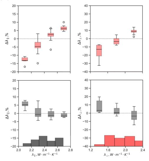
**Figure 28**. Boxplots of the relative discrepancies between the measured and predicted values of rock thermal conductivity for the investigating clayous rocks. The upper panel represents the boxplots for determinations that are made via the Deming correction approach. The lower panel represents the boxplots for determinations that are made via the gradient boosting regression models. Histograms of thermal conductivities for the test dataset are also shown.
