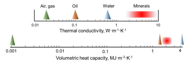
**Figure 2.** Thermal conductivity and volumetric heat capacity for rock-forming minerals and pore fluids.
