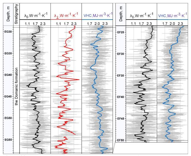
**Figure 22**. Results of rock thermal property measurements for wells F (left) and G (right).  $\lambda$  stands for rock thermal conductivity, subscripts || and  $\bot$  stand for the thermal conductivity components in the directions parallel and perpendicular to the bedding plane, respectively; grey lines represent the original profiles of the rock thermal properties. Black, red and blue lines represent averaged thermal property profiles in a moving 0.5 window.
