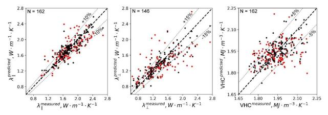
**Figure 11**. Experimental data of the rock thermal properties compared to the thermal properties predicted from well-logging data of training datasets for the Bazhenov Formation. Black dots present results with the gradient boosting method, red dots results via theoretical model. The dashed black line (y=x) shows a perfect determination.
