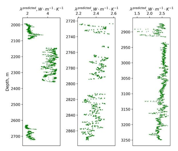
**Figure 45**. Thermal conductivity within not cored depth intervals predicted from well-logging data by means of the established regression equations.
