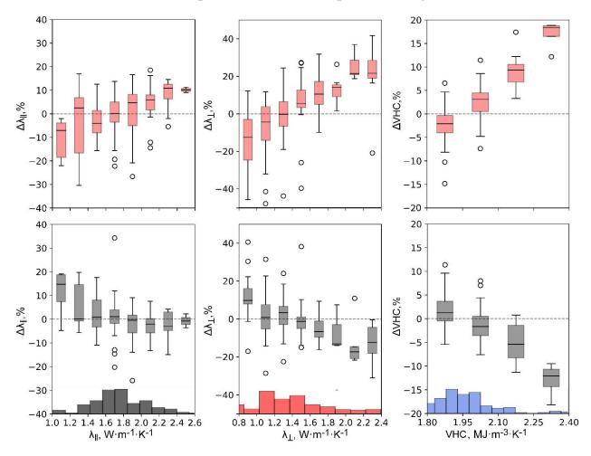
**Figure 12**. Boxplots of the relative discrepancies between the measured and predicted values of rock thermal properties for the Bazhenov Formation. Above, determinations based on the theoretical models; below, determinations based on the gradient boosting algorithm. Histograms of thermal properties from the test dataset are also shown.
