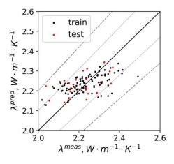
**Figure 36**. The cross-plot of measured and predicted values of thermal conductivity parallel to the bedding plane.
