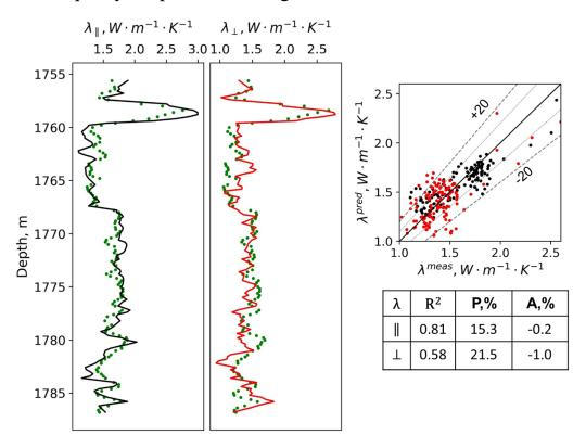
**Figure 35**. The results of predicting the thermal conductivity of rocks and assessment of determination quality for the Vikulov Formation. Black and red curves (left panel) represent measured values of thermal conductivity for parallel and perpendicular directions to the bedding plane, respectively. Green dots represent the predicted thermal conductivity. Determination quality is reported for a 0.95 confidence level.
