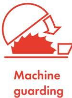
Never remove the machine safety guards from equipment when working with it. Never work with broken guarding or unguarded machines.
