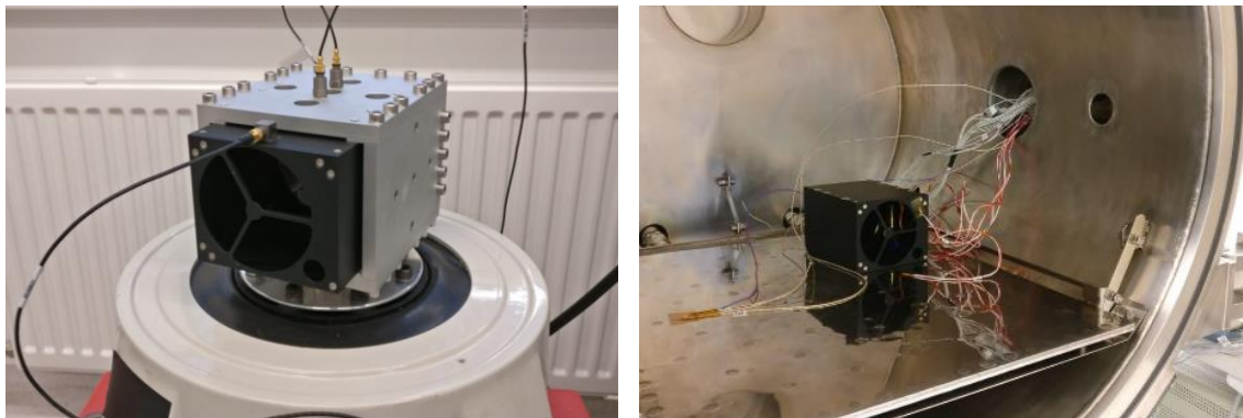
Figure 18. Qualification model vibration test (left), proto-flight model TVAC test (right)
