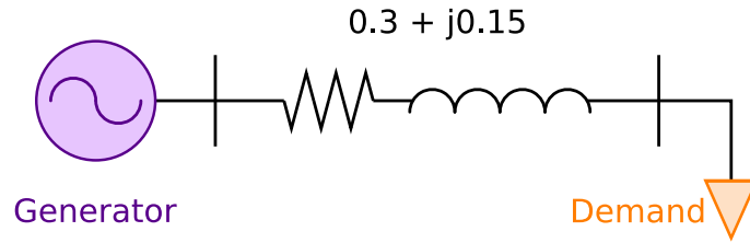
(a) Sample two-node power system.
