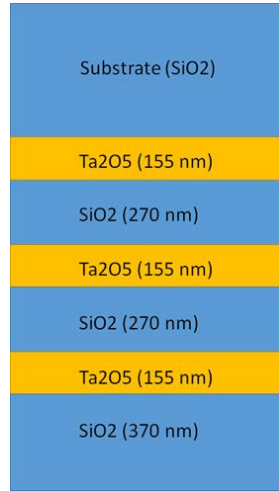
Figure 4-1: The scheme of the photonic crystal providing the resonance at 780 nm.
