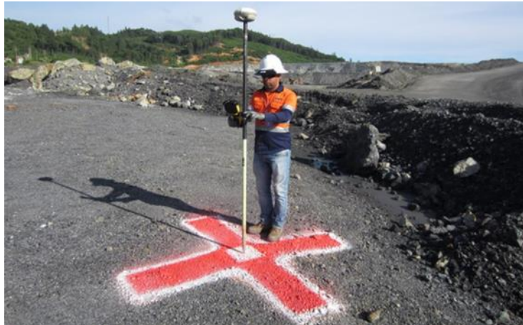
Figure 1-3. Example of fieldwork for GCP surveying (Ground Control Points for Drone Mapping, 2021)
