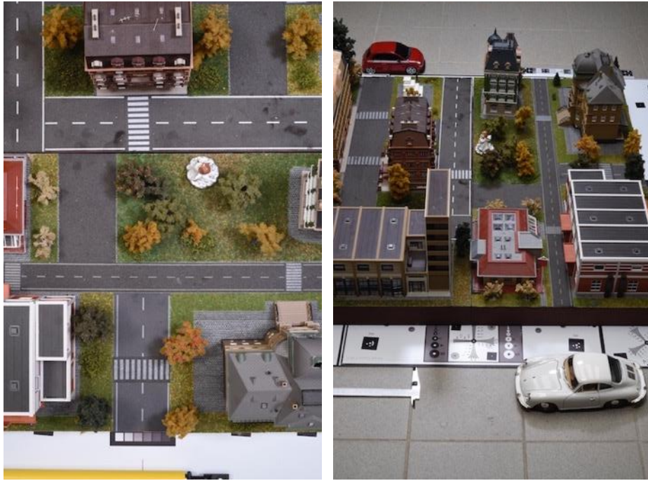
Figure 1-11. Examples for nadir (left) and oblique (right) images from the 3DOMCity benchmark (Özdemir et al., 2019b).
