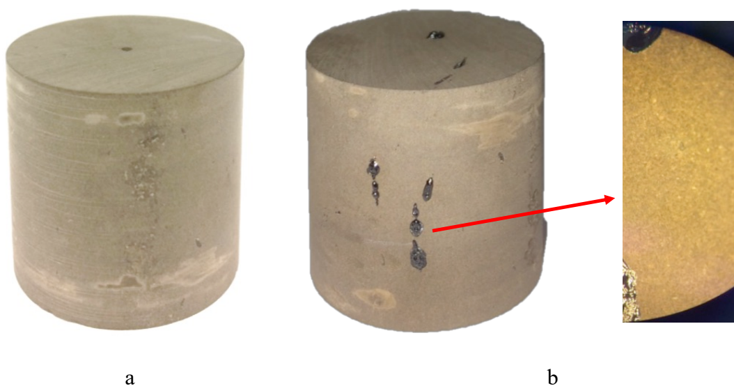
Figure 43. Photo of sample №1 before (a) and after high-temperature measurements with a zoomed area of bitumen exudation (b).
