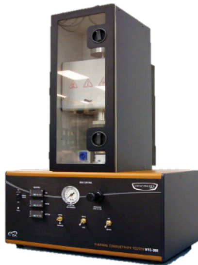
Figure 1. DTC-300 instrument for measuring Thermal conductivity of rock samples at elevated temperatures.
