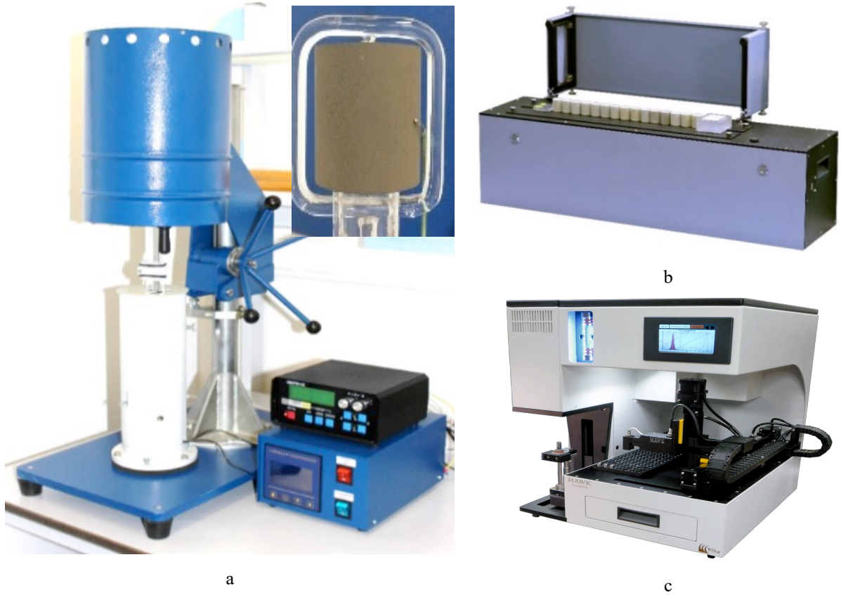
Figure 12. Main (a) and auxiliary equipment (b, c) used in the study; a - Quartz dilatometer with an installed core sample, b - Thermal Conductivity Scanner, c - HAWK pyrolysis instrument.
