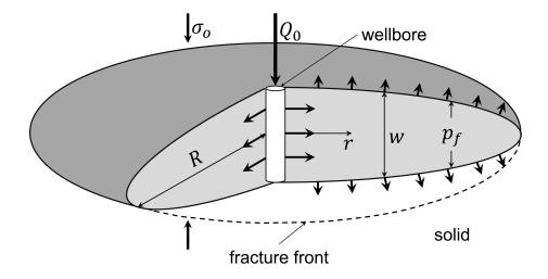
Figure 2-2: A radial fracture model with the classical set of assumptions.
