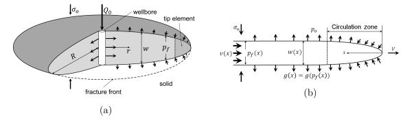
Figure 3-15: A radial fracture model (a) with the pressure-dependent fluid exchange and its near-tip region (b) described by a semi-infinite fracture model.
