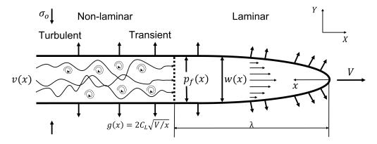
Figure 4-1: Schematics of the fracture-tip model with turbulent flow and leak-off.
