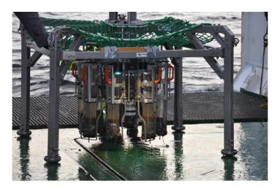
Figure 19. A sampling of bottom sediments by multi-corer sediment.
