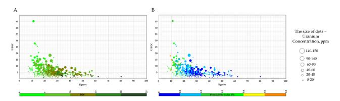
Figure 59. U/TOC - Kgoc<sub>ex</sub> diagram based on pyrolysis studies of 11 wells. The dot color corresponds to the total organic carbon TOC (A) and the productivity index PI (B), the dot size reflects the uranium concentration.
