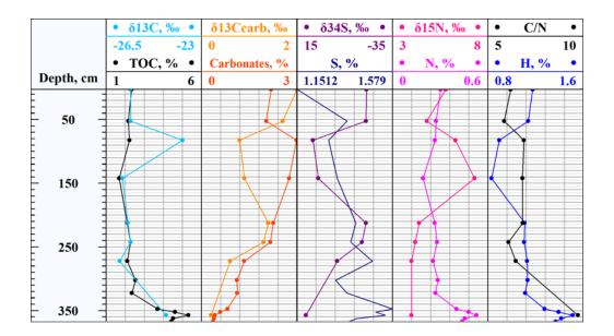
Figure 30. The bottom sediments of station 7. The distributions: H, N, S elements and TOC (analyzer CHN628); isotopy data:  $\delta^{34}$ S,  $\delta^{13}$ C,  $\delta^{13}$ Ccarb,  $\delta^{15}$ N; the ratio C/N.
