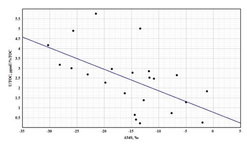
Figure 53. Cross-plot of U/TOC and sulfur isotopic composition for well 1, Bazhenov Formation. Blue line corresponds to equation U/TOC =  $-0.11 \cdot \delta^{34}$ S+0.77, where the correlation coefficient R = 0.57.
