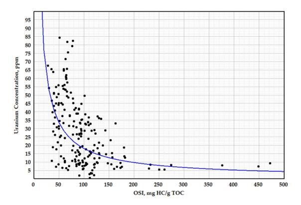
Figure 58. Uranium concentration as a function of oil saturation index (OSI) according to the study of 3 wells drilled at oil fields [Spasennykh и др., 2021] characterized by low maturity kerogen (Kgoc≈55). Blue line corresponds to the equation U = 1133\*OSI<sup>-0.9</sup>, where the determination coefficien R<sup>2</sup> = 0.25.
