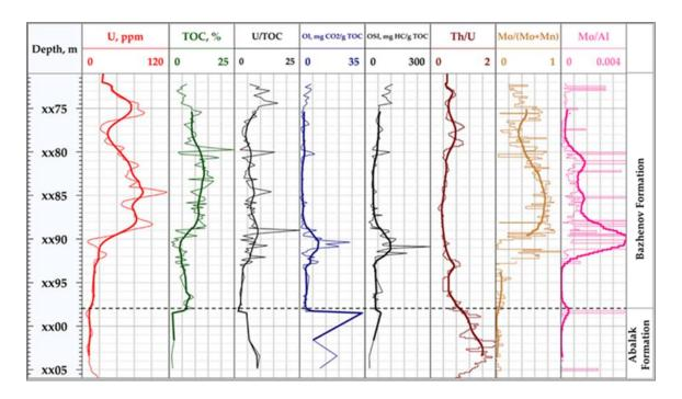
Figure 49. Logview well 2: U and Th/U ratio (gamma-ray spectrometry); TOC is organic matter content, OI is oxygen index, and OSI is oil saturation index (Rock-Eval pyrolysis); U/TOC ratio; Mo/Al and Mo/(Mo+Mn) ratios (XRF analysis).
