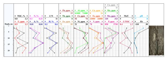
Figure 37. The bottom sediments of station 5. The distributions: H, N, S elements and TOC (analyzer CHN628); U, Pb, Th, Zn, Al, Cr, Ni, Cu, Fe, V, Co, Mo, Mn, P concentrations (ICP-MS); the ratios C/N, U/TOC, and Th/U; also pH and Eh.
