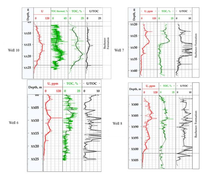
Figure 46. Logviews BF: U-core (gamma spectrometry); TOC – organic matter profile with 1 mm resolution (TOC thermal was determined by the thermal core logging, TOC was determined by the Pyrolysis for Well 10).
