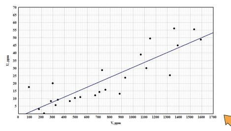
Figure 50. Cross-plot of uranium and vanadium concentrations for well 1, Bazhenov Formation. Blue line corresponds to equation  $U = 0.03 \cdot V - 2.05$ , where the correlation coefficient R = 0.87.
