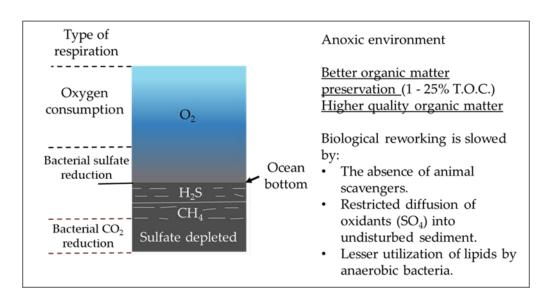
Figure 6. Degradation of organic matter under anoxic water column. Modified after [Demaison, Moore, 1980].
