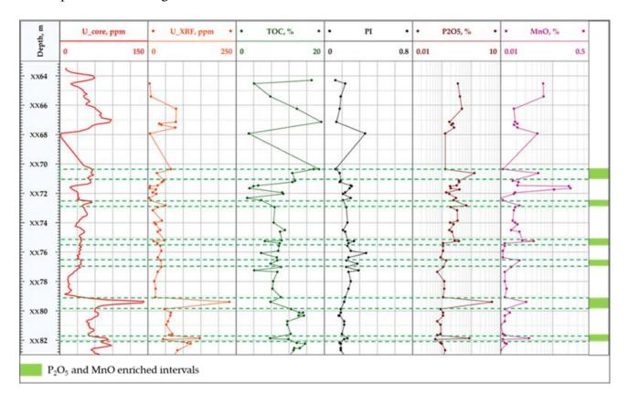
Figure 61. Example of depth distributions of MnO, P<sub>2</sub>O<sub>5</sub>, and uranium concentration (from gamma-ray spectrometry on core samples and XRF), as well as pyrolytic productivity indices (PI) and total organic carbon (TOC).
