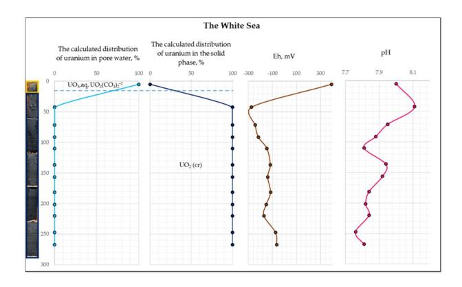
Figure 41. The distribution of the calculated uranium concentration in the pore water and the solid phase of the White Sea bottom sediments for station 1.
