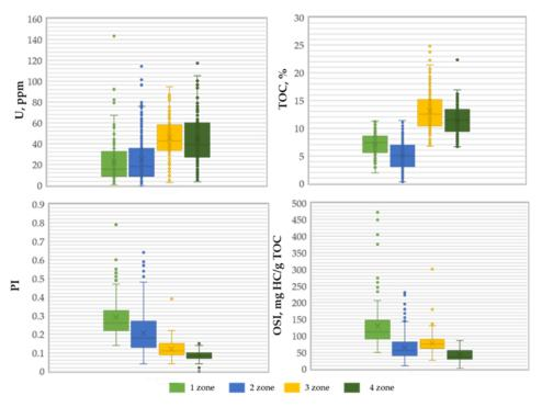
Figure 65. Box-plots for 4 productivity types. Uranium content, TOC, oil saturation, and productivity indices are shown.
