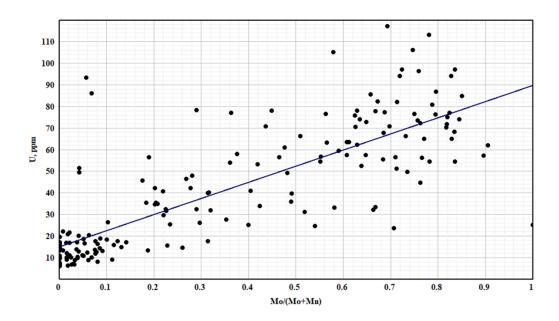
Figure 51. Cross-plot of uranium concentration and Mo/(Mo+Mn) ratio for well 2, Bazhenov Formation. Blue line corresponds to equation U = 74.81·Mo/(Mo+Mn)+14.95, where the correlation coefficient R = 0.81.
