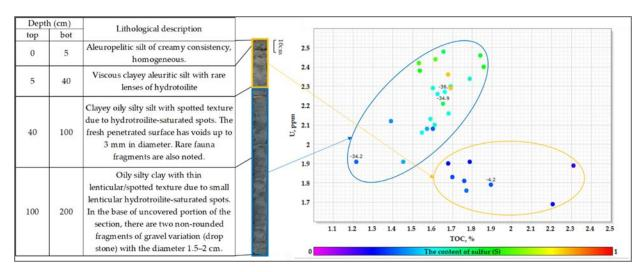
Figure 39. Correlation between the uranium concentration and organic matter content in the bottom sediments of the White Sea for station 2. Above the points, the sulfur isotopic composition ( $\delta^{34}$ S) is indicated. Dot color change is due to sulfur content (S).
