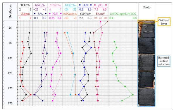
Figure 33. The bottom sediments of station 1. The distributions: H, N, S elements, and TOC (analyzer CHN628); uranium concentration U (ICP-MS); isotopy data:  $\delta^{34}$ S,  $\delta^{13}$ C,  $\delta^{13}$ C<sub>carb</sub>,  $\delta^{15}$ N; the ratios C/N, U/TOC, also pH and Eh.
