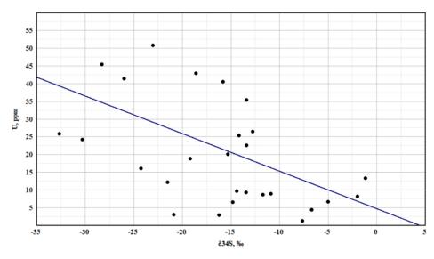
Figure 52. Cross-plot of uranium concentration and sulfur isotopic composition for well 1, Bazhenov Formation. Blue line corresponds to equation  $U = -1.06 \cdot \delta^{34}S + 4.69$ , where the correlation coefficient R = 0.46.
