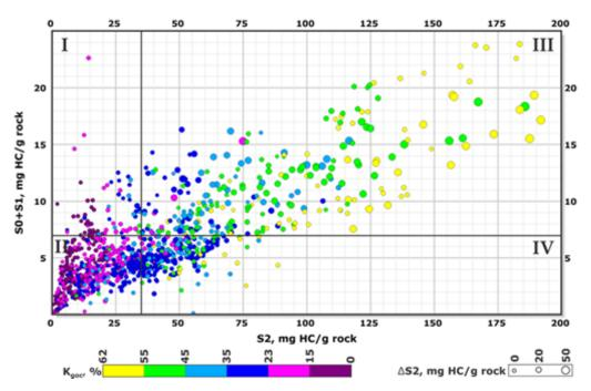
Figure 62. Diagram  $S_0 + S_1$  vs.  $S_2$  [Spasennykh et al., 2021], Quadrants I - IV. The color indicates  $K_{goc}$  the proportion of generative organic carbon in TOC wt.%, and the size of dots reflect  $\Delta S_2$ , mg HC/g TOC.
