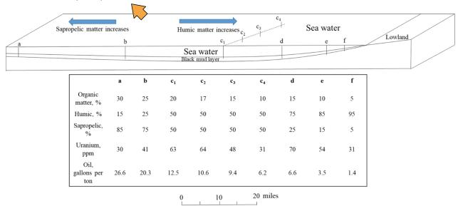
Figure 8. Theoretical humic and sapropelic materials distributions, accumulating organic matter, estimated uranium and oil content in a shallow sea. Modified after [Swanson, 1960].
