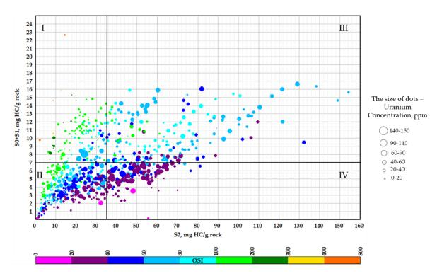
Figure 63. Diagram  $S_0+S_1-S_2$  from core studies of 11 wells. Dot color reflects oil saturation index (OSI), dot size corresponds to the uranium concentration.
