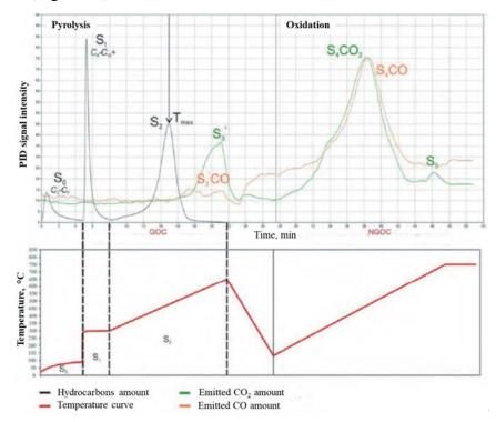
Figure 45. A rock sample pyrogram. Modified after [Vtorushina, Bulatov, 2018].
