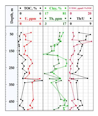
Figure 29. The Black Sea Deep Well. The distributions of the uranium concentration U (natural gamma-ray spectrometry), thorium concentration Th (natural gamma-ray spectrometry), the ratio Th/U, the content of organic matter, and the content of the clay minerals. It was modified after [Neprochnov, 1980].
