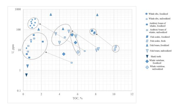
Figure 10. The relationship between the uranium content and organic carbon in bone phosphates. Modified after [Baturin, 2004].
