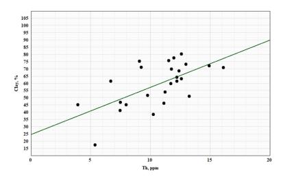
Figure 32. The correlation between the content of clay minerals and thorium concentration for bottom sediments of the Black Sea deep well. Green line corresponds to the equation Clay = 3.26\*Th + 24.52, where the R = 0.61. Modified after [Neprochnov, 1980].
