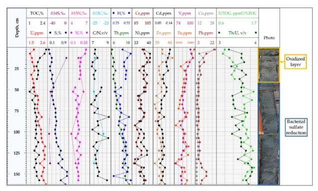
Figure 34. The bottom sediments of station 2. The distributions: H, N, S elements and TOC (analogy CHN628); U, Th, Cr, Ni, Cd, Zn, V, Fe, Co, Pb concentrations (ICP-MS); isotopy data:  $\delta^{34}$ S,  $\delta^{13}$ C,  $\delta^{15}$ N; the ratios C/N, U/TOC, and Th/U.
