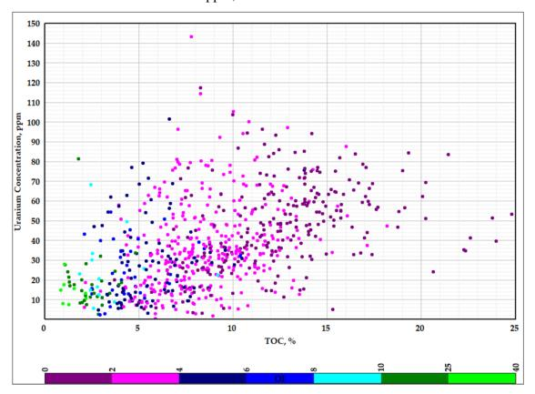
Figure 54. Cross-plot of uranium concentration (measured by gamma-ray spectrometry) and organic matter content (TOC, determined by Rock-Eval pyrolysis) according to the study of 11 wells. Dot color corresponds to oxygen index (determined by Rock-Eval pyrolysis).
