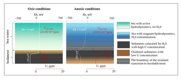
Figure 43. The behavior of uranium in the different redox conditions in the water sea and the bottom sediments (the Arctic Sea (**left**) and the Black Sea (**right**)).
