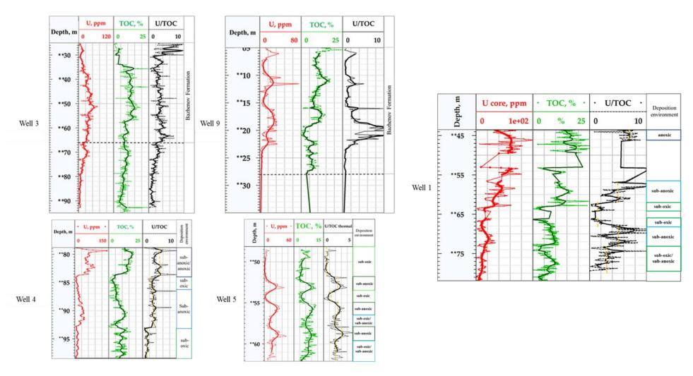
Figure 47. Logviews BF: U-core (gamma spectrometry); TOC – organic matter profile with 1 mm resolution (TCP); ratio U/TOC; sulphur isotopy  $\delta^{34}$ S; deposition environment: sub-anoxic, anoxic, sub-oxic.
