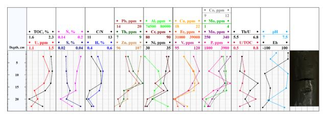
Figure 35. The bottom sediments of station 3. The distributions: H, N, S elements and TOC (analyzer CHN628); U, Pb, Th, Zn, Al, Cr, Ni, Cu, Fe, V, Co, Mo, Mn, P concentrations (ICP-MS); the ratio C/N, U/TOC, and Th/U; also pH and Eh.
