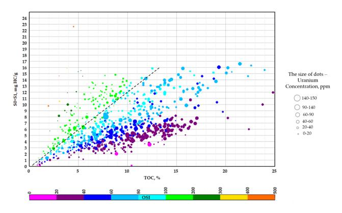
Figure 60.  $S_0+S_1$  - TOC diagram from pyrolysis studies of 11 wells, where color indicates OSI value and dot size reflects uranium concentration. The dotted line separates dots with OSI > 100 from other dots for which OSI < 100 (see color fill).
