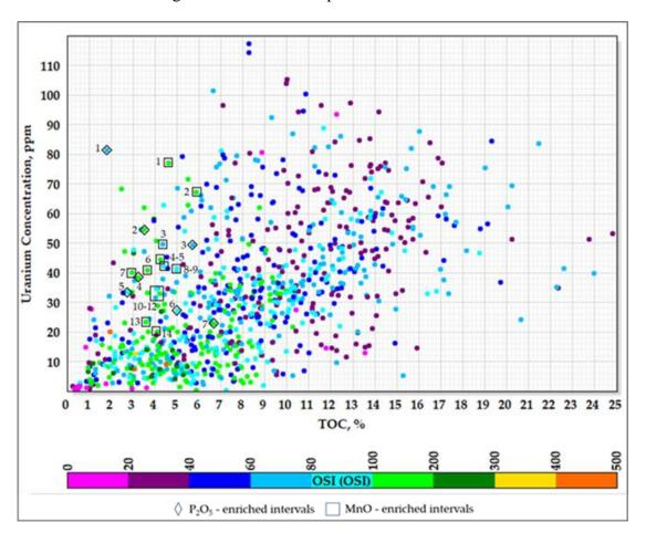
Figure 56. Cross-plot of the uranium concentration and total orgaic carbon (TOC) according to the study of 12 wells penetrating the BF. The color of the dots reflects the oil saturation index (OSI) values.
