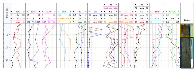
Figure 36. The bottom sediments of station 4. The distributions: H, N, S elements and TOC (analyzer CHN628); U, Th, Cu, Cr, Al, Cd, Zn, V, Fe, Ni, Co, Pb concentrations (ICP-MS); isotopy data:  $\delta^{34}$ S,  $\delta^{13}$ C, and  $\delta^{13}$ C<sub>carb</sub>,  $\delta^{15}$ N; the ratios C/N, U/TOC, and Th/U; also pH.
