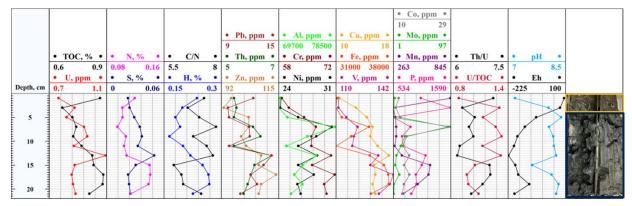
Figure 38. The bottom sediments of station 6. The distributions: H, N, S elements and TOC (analyzer CHN628); U, Pb, Th, Zn, Al, Cr, Ni, Cu, Fe, V, Co, Mo, Mn, P concentrations (ICP-MS); the ratio C/N; also pH and Eh.
