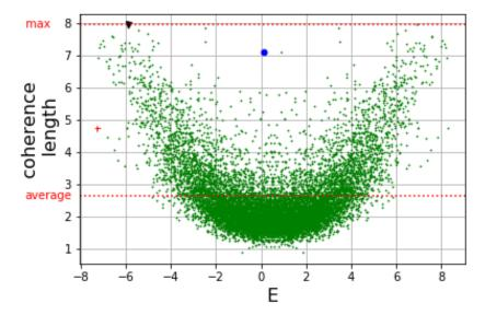
Figure 4-1: The coherence length for eigenstates of the nonintegrable Hamiltonian (4.2) with J=1, J'=0.2, U=1, N=6, L=12,  $\delta H=0$ . The ground state, the state with the maximal coherence length and a state in the middle of the spectrum with a large coherence length are marked with the red cross, black triangle and blue circle, respectively. Fig. from ref [2]
