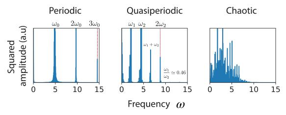
Figure 2-7: Fourier spectrum of the observable  $S_1^z(t)$  for different regimes of motion.
