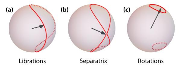
Figure 2-2: Periodic solutions corresponding to the one-body Hamiltonian (2.7) (a) J = 0.79 Librations, trajectory oscillates between two poles (b)  $J \simeq J^* = 1.15041$  Vicinity of the separatrix distinguishing between two regimes (c) J = 1.76 Rotations, trajectory is confined inside the upper hemisphere. There is an identical trajectory inside the bottom hemisphere obtained from  $\mathbf{S}_p(0) = (0, 0, -1)$ .
