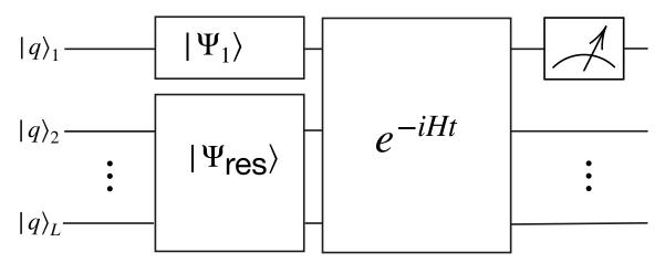
Figure 3-10: Scheme for implementing the delayed disclosure of a secret: a classical bit is encoded into a local observable  $S_1^z = \pm 1/2$ . The rest of the system (a reservoir) is prepared in a state  $|\Psi_{\rm res}\rangle$  constructed to generate a revival at time  $\tau$ . The bit is retrieved when the measurement time t is equal to  $\tau$ . Measurements at times t outside of a narrow interval around  $\tau$  would lead to random outcomes.
