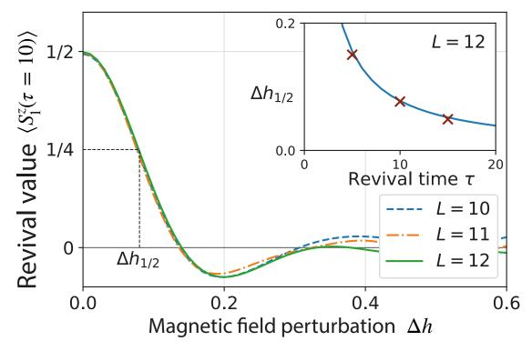
Figure 3-8: Dependence of revival value  $\langle S_1^z(\tau=10)\rangle$  on the magnetic field perturbation  $\Delta h$ . Revival time is fixed at  $\tau=10$ , perturbation is introduced as  $(h_x, h_y) = (2.2 - \Delta h, 2.2 - \Delta h)$ . The inset shows the dependence of resolution  $\Delta h_{1/2}$  on the revival time  $\tau$ . Solid line corresponds to the fit  $\Delta h_{1/2} = c_0/\tau$ , where  $c_0 = 0.3895$ .
