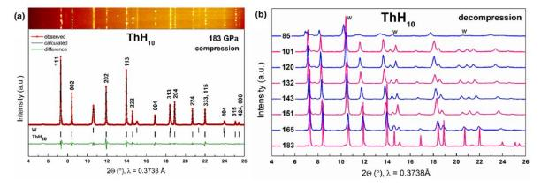
**Figure 13.** (a) Le Bail refinement of  $Fm \, \bar{3} \, m$ -ThH<sub>10</sub> and bcc-W at 183 GPa. The experimental data, fit, and residues are shown in red, black, and green, respectively. (b) Experimental XRD patterns of  $Fm \, \bar{3} \, m$ -ThH<sub>10</sub> in the pressure range of 183–85 GPa.
