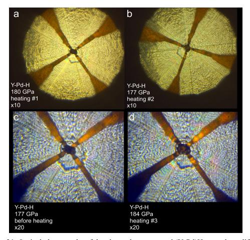
**Figure 21**. Optical photographs of the electrode system and  $(Y_3Pd)H_x$  sample at different stages of the laser heating. Gasket consists of  $CaF_2/epoxy$ .
