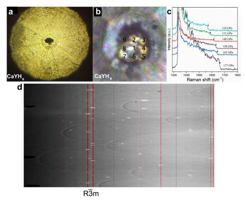
**Figure 55.** Optical photography of diamond anvils of (a) DAC MgY at 175 GPa and (b) DAC CaY at 177 GPa. Numbers indicate the area of the X-ray diffraction analysis of the CaYH<sub>x</sub> sample. (c) Raman spectra of the DAC CaY recorded during decompression. Arrows indicate the frequency points that were used to calculate the pressure. (d) Typical diffraction pattern ("cake") of a CaYH<sub>x</sub> sample at 177 GPa. Red lines correspond to the XRD pattern of CaYH<sub>10</sub>.
