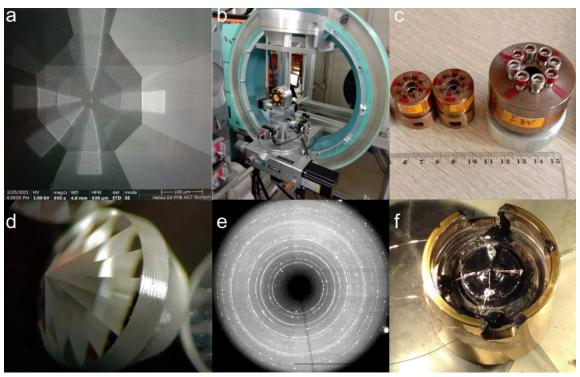
**Figure 4**. Elements of high-pressure diamond chambers and the experiment technique. (a) System of five platinum electrodes applied by a focused ion beam to the surface of a diamond anvil. (b) High-pressure chamber mounted on a goniometer for synchrotron imaging (Kurchatov synchrotron radiation source). (c) High-pressure bronze chambers of
