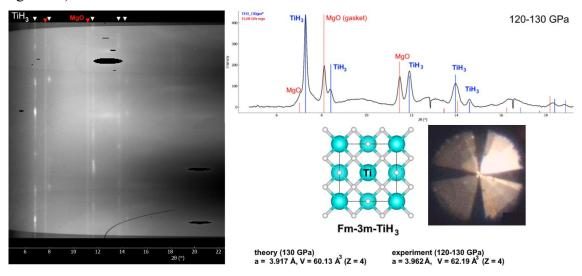
**Figure 63.** X-ray diffraction pattern of a titanium hydride sample obtained by heating the  $TiH_2/H_2$  target at 120-130 GPa. MgO was used as a gasket. The obtained data indicate the formation of the previously predicted  $Fm\overline{3}m$ -TiH<sub>3</sub> [298], the sample of which does not exhibit superconducting properties. This experiment was carried out jointly with Dr. M. Kuzovnikov.
