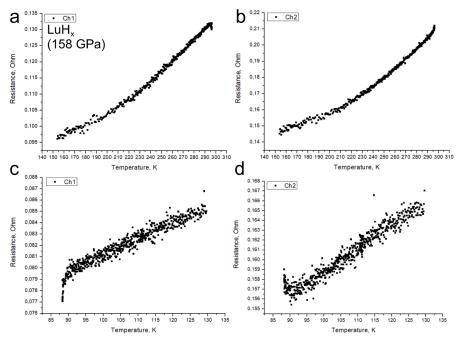
**Figure 44.** Temperature dependence of the electrical resistivity of the LuH<sub>x</sub> sample synthesized at 158-161 GPa for 2 channels (ch1, ch2, cooling). In the interval from 155 to 130 K, there is a gap in the data because of an error of a recording device. A possible superconducting transition begins around 90 K.
