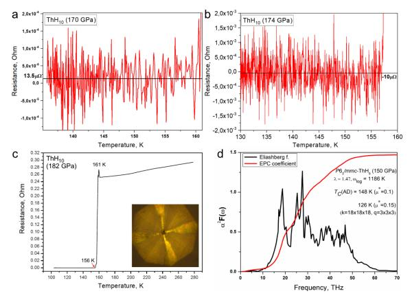
**Figure 17.** Superconducting properties of thorium polyhydrides. (a, b) Residual resistance of ThH<sub>10</sub> in the superconducting state at 170–174 GPa. (c) Superconducting transition width  $\Delta T_C = 5$  K for ThH<sub>10</sub> at 161 K. Inset: thorium polyhydride sample lying on a diamond anvil with electrodes placed on it. The culet size is 50  $\mu$ m. (d) Refined Eliashberg function of P63/mmc-ThH<sub>9</sub> calculated at 150 GPa.
