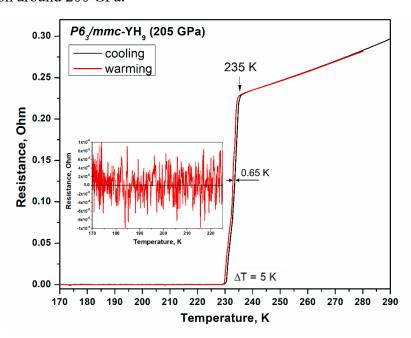
**Figure 35.** Temperature dependence of the electrical resistance of YH<sub>9</sub> at 205 GPa in the cooling and heating cycles. The hysteresis does not exceed 0.65 K. Inset: residual resistance in the superconducting state, not exceeding  $16 \mu\Omega$ .
