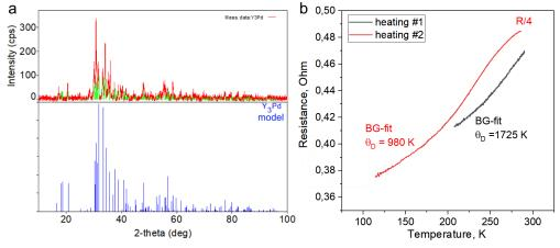
**Figure 22.** (a) X-ray diffraction pattern (wavelength:  $CuK_a$ ) of an initial Y<sub>3</sub>Pd intermetallic prepared by arc melting (K. Pervakov, LPI) and used for loading a high-pressure diamond anvil cell. (b) Temperature dependence of the electrical resistance of the sample (Y<sub>3</sub>Pd) $H_x$  after the first and second laser heating.
