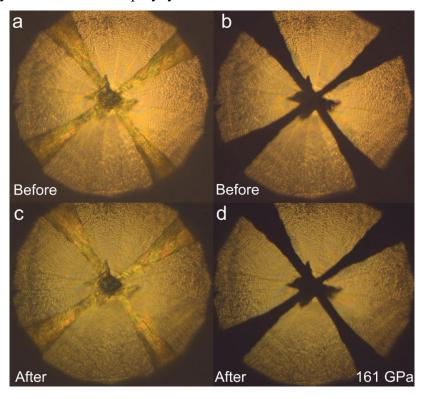
**Figure 43**. Photos of the Lu/AB sample (a, b) before and (c, d) after the laser heating at 161 GPa. Gasket consists of CaF<sub>2</sub>/epoxy.
