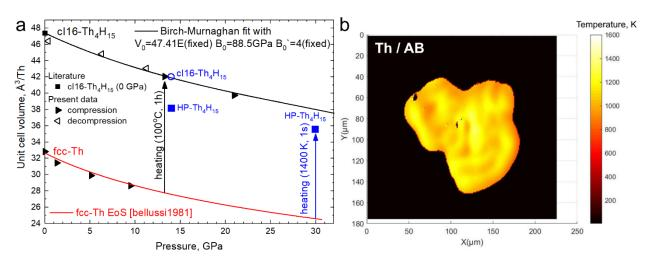
**Figure 7.** Equations of state of lower thorium hydrides. The data marked by black symbols were obtained by Dr. M. Kuzovnikov [186]; those marked in blue were obtained in this work when heating the sample at a higher temperature and pressure. (b) Heat map of a laser-heated thorium sample in an ammonia borane medium, obtained using an acousto-optical filter in the laboratory of Prof. P. Zinin (STC UI RAS, Moscow) [189, 190].
