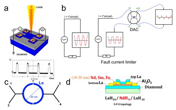
**Figure 72**. Possible applications of superhydrides as (a) single-photon detectors; (b) current limiters and nonlinear electronic elements; (c) SQUID magnetometers and magnetic field sensors; (d) gates controlled by magnetic field in SFS contacts.
