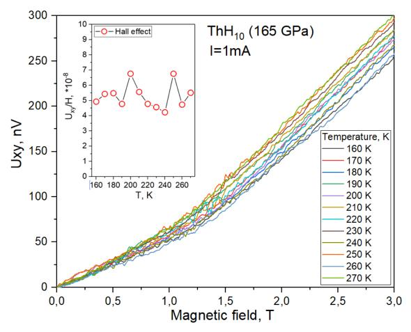
**Figure 19.** Hall effect in  $ThH_{10}$ . Dependence of the Hall voltage ( $U_{xy}$ , nV) on the applied magnetic field at different temperatures from 160 to 270 K. Inset: temperature dependence of the Hall voltage divided by the value of the external magnetic field for the linear part of the diagram (H > 1.2 T).
