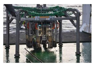
Figure 19. A sampling of bottom sediments by multi-corer sediment.
