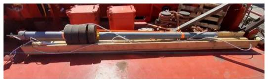
Figure 18. A sampling of bottom sediments by a gravitational steel pipe.
