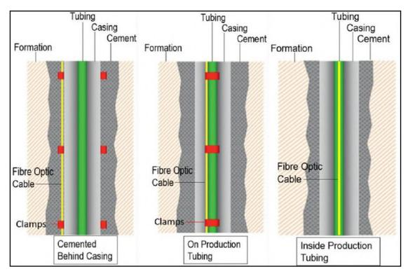
Figure 2-4: Fibre optic cable coupling options in a borehole survey. Modified from Fenta et al. [2021]
