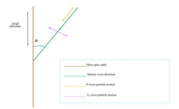
Figure 4-23: Directional sensitivity of DAS to body waves. DAS is most sensitive to the component of particle motion that is in the axial direction. Source: [Wamriew et al., 2021b].
