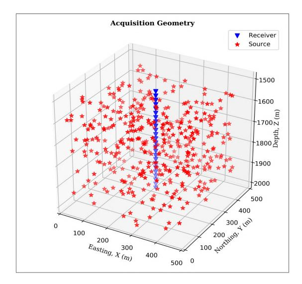
Figure 4-4: Acquisition geometry comprising of 24 3-C receivers in a downhole array (blue triangles) at intervals of 20 m, and 200 microseismic events (red stars) randomly distributed within the cube of sides 500m. The events had varying moment magnitudes in the range  $-2.0 \leq \mathbf{M_w} \leq 0.$ Source: [Wamriew et al., 2022a]
