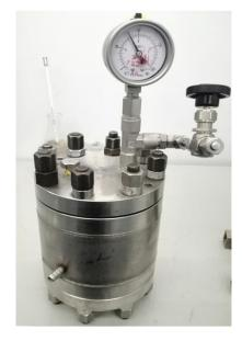
Figure 16. Equipment (pressure cell) for artificial formation of hydrate in sediment samples.
