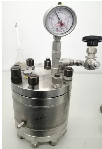
Figure 16. Equipment (pressure cell) for saturation of sediment by hydrate.
