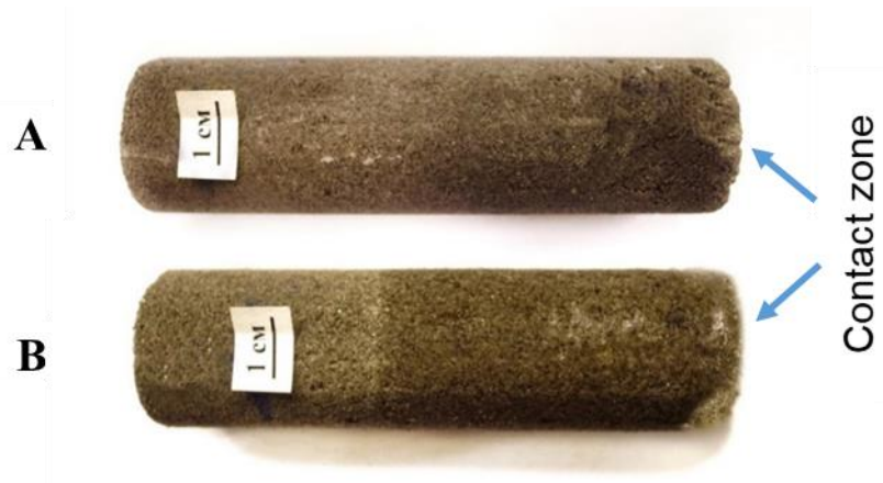
Figure 29. The appearance of frozen sand samples (fine sand 4, W=12%) before (A) and after interaction (B) with 0.1 NaCl solution at -6^{\circ}\text{C} .
