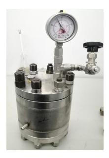
Figure 16. Equipment (pressure cell) for artificial formation of hydrate in sediment samples.
