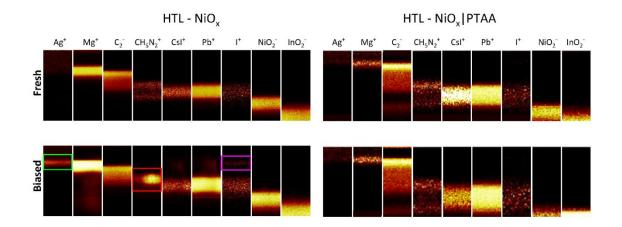
Figure 24. ToF-SIMS ions profiles for fresh and biased (2000 h) samples of solar cells with NiO<sub>x</sub> and NiO<sub>x</sub>|PTAA as HTLs.
