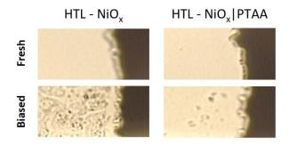
Figure 26. Optical microscope images of the top silver electrode edges before and after biasing for 2000 h.
