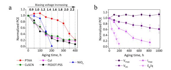
Figure 22. Evolution of normalized PCE during the "stepwise" biasing of solar cells with various HTLs (a). Evolution of the efficiency of PSCs with PTAA as HTL under applied electric bias ( $V_{mpp} = 0.7 \text{ V}$ ,  $V_{OC} = 1 \text{ V}$ ,  $I_{mpp} = 18.3 \text{ mA/cm}^2$ ,  $E_g/q = 1.55 \text{ V}$ ) (b).
