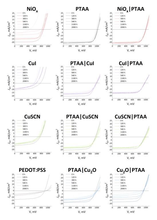
Figure A4. The typical examples of the device J-V curves evolution under 1 V external
