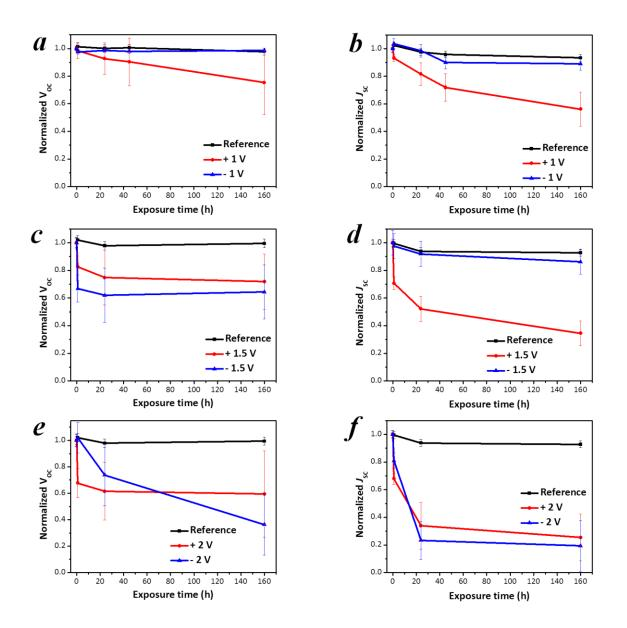
Figure A1. Evolution of the solar cell open circuit voltage ( $V_{OC}$ ; a, c, e) and short circuit current density ( $J_{SC}$ ; b, d, f) as functions of the electric bias exposure time at the applied potentials of 1 V (a-b), 1.5 V (c-d) and 2 V (e-f) in forward and reverse directions.
