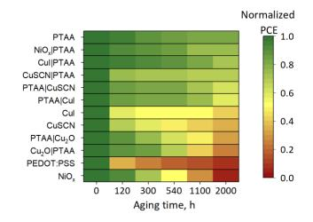
Figure 23. Evolution of normalized average efficiency for solar cells with various HTLs under constant 1V electric bias. HTLs are ranged from the best (top) to worst (bottom).
