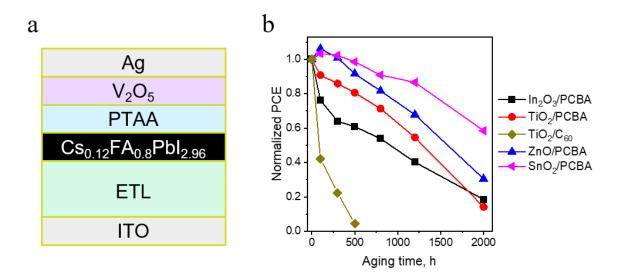
Figure 27. Schematic structure of solar cells used in experiment (a). Evolution of normalized average PCE of solar cells with various ETLs (b).
