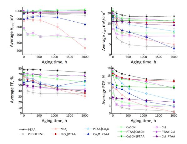
Figure A3. Evolution of the solar cell average open circuit voltage ( $V_{OC}$ ), short circuit current density ( $J_{SC}$ ) fill factor (FF) and power conversion efficiency (PCE) as functions of the electric bias exposure time at the applied potential of 1 V in forward direction.
