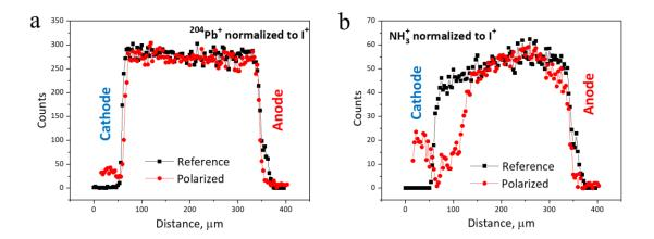
Figure 10. ToF-SIMS profiles of lateral two-terminal devices across the channel formed by MAPbI<sub>3</sub> semiconductor film before (reference) and after (biased) exposure to electric bias of 1 V/µm for 340 h. A ratio of ion yields is given to account for possible geometry effects: <sup>204</sup>Pb<sup>+</sup> normalized to I<sup>+</sup> (a) and NH<sub>3</sub><sup>+</sup> normalized to I<sup>+</sup> (b).
