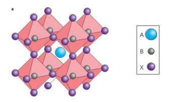
Figure 1. Perovskite structure with orthorhombic symmetry.<sup>26</sup>
