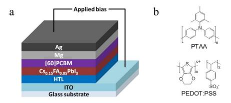
Figure 21. Schematic structure of solar cells used in experiments (a). Chemical structures of organic HTMs (b).
