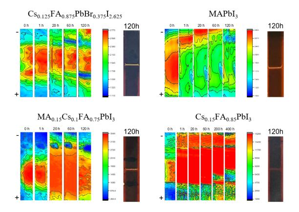
Figure 17. PL mapping of different perovskite materials and optical photos of corresponding channels.
