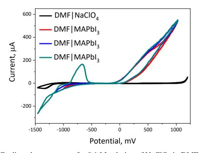
Figure 14. Cyclic voltammograms for 0.1 M solution of NaClO<sub>4</sub> in DMF as illustration of the DMF electrochemical stability window and 0.01 M solution of MAPbI<sub>3</sub> in DMF measured with different cathodic potential cutoffs.
