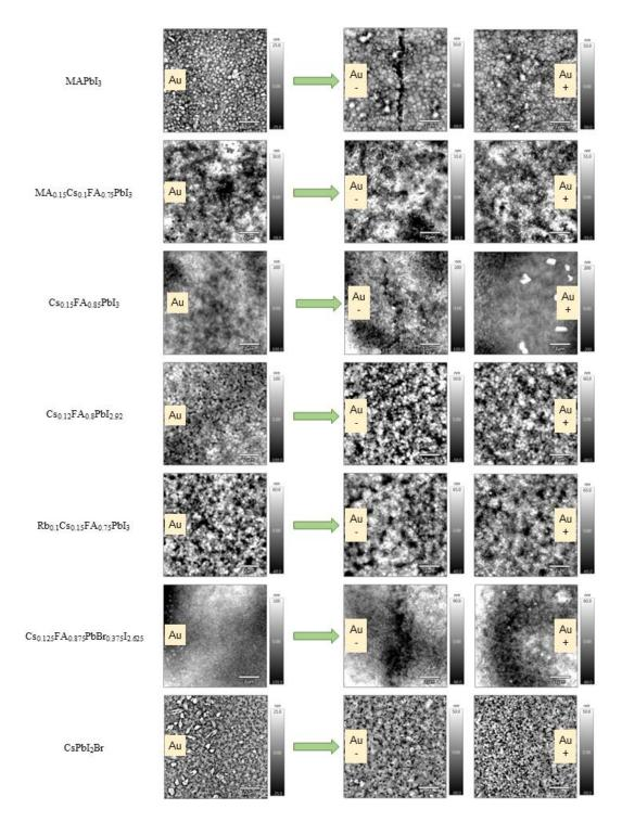
Figure 19. AFM data for different perovskite materials before and after biasing for 80
