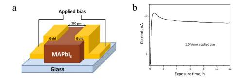
Figure 8. General layout of the lateral two-electrode device (a). Evolution of the current flowing through the channel of the lateral two-terminal device under potentiostatic polarization with 1 V/µm applied bias (b).
