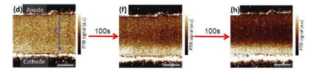
Figure 7. IR-microscopy for CH<sub>3</sub><sup>+</sup> migration monitoring under applied electric field in the publication of Y. Yuan et al.<sup>[56]</sup>
