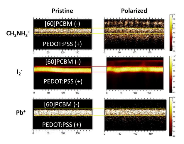
Figure 13. ToF-SIMS chemical maps showing the distribution of the characteristic marker ions Pb<sup>+</sup>, I<sub>2</sub><sup>-</sup> and CH<sub>3</sub>NH<sub>3</sub><sup>+</sup> in the reference cells and devices exposed to 2 V under forward bias for 160 h.
