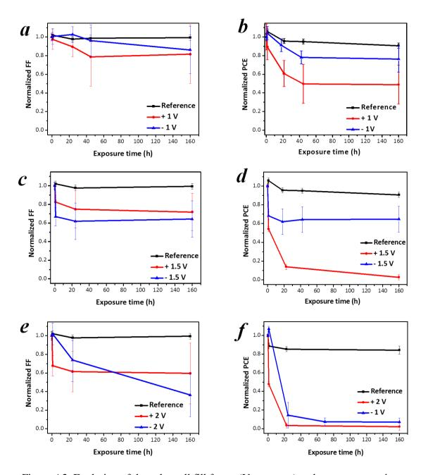
Figure A2. Evolution of the solar cell fill factor ( $V_{OC}$ ; a, c, e) and power conversion efficiency (*PCE*; b, d, f) as functions of the electric bias exposure time at the applied potentials of 1 V (a-b), 1.5 V (c-d) and 2 V (e-f) in forward and reverse directions.
