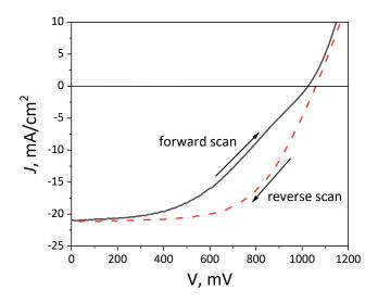
Figure 3. Typical *J*-V curve for perovskite solar cell with hysteresis effect between forward and reverse scan.
