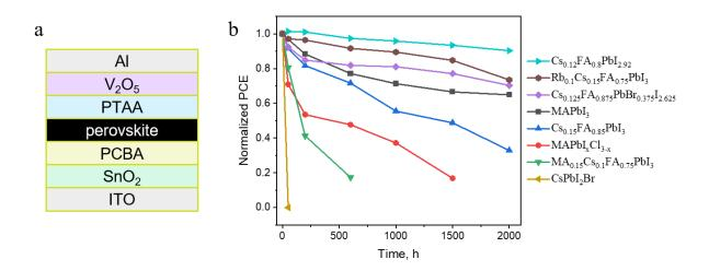
Figure 20. N-i-p solar cells device configuration (a). Normalized average PCE evolution for the batches of solar cells with different perovskite photoactive lyers.
