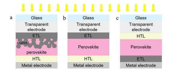
Figure 2. Mesoporous (a) and planar (b,c) perovskite solar cell configuration, including conventional n-i-p (b) and inverted p-i-n(c).
