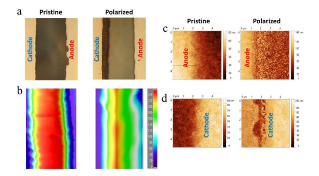
Figure 9. Optical microphotograph of the device channel before (left) and after (right) applying 1 V/μm bias for 340 h (a). PL mapping of the channel before (left) and after (right) applying 1 V/μm bias for 24h. (b) AFM for anode (c) and cathode (d) areas before (left) and after (right) applying 1 V/μm bias for 100 h.
