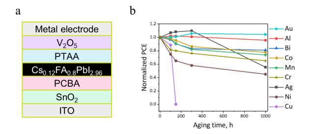
Figure 28. Evolution of normalized average PCE of solar cells with various electrodes.
