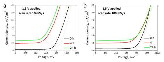
Figure 12. Evolution of forward (solid lines) and reverse (dot lines) *J*-V curves at scan rates of 10 mV/s (a) and 100 mV/s (b) for device biased at the applied potential of 1.5 V in forward direction.
