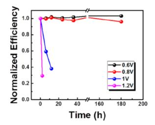
Figure 6. PCE drop depending on the external electric field demonstrated by S. Bae et al.<sup>49</sup>
