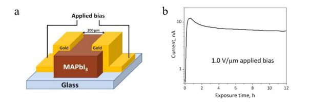
Figure 8. General layout of the lateral two-electrode device (a). Evolution of the current flowing through the channel of the lateral two-terminal device under potentiostatic polarization with 1 V/ $\mu$ m applied bias (b).
