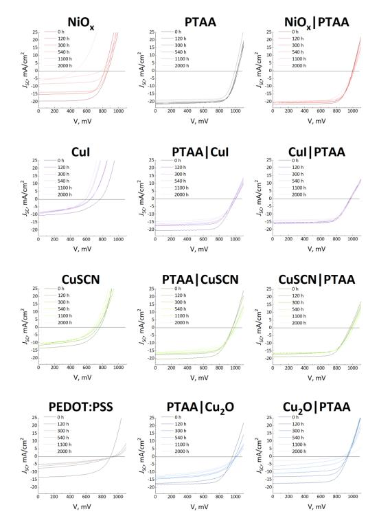
Figure A6. The typical examples of the device *J*-V curves evolution under 1 V external bias voltage applied in forward direction.
