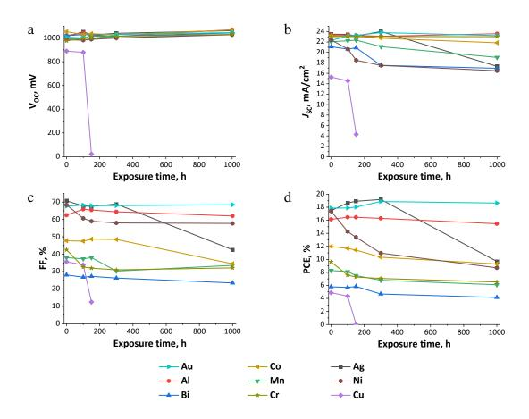
Figure A8. Evolution of the absolute values for solar cell average open circuit voltage  $V_{OC}$  (a), short circuit current density  $J_{SC}$  (b), fill factor FF (c) and power conversion efficiency PCE (d) as functions of the electric bias exposure time at the applied potential of 1 V in forward direction, depending on the used top electrode metal.
