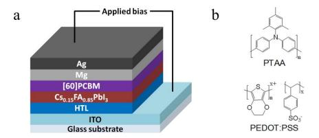
Figure 21. Schematic structure of solar cells used in experiments (a). Chemical structures of organic HTMs (b).
