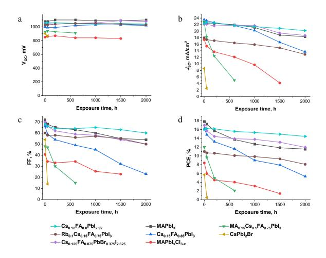
Figure A4. Evolution of the absolute values for solar cell average open circuit voltage  $V_{OC}$  (a), short circuit current density  $J_{SC}$  (b), fill factor FF (c) and power conversion efficiency PCE (d) as functions of the electric bias exposure time at the applied potential of 1 V in forward direction, depending on the used perovskite material.
