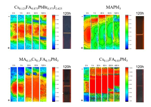
Figure 17. Evolution of PL signal in the channel of lateral two-electrode device during the electric bias exposure for various perovskite materials. Optical photos of corresponding channels for every material after the 120 h biasing are presented on the left. Channels on all figures oriented horizontally, with cathode on top position and anode in bottom position.
