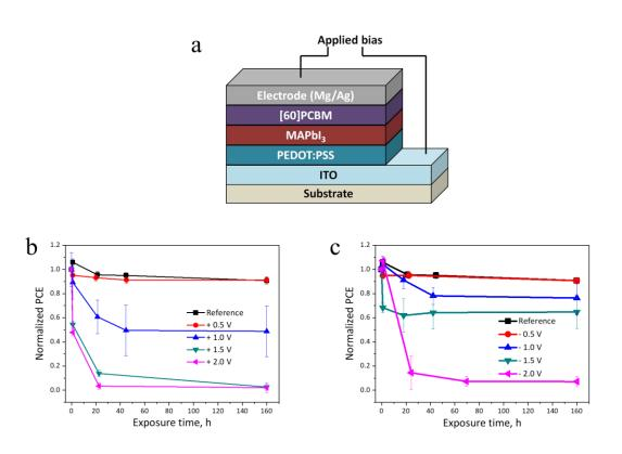
Figure 11. Schematic layout of the p-i-n perovskite solar cell architecture (a). The evolution of the device performance under different external biases applied in forward direction (b) and the comparison of the device degradation kinetics under forward and reverse bias of 1.5 V (c).
