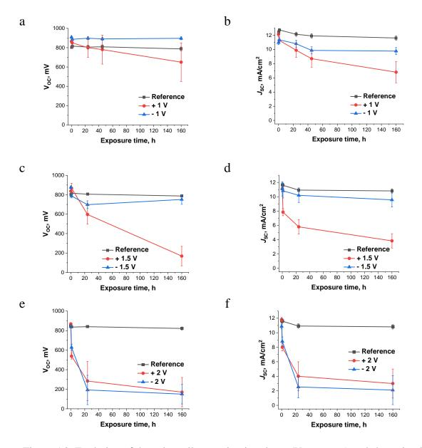
Figure A2. Evolution of the solar cell open circuit voltage ( $V_{OC}$ ; a, c, e) and short circuit current density ( $J_{SC}$ ; b, d, f) as functions of the electric bias exposure time at the applied potentials of 1 V (a-b), 1.5 V (c-d) and 2 V (e-f) in forward and reverse directions.
