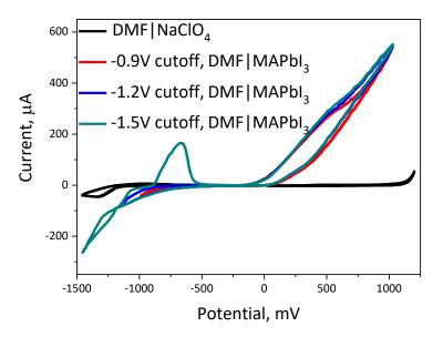
Figure 14. Cyclic voltammograms for 0.1 M solution of NaClO<sub>4</sub> in DMF as illustration of the DMF electrochemical stability window (from -1200 mV to 1100 mV) and 0.01 M solution of MAPbI<sub>3</sub> in DMF measured with various cathodic potential cutoffs.
