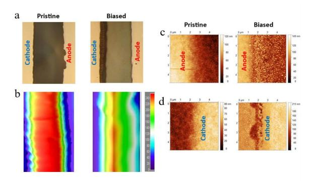
Figure 9. Optical microphotograph of the device channel before (left) and after (right) applying 1 V/μm bias for 340 h (a). PL mapping of the channel before (left) and after (right) applying 1 V/μm bias for 24 h (b). AFM for anode (c) and cathode (d) areas before (left) and after (right) applying 1 V/μm bias for 100 h.
