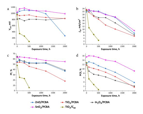
Figure A7. Evolution of the absolute values for solar cell average open circuit voltage  $V_{OC}$  (a), short circuit current density  $J_{SC}$  (b), fill factor FF (c) and power conversion efficiency PCE (d) as functions of the electric bias exposure time at the applied potential of 1 V in forward direction, depending on the used ETL.
