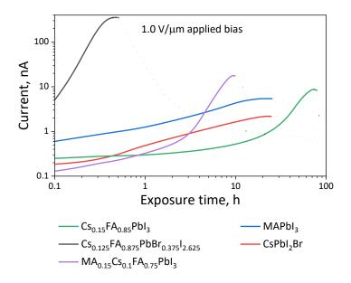
Figure 16. Evolution of the current flowing through the channel of the lateral two-terminal device under potentiostatic polarization with 1  $V/\mu m$  applied bias for various perovskite materials.
