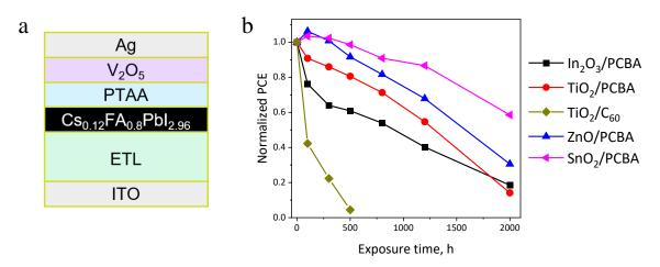
Figure 27. Schematic structure of solar cells used in the experiment of ETL variation (a). Evolution of normalized average PCE of solar cells with various ETLs (b).
