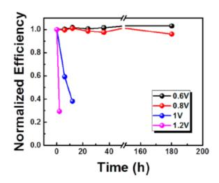
Figure 6. PCE drop depending on the external electric field demonstrated by S. Bae et al. Reproduced with permission from ref.<sup>49</sup> Copyright 2016, ACS Publications.
