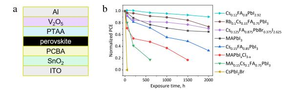
Figure 20. N-i-p solar cells device configuration (a). Normalized average PCE evolution for the batches of solar cells with different perovskite photoactive layers (b).
