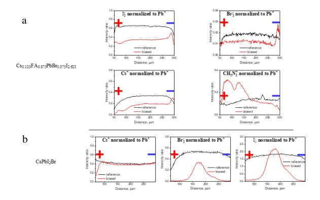
Figure 18-2. ToF-SIMS profiles of lateral two-terminal devices for across the channel formed by corresponding (noted on the left) perovskite semiconductor film Cs<sub>0.125</sub>FA<sub>0.875</sub>PbBr<sub>0.375</sub>I<sub>2.625</sub> (a) CsPbI<sub>2</sub>Br (b) before (reference) and after (biased) exposure to electric bias of 1 V/μm for 300 h. A ratio of ion yields is given to account for possible geometry effects.
