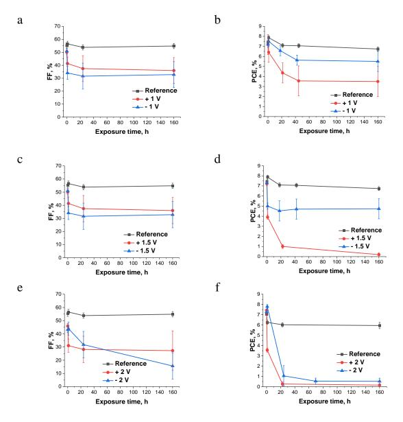
Figure A3. Evolution of the solar cell fill factor (FF; a, c, e) and power conversion efficiency (PCE; b, d, f) as functions of the electric bias exposure time at the applied potentials of 1 V (a-b), 1.5 V (c-d) and 2 V (e-f) in forward and reverse directions.
