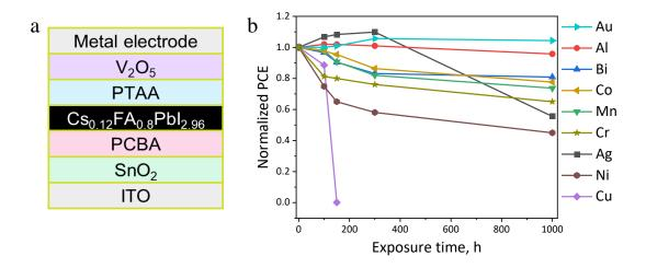
Figure 28. Schematic structure of solar cells used in the experiment of top electrode variation (a). Evolution of normalized average PCE of solar cells with various electrode materials (b).
