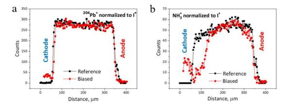
Figure 10. ToF-SIMS profiles of lateral two-terminal devices across the channel formed by MAPbI<sub>3</sub> semiconductor film before (reference) and after (biased) exposure to electric bias of 1 V/μm for 340 h. A ratio of ion yields is given to account for possible geometry effects: <sup>204</sup>Pb<sup>+</sup> normalized to I<sup>+</sup> (a) and NH<sub>3</sub><sup>+</sup> normalized to I<sup>+</sup> (b).
