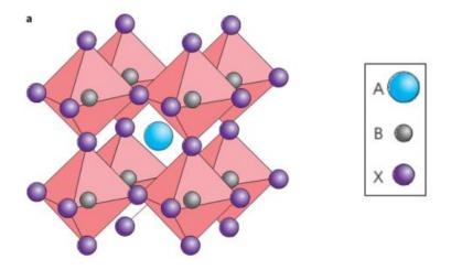
Figure 1. A typical crystal structure of a perovskite. Reproduced with permission from ref.<sup>25</sup> Copyright 2018, Springer Nature.
