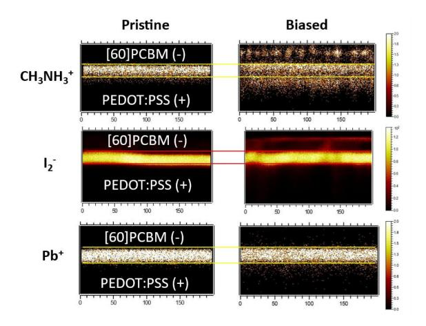
Figure 13. ToF-SIMS chemical maps showing the distribution of the characteristic marker ions  $Pb^+$ ,  $I_2^-$  and  $CH_3NH_3^+$  in the reference cells and devices exposed to 2 V under forward bias for 160 h.
