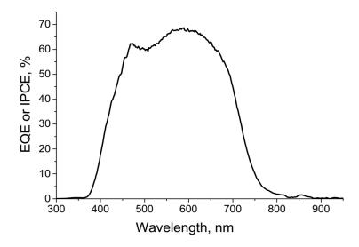
Figure 5. Typical EQE curve
