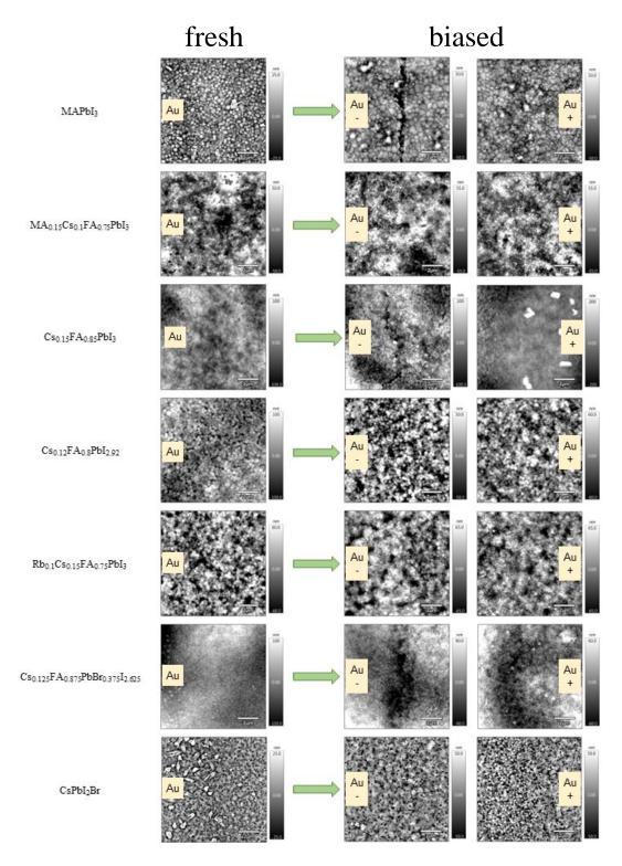
Figure 19. AFM data for corresponding (marked on the left) perovskite materials before and after biasing for 80 hours near both electrodes.
