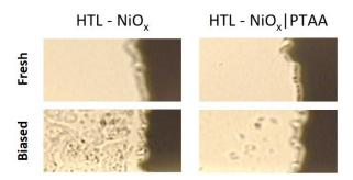
Figure 26. Optical microscope images of the top silver electrode edges before and after biasing for 2000 h.
