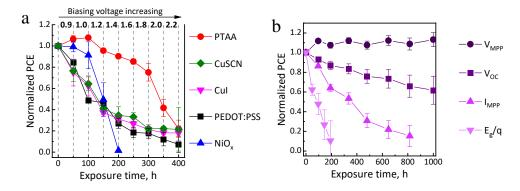
Figure 22. Evolution of normalized PCE during the "stepwise" biasing of solar cells with various HTLs (a). Evolution of the efficiency of PSCs with PTAA as HTL under applied electric bias ( $V_{MPP} = 0.7 \text{ V}$ ,  $V_{OC} = 1 \text{ V}$ ,  $I_{MPP} = 18.3 \text{ mA/cm}^2$ ,  $E_g/q = 1.55 \text{ V}$ ) (b).
