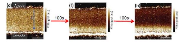
Figure 7. IR-microscopy for CH<sub>3</sub><sup>+</sup> migration monitoring under applied electric field in the publication of Y. Yuan et al. Reproduced with permission from ref.<sup>55</sup> Copyright 2015, John Wiley & Sons.
