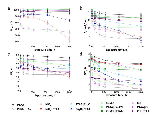
Figure A5. Evolution of the absolute values for solar cell average open circuit voltage  $V_{OC}$  (a), short circuit current density  $J_{SC}$  (b), fill factor FF (c) and power conversion efficiency PCE (d) as functions of the electric bias exposure time at the applied potential of 1 V in forward direction, depending on the used HTL.
