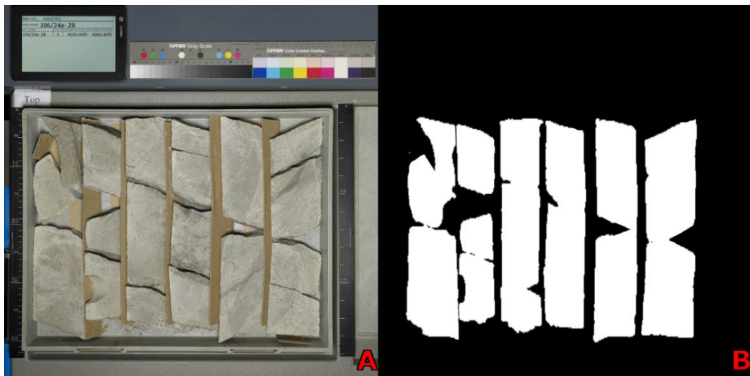
Figure 41. Examples of the labelled datasets for core column extraction. A – the original image; B – the produced mask. Up to 10 minutes required to produce such labels.
