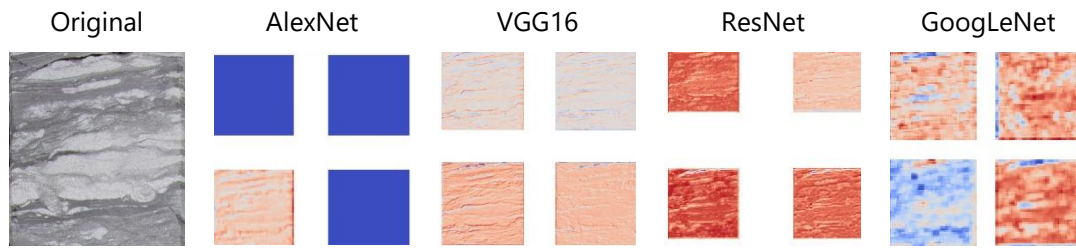
Figure 28. An image and extracted features from a random layer of different CNNs. The extracted features show various patterns extracted by the CNN. It may include structure (AlexNet, VGG, ResNet), texture and general patterns (GoogLeNet).
