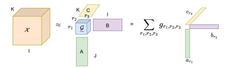
Figure 2-3: The scheme of Tucker decomposition in a case of 3-d tensor. The source of the image: Cichocki et al. [2016].
