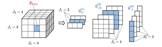
Figure 2-4: The example of computation tensor elements via it's TT representation. Source of the image: [Xu et al., 2022].
