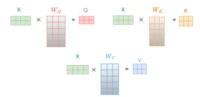
Figure 2-7: Visualization of Query, Key and Value claculation inside the transformer block.
