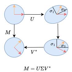
Figure 2-1: The interpretation of SVD. The operator of transformation  $\mathbf{M}$  is decomposed into rotation  $\mathbf{U}$ , scaling  $\boldsymbol{\Sigma}$  and rotation back  $\mathbf{V}^{\mathbf{T}}$ .
