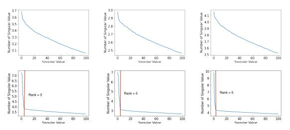
Figure 6-5: First row: singular values for the 1-st module layer, "**uncompressible**", in ColBERT. Gradual slope of spectrum is less sharp. Second row: singular values for the 4-th module layer,"**compressible**", in ColBERT. Gradual slope of spectrum is more sharp.
