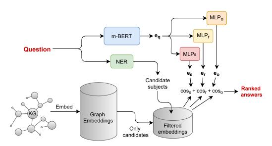
Figure 3-6: Text2Graph method used in our experiments: 1-Hop QA pipeline. First, we take an original entity and relation embeddings. The question is embedded using m-BERT. This embedding is then processed by MLP, yielding candidate representations of an object, relation, and subject. The sum of the subject, relation, and object cosines is the final score of the triple candidates.
