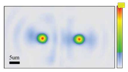
Figure 5-11: Real-space normalised intensity distribution of two coupled elliptical and horizontally elongated condensates.
