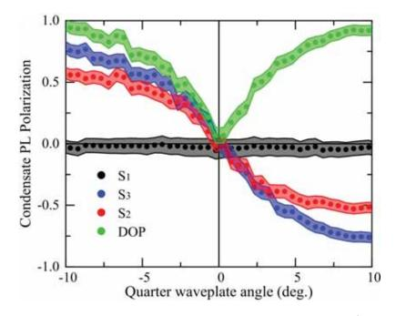
Figure 4-8:  $S_1$ ,  $S_2$ ,  $S_3$  and DOP for the small pump ellipticity (QWP angle) at  $P = 1.23P_{\text{th}}$ . Figure is adopted from [1].
