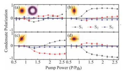
Figure 5-2: (a) Power dependence of the condensate  $S_{1,2,3}$  Stokes parameters (black, red, blue markers) for the annular pump with resultant cylindrically symmetric condensate profile (see right and left insets, respectively). (b) Same, but now for a trap/condensate with a major axis orientated at 90°, (c) 45°, and (d) 0°. Insets in (a)-(d) depict the real-space condensate PL with black line showing the orientation of the trap major axis. Adopted from [2]
