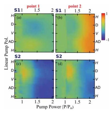
Figure 4-7: (a,b)  $S_1$  and (c,d)  $S_2$  polarisation maps for two different sample positions for varying linear polarisation and power of the excitation laser. H, D, V and AD correspond to horizontal, diagonal, vertical, anti-diagonal polarisation, respectively. The figure is adopted from [1].
