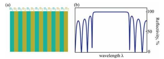
Figure 2-1: (a) The schematic of the Distributed Bragg Reflector (DBR) built of the alternating layers of two semiconductor materials with different refractive indices  $n_1$  and  $n_2$ . (b) The typical reflectivity spectrum of the DBR at a normal incidence.
