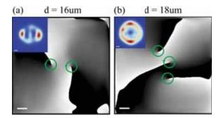
Figure 7-13: (a) The phase profile of the condensate in the rotating trap with 16  $\mu$ m diameter d at f = 3 GHz demonstrating two co-rotating vortices in the condensate. (b) The phase profile of the condensate in the rotating trap with 17.5  $\mu$ m diameter d at f = 3 GHz demonstrating 3 vortices. The insets in (a) and (b) represent the real-space condensate intensity distribution.
