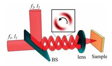
Figure 3-5: Experimental setup for the rotating excitation pattern generation. Two single-mode, frequency stabilised lasers (with frequencies  $f_1$ ,  $f_2$ , and OAMs  $l_1$ ,  $l_2$  respectively) are overlapped on the beamsplitter(BS). The resulting dumbbell-shaped beating pattern rotates with the frequency and direction defined by two lasers.
