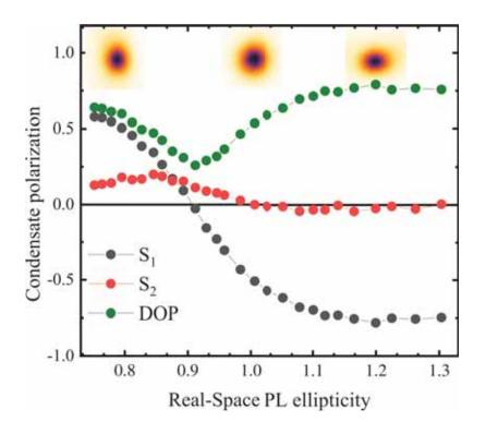
Figure 5-10:  $S_1$ ,  $S_2$  and DOP of the condensate PL as a function of the spatial ellipticity (the ratio between the major and minor axes of the condensate real-space intensity distribution).
