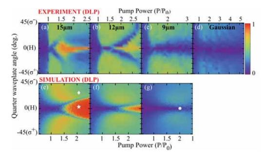
Figure 4-12: DLP polarisation maps as a function of pump power and QWP angle. Panels (a-c) show results for decreasing pump diameter  $d = 15, 12, 9 \ \mu\text{m}$ . Panel (d) shows the condensate DLP in the case of a Gaussian spot excitation (no confinement). (e-f) Simulated time-average condensate DLP using Eqs. ((4.2)-(4.4)). The star, circle and diamond markers correspond to panels (a-c) in Figure 4-15. Figure is adopted from [1].
