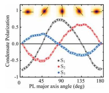
Figure 5-7: The date for the elliptical trap rotation without the correction on the optical retardance of the experimental setup. Figure demonstrates the condensate Stokes components  $S_1$  (black),  $S_2$ (red) and  $S_3$  (blue) as a function of the orientation of the elliptical condensate (x- axis and yellow-to-black insets). The image is adopted from [2].
