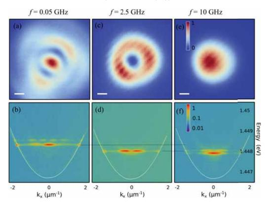
Figure 7-7: Time-integrated condensate intensity profiles (a,c,e) and dispersion (b,d,f), when externally stirred at f = 0.05, 2.5 and 10 GHz respectively. The white dashed lines in panels (b-f) depict the lower polariton branch dispersion. The black dashed line is to guide the eye and compare the energy of the condensate at different rotations.
