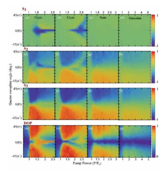
Figure 4-13:  $S_1$  (a-c),  $S_2$  (e-h),  $S_3$  (i-l), and DOP (m-p) for a ring excitation geometry of diameter  $d = 15, 12, 9 \ \mu \text{m}$  and a Gaussian excitation geometry of FWHM = 4  $\mu \text{m}$ respectively. The figure is adopted from [1].
