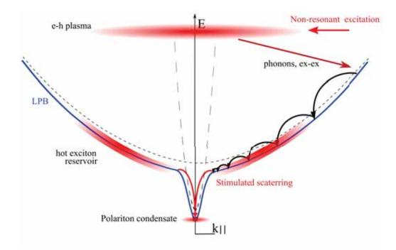
Figure 2-4: Mechanism of polariton condensation under non-resonant excitation.
