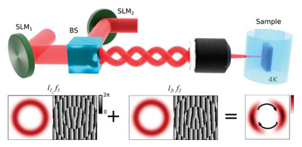
Figure 7-3: The excitation part of the experimental setup. The beating of two modified with the SLMs and frequency-detuned lasers forms the rotating in-time laser pattern utilised as the confining and stirring potential for polaritons. The red-scaled images show the excitation lasers' profiles, and the grayscaled images are SLM masks for corresponding pattern generation. The figure is adopted from [3]
