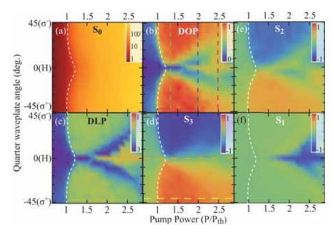
Figure 4-4: (a) Total emission intensity  $S_0$  in arbitrary units, (b) DOP, (c) DLP, (d)  $S_3$ , (e)  $S_2$  and (f)  $S_1$  as a function of pump power P and ellipticity (QWP angle) for a ring excitation geometry with a diameter of  $d = 12 \ \mu m$ . QWP angles  $\pm 45^{\circ}$  and 0° correspond to right-, left-circular, and linear polarised excitation. White dashed lines depict the condensation threshold. Figures are adapted from [1].
