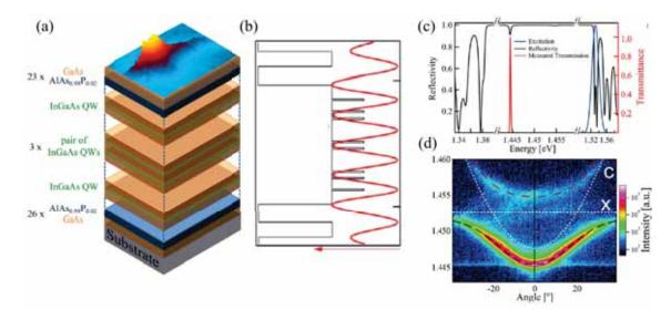
Figure 3-6: The microcavity sample used for experiments. (a) The layered semiconductor structure of the microcavity sample. (b) The refractive index distribution (x-axis) along the cross-section of the microcavity (y-axis). The red line depicts the electric field distribution. (c) The sample's reflectivity (black) and transmittance (red) spectrum. (d) The dispersion of the polariton PL. The image is adapted from ref. [56]
