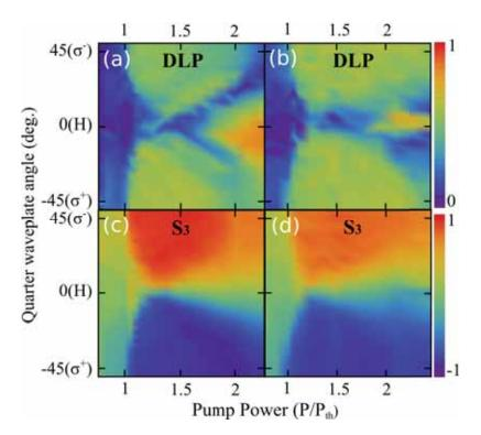
Figure 4-10: Measured DLP (a,b) and  $S_3$  (c,d) for the exciton-photon detuning of  $\Delta = -4$  meV (a,c) and  $\Delta = -2$  meV (b,d). The figure is adopted from [1].
