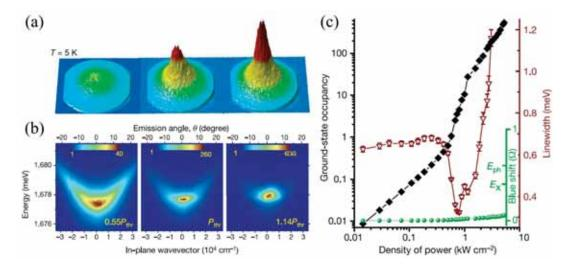
Figure 2-5: Polariton condensation under non-resonant excitation. The narrowing of the distribution and intensity increase in real-space (a) and on the dispersion (b). (c) The power-driven condensation is visible in the nonlinear growth of polariton number, the narrowing of linewidth and energy blueshift. Adapted from Ref. [17]
