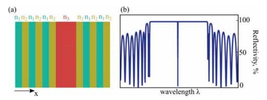
Figure 2-2: (a) The schematic of the microcavity built of DBRs. (b) The typical reflectivity spectrum of the microcavity.
