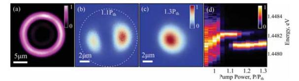
Figure 7-5: (a) Experimental pump profile of one of the excitation lasers. The condensate PL in the stationary optical trap (a) with 14  $\mu$ m diameter at a pump power of (b) 1.1Pth and (c) 1.3Pth. (d) Corresponding energy resolved power dependence of the condensate PL, showing an eventual departure from the excited state into the trap ground state. The white dashed line in (b) schematically depicts the annulus of the laser pump profile.
