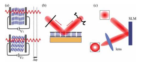
Figure 3-2: (a) The schematic of the pixel of the spatial light modulator under different applied voltage  $V_1$  and  $V_2$ . Alternated with voltage refractive index result into the phase shift  $\Delta \phi = \phi(V_1) - \phi(V_2)$  of the transmitted light. (b) The schematic of the change of the wavefront of the incident light by the SLM screen with black lines depicting the phase fronts. (c) Reflective SLM and transformation of the Gaussian beam into the ring-shaped one.
