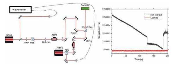
Figure 6-3: Left panel: experimental setup for the realisation of the rotating optical pattern with the beating note of two single-mode lasers (MBR1 and MBR2). The frequency of both lasers is externally stabilised with the wavemeter and PID loop. Right panel: the track of the laser frequency (in THz) on time (in seconds) when externally stabilised (red line) and not (black line).
