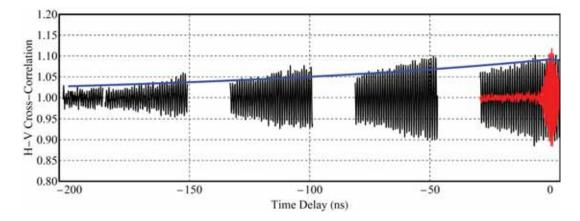
Figure 6-9: The H-V cross-correlation  $g_{H,V}^{(2)}$  for the condensate in the rotating optical trap (black curve) and static annular optical trap (red curve). The blank spaces in the black graph appear due to the incremental addition of the optical delay and limited measurement window. The solid blue line is the fit of the experimental data envelope with  $Ae^{-t/\tau}$ . Figure is adopted from Ref. [4].
