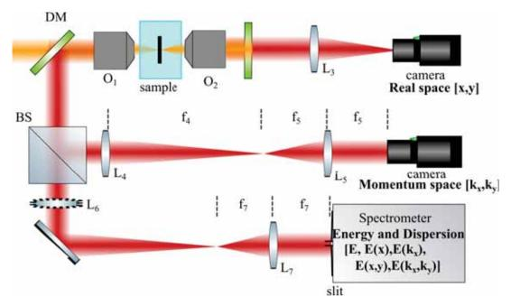
Figure 3-7: Detection part of the experimental setup. The real-space of the polariton emission is recorded in the transmission geometry. The sets of conjugated lenses transfer the k-space distribution both to the CCD camera and the slit of the imaging spectrometer (for dispersion imaging) in the reflection from the sample. The residual excitation laser light is filtered out by the long-pass filter in the transmission and by the dichroic mirror in the reflection.
