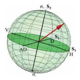
Figure 3-11: Poincare sphere for the representation of polarisation states. The red arrow depicts the polarisation vector. H, V, D, AD  $\sigma_+$  and  $\sigma_-$  stand for the horizon-tal, vertical, diagonal, anti-diagonal right- and left-circular polarisation, respectively.
