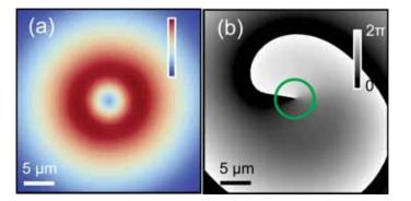
Figure 7-10: Simulated time integrated real-space intensity (a) and instantaneous phase (b) of the condensate at f = 2 GHz demonstrating the formation of the quantised vortex after 800 ps of numerical integration. The figure is adopted from [3].
