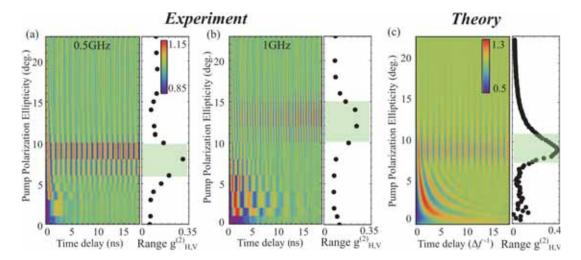
Figure 6-8: Measured H-V cross-correlation maps for (a) f = 0.5 GHz and (b) f = 1 GHz trap rotation as a function of time-delay and pump polarisation ellipticity. (c) Simulated  $g_{H,V}^{(2)}$  of the condensate emission versus the time delay and pump polarisation ellipticity. The black and red point graphs on (a-c) respectively demonstrate the amplitude of the cross-correlation function at 15 ns delay. Figure is adopted from Ref. [4].
