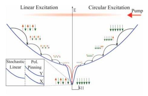
Figure 4-2: Schematic of the lower polariton dispersion (blue curve) illustrating the formation mechanism of the spinor condensate for circular (right side) and linear (left side) polarised non-resonant excitation (red area). The inset: Birefringence splits the degeneracy between X (horizontal) and Y (vertical) polarised modes of the cavity field, leading to the pinning of the condensate pseudospin into the lower energy mode. The figure is adapted from [1].
