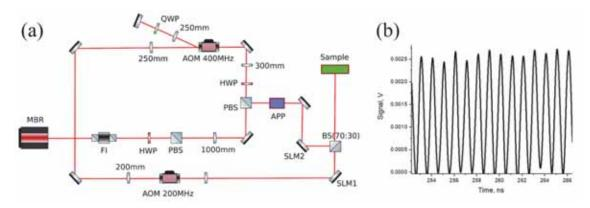
Figure 6-2: (a) Experimental setup for realising the rotating optical pattern with AOMs used for the laser frequency shift. One part of the laser is shifted in a double-path AOM (driving frequency 400 MHz) configuration, the other one with another AOM (driving frequency 200 MHz). Here, we used the anamorphic prism pair (APP) to correct for the beam ellipticity induced by AOM . (b) The beating signal at 1 GHz of two beams frequency-shifted with AOMs.
