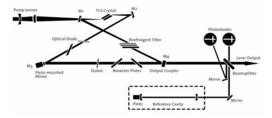
Figure 3-1: The sketch of the MBR-110 Ti:Sapphire laser cavity. The image is taken from the laser manual.
