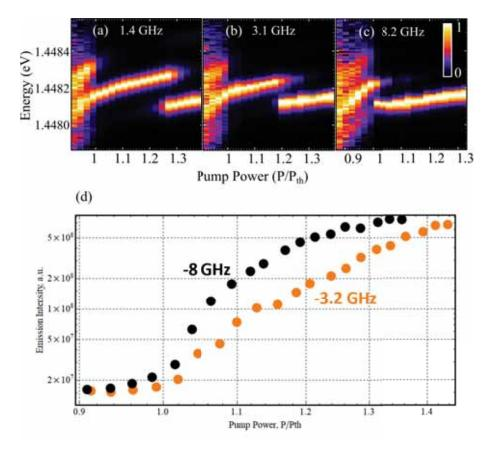
Figure 7-12: Condensate energy spectrum pump power dependence for (a) f = 1.4GHz (b) 3.1 GHz, (c) 8.2 GHz. (d) Intensity power dependence for two values of rotation frequencies demonstrating the different no-linear growth of condensate emission in intensity.
