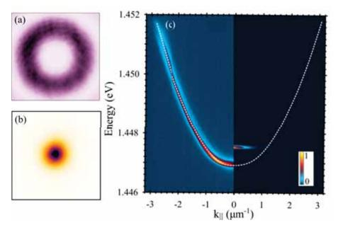
Figure 4-3: (a)The excitation laser profile. (b)The condensate real-space integrated intensity distribution. (c) The normalised polariton dispersion below (left part) and above (right part) the condensation threshold. The white dashed line is to guide the eye.
