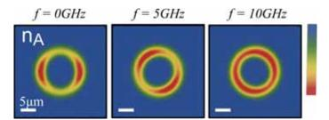
Figure 7-11: The active reservoir distribution snapshots for 0 GHz, 5GHz, and 10 GHz rotation frequency.
