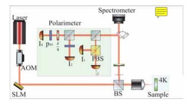
Figure 4-1: The schematic of the experimental setup for study of polariton condensate spin in the optical trap. The condensate is created with the non-resonant laser beam chopped with AOM and shaped with the SLM. The condensate PL is studied in reflection configuration with the polarimeter, real-space camera and spectrometer.
