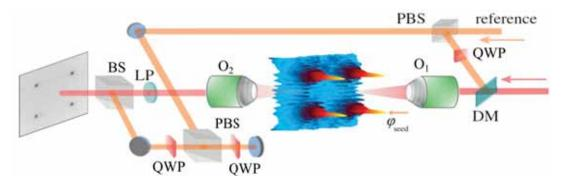
Figure 3-8: Homodyne interferometry setup. The part of the single-mode reference laser is resonantly seeded to the condensate through the dichroic mirror (DM). The other part is greatly expanded and overlapped with the condensate PL (collected with objective  $O_2$ ) on the BS of the Michelson interferometer. The image is adopted from [24] and represents the case of the non-resonant excitation of the condensate with four spots.
