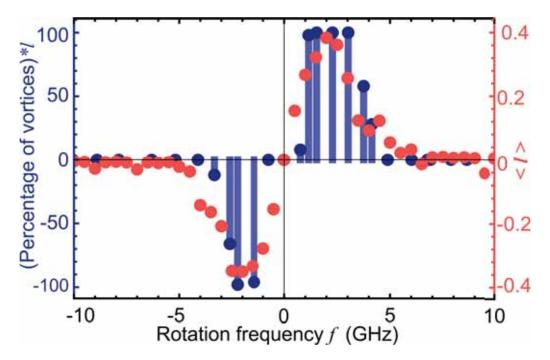
Figure 7-9: Blue points: the number of condensate realisations with vortex out of 100 for each rotation frequency f multiplied by the corresponding topological charge of the vortex  $l = \pm 1$ . Red points: average angular momentum  $\langle l \rangle$  of the condensate over 40 simulation runs. The figure is adopted from [3].
