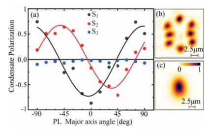
Figure 5-6: (a) Condensate polarisation for different spatial orientations of the 8-Gaussian excitation profile at  $P = 2P_{th}$ . Red and black curves are the sine fit for the experimental data. (b) Excitation laser intensity profile. (c) Condensate PL. Adopted from [2]
