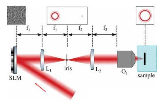
Figure 3-4: The excitation part of the experimental setup: the laser emission is reflected from the SLM and transferred to the excitation objective with the conjugated telescope (lenses  $L_1$  and  $L_2$ ). The iris is used to cut the zeroth diffraction order in the real-space plane. The desired excitation pattern shaped in SLM forms in the focal plane of the objective on the sample held in the cryostat at 4K.
