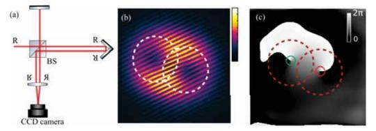
Figure 3-9: The interference of the condensate with the retro-reflected and displaced copy of itself and reconstructed phase - experimental setup (a), the interference pattern (b), the real-space phase distribution (c).
