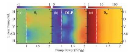
Figure 4-14: Condensate polarisation as a function of pump power and incident linear polarisation angle. (a)  $S_3$ , (b) DLP, (c) and total emitted intensity. The vertical axis denotes the half-waveplate angle and is marked with different linear polarisations. Horizontal (H), vertical (V), diagonal (D), and anti-diagonal (AD). The figure is adopted from [1].
