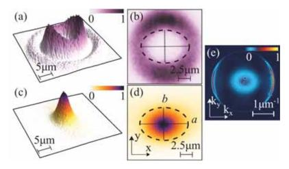
Figure 5-1: Spatial profiles of the (a,b) excitation laser and (c,d) condensate PL. The excitation laser induces a trapping potential with horizontal and vertical radii denoted a, b, respectively. (e) Momentum distribution of the condensate PL. Panels (c,d,e) correspond to a condensate pumped twice above its condensation threshold (i.e.,  $P = 2P_{th}$ ). Adopted from [2]
