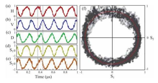
Figure 6-5: Horizontal (a), vertical (b) and diagonal (c) polarisation projections of the condensate emission. The power ratio of excitation lasers is 10%. Time-resolved (d)  $S_1$  and (e)  $S_2$  polarisation components of the condensate emission. (f) The trajectory of the condensate spinor on the equator of the Poincare sphere. The red dashed line is to guide the eye. Figures are adopted from Ref. [4].
