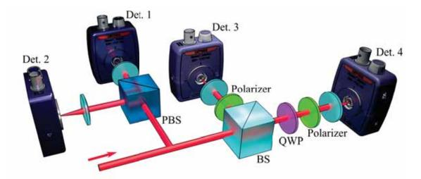
Figure 3-12: The polarimeter optical setup. The intensities of horizontal, vertical, diagonal and circular polarisation projections of the incoming light are measured by Det.1-4, respectively.
