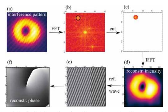
Figure 3-10: 2D FFT is performed on the experimental interference pattern (a), and the resultant image is depicted in (b). The IFFT is performed on the filtered spatial frequency harmonic corresponding to the interference (c). The reconstructed intensity distribution of IFFT intensity is in panel (d). The reconstructed phase corrected on the reference wave (e) is depicted in panel (f).
