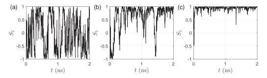
Figure 4-5: Simulated  $S_1$  Stokes component for QWP = 0° showing the onset of pinning with growing pump power. (a)  $P = 1.2P_0$ . (b)  $P = 1.5P_0$ . (c)  $P = 2P_0$ . Figure is adopted from [1].
