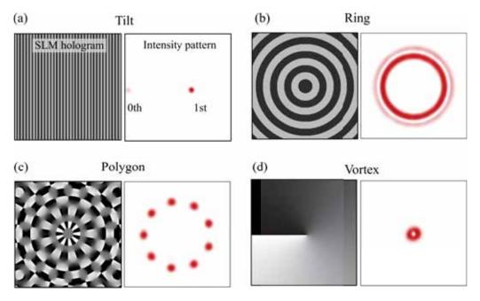
Figure 3-3: The left image in panels (a-d) correspond to the holograms on the SLM for the generation of (a) tilt to separate the reflection from the SLM (zeroth order) and generated laser pattern, ring pattern (b), a polygon of 9 Gaussian spots (c) and optical vortex (d). The right panels in (a-d) represent the corresponding intensity patterns.
