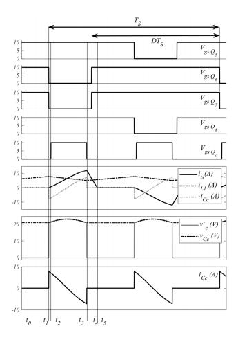
Fig. 26 Bidirectional Full-bridge Boost-mode waveforms.
