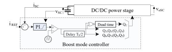
Fig. 25 Proposed SM Boost-mode controller.
