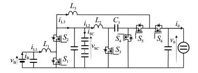
Fig. 12 High-gain dual-input DC/DC converter [48].
