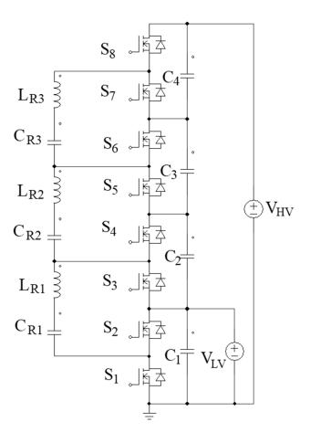
Fig. 17 SiC-based high-gain bidirectional DC/DC multi-level resonant converter.
