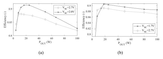
Fig. 47 Efficiency of the MMC for (a) buck and (b) boost-mode.
