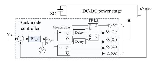
Fig. 23 Proposed SM Buck-mode controller with gating signals.
