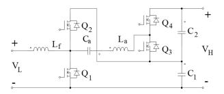
Fig. 10 High-gain soft-switching bidirectional DC/DC converter composed of two half-bridges [46].
