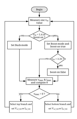
Fig. 32 MMC control diagram for the mode selection.
