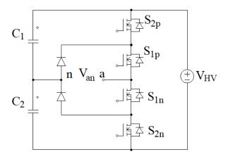
Fig. 53 Diode-clamped 3-level DC/AC multi-level inverter.
