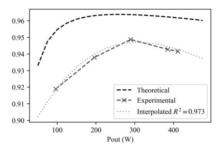
Fig. 49 SM obtained efficiency values vs theoretical curve.
