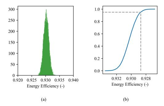
Fig. 50 Probabilistic study based on the extracted SM efficiency from the prototype, (a) histogram and (b) CDF plot.
