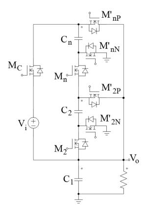
Fig. 15 An n-stage switched-capacitor DC/DC converter schematic.
