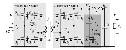
Fig. 22 Bidirectional full-bridge DC/DC converter, presented in [50].
