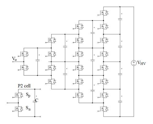
Fig. 54 Generalized multi-level DC/AC inverter with P2 cell.
