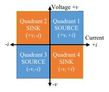
Fig. 51 Four-quadrant plot for bidirectional DC/AC inverters.
