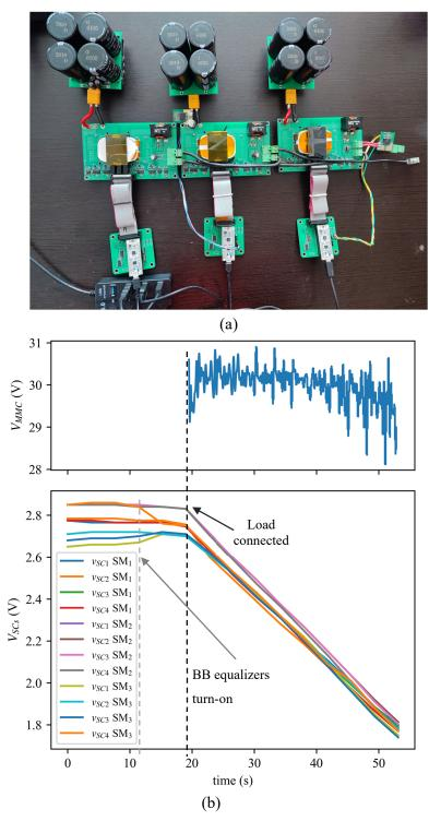
Fig. 48 MMC (a) prototype with Case 3 SMs and (b) discharge process using
