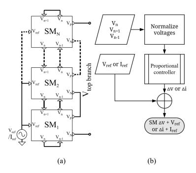
Fig. 29 MMC (a) branch detailed interconnection, and (b) proportional controller of each SM to achieve the self-balancing capability.
