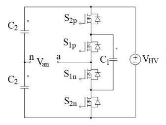
Fig. 52 Capacitor-clamped 3-level DC/AC multi-level inverter.
