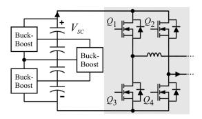
Fig. 35 Internal Buck-Boost balancing system, Case 4 example.
