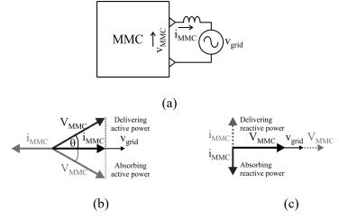
Fig. 30 MMC connected to the grid: (a) basic diagram, (b) phasors when MMC is delivering or absorbing active power, and (c) reactive power.
