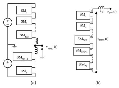
Fig. 21 Block diagram (a) of the traditional and (b) the proposed MMC topology.
