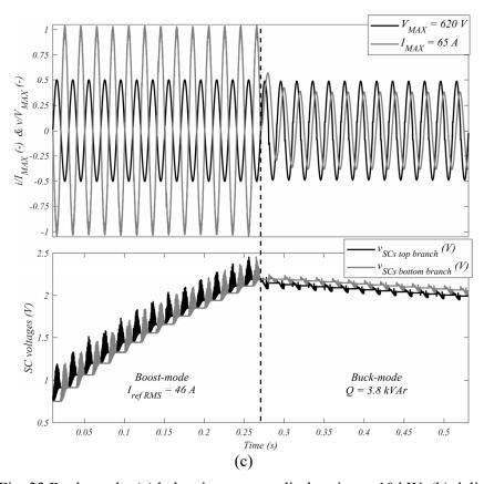
Fig. 33 Buck-mode: (a) balancing process discharging at 10 kW, (b) delivering or absorbing active or reactive power and (c) changing from boost-mode to buck-mode.
