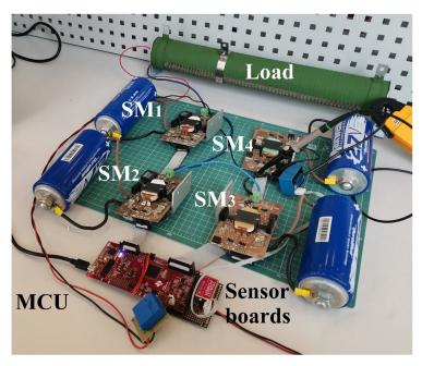
Fig. 43 Complete MMC Prototype.
