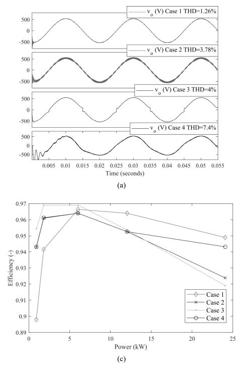
Fig. 19 MMC-based ESS comparison results for (a) Output voltage and calculated THD and (b) Efficiencies.
