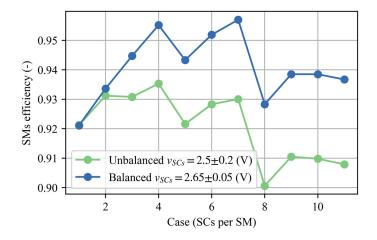
Fig. 39 Minimum SM efficiency with a confidence level of 95% for unbalanced and balanced initial conditions for all Cases.
