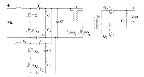
Fig. 9 Wide input range DC/DC converter composed of two cascaded stages [45].
