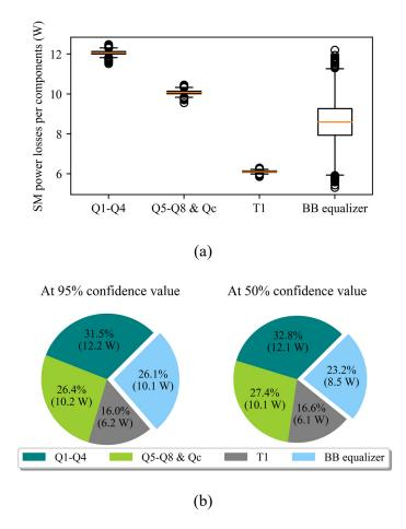
Fig. 42 SM power losses for the main components (a) box plot and (b) pie charts at 95% and 50% confidence levels.
