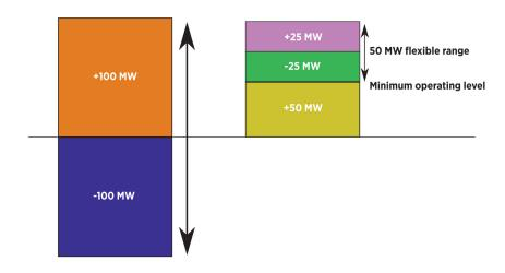
Fig. 3 100MW ESS (left) versus 100MW gas turbine (right) [5].
