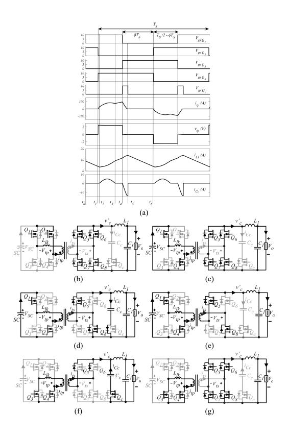
Fig. 24 Bidirectional full-bridge, (a) waveforms, (b) before 1<sup>st</sup> interval, (c) 1<sup>st</sup> interval, (d) 2<sup>nd</sup> interval, (e) 3<sup>rd</sup> interval, (f) 4<sup>th</sup> interval, and (g) 5<sup>th</sup> interval for the Buckmode.
