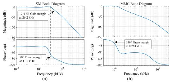
Fig. 28 Closed loop transfer function for: (a) SM using a type-III controller and (b) MMC using a PI controller.
