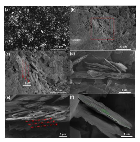
**Figure 6.** SEM of (a) pristine h-BN Powder; (b-f) Self assembled BN: PVA (2:1) composites at different magnifications.
