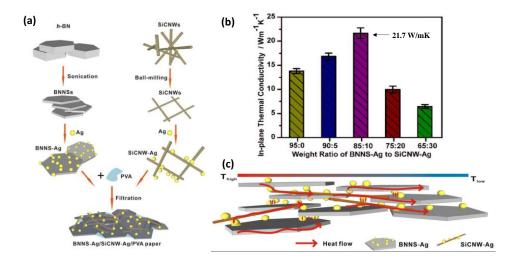
**Figure 10.** (a)Preparation procedure;(b) In-plane thermal conductivity;(c) Proposed mechanism model of thermal conduction in BNNS-Ag/SiCNW-Ag-PVA composite film. (Reprinted with permission from [97] Copyright (2020) American Chemical Society).
