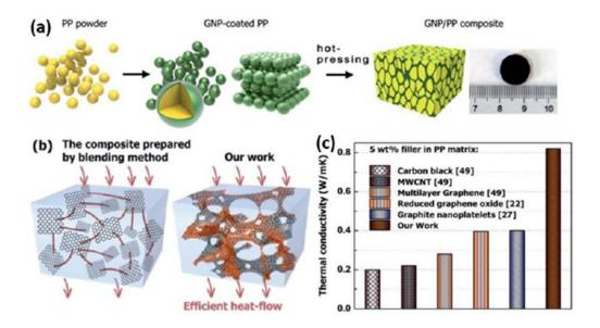
**Figure 7**. Schematics of the fabrication process of GNP/PP framework composites. (a) Fabrication of GNP-coated / PP composites; (b) Diagram comparing effective thermal conduction through a network of connected graphene to that through dispersed graphene; (c) Comparison between the TC values of these composites and randomly dispersed filler composites with the TC of GNP/PP composites (Reprinted with permission from Royal Society of Chemistry, copyright 2017) [64]
