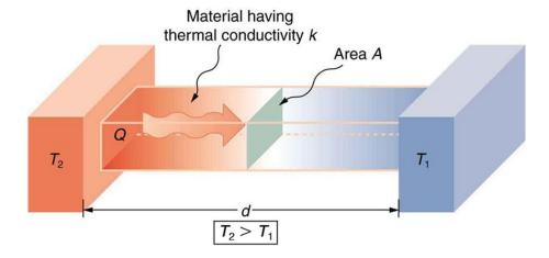
**Figure 1**: Illustration of heat conduction mechanism through any material. (Image Credit: Openstax College Physics)
