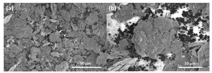
**Figure 7.** SEM image of agglomeration and clustering of BN platelets in BN: PVA (9:1) aerogel-based 3D structure.
