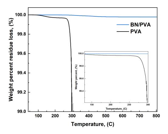
**Figure 11.** TGA curves of PVA and BN/PVA nanocomposites
