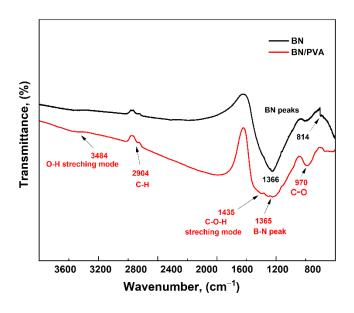
Figure 3. FTIR spectra of PVA aerogel and BN- PVA aerogel.
