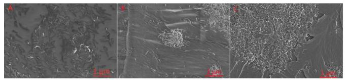
**Figure 2**. SEM imagery of (A) SW, (B) MW2 and (C) MW1. All images are from samples with 2 % wt. CNTs at 65,000X magnification.
