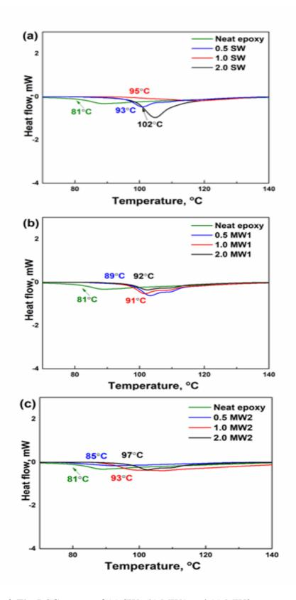
Figure 6. The DSC curves of (a) SW, (b) MW1 and (c) MW2 nanocomposites
