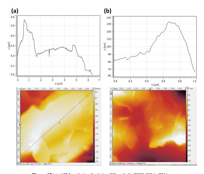
Figure 12(a): AFM analysis of pristine GO and; (b) DEG-GO in PVA.
