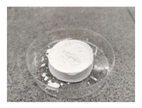
Figure 3. Typical BN/PVA aerogel prototype with the stoichiometric ratio of (2:1) (chapter 3).
