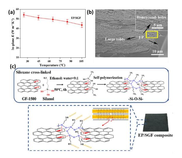
**Figure 9.** (a) Thermal conductivity as a function of temperature for EP/SGF composite at a loading concentration of 20.2 wt.% graphene; (b) Cross-sectional SEM image of EP/SGF. The inset shows EP-filled honeycomb holes [83]; (c) Schematic diagram for synthesizing EP/SCF composites (Reprinted with permission from Springer, copyright 2021).
