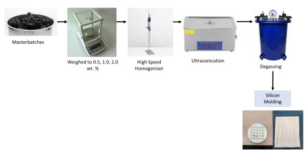
Figure 1. Schematic description of fabrication of CNTs/epoxy composites.
