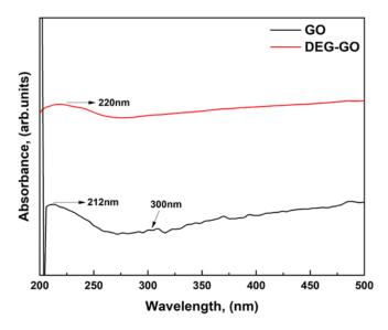
Figure 3. UV-Vis spectra of GO and DEG treated GO.
