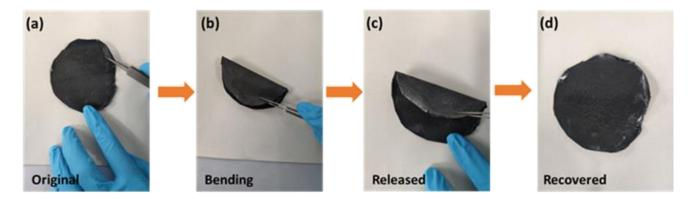
**Figure 9**. Flexibility of thermally conductive DEG-GO/PVA films.
