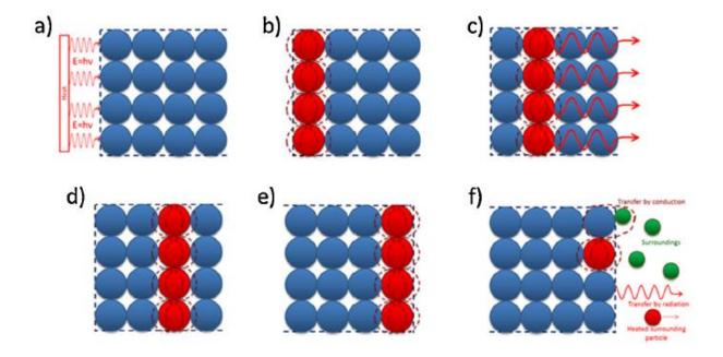
**Figure 2**. Thermal conductivity mechanism in a crystalline material. [32] This simplification of the thermal conductivity mechanism within a perfectly crystalline, ordered, and rigid sample aids in visualizing the phenomenon:
