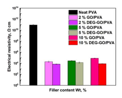
Figure 13. Electrical resistivity of GO/PVA composites
