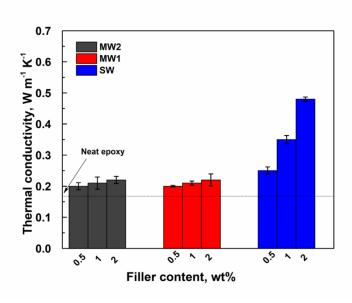
**Figure 4.** Thermal conductivity of epoxy nanocomposites
