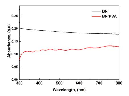
Figure 2. UV-Vis absorption spectra of PVA and BN/PVA (9:1) composite 3D framework (Chapter 3).
