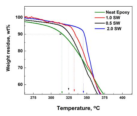
**Figure 5**. Thermogravimetric analysis (TGA) of SW/epoxy composites with various loading contents with thermal stability of specimens at 10 % thermal degradation temperature.
