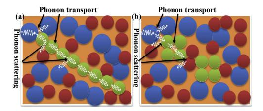
**Figure 5**. (a) Thermal conduction mechanism in the crystalline polymer nanocomposites with a continuous filler network; and (b) thermal conduction mechanism in crystalline polymer nanocomposites with a discontinuous filler network. Here, the crystalline fillers are represented by the green balls whereas, the others represent the polymer atoms [142]. (Reprinted with permission from Elsevier, copyright 2019)
