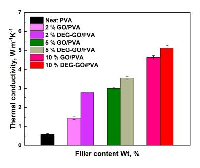
Figure 14. Thermal conductivity of GO/PVA composites.
