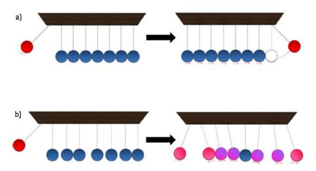
**Figure 4.** Schematic comparison by the Newton pendulum of thermal conductivity in crystalline materials (a) and polymers (b). [32]
