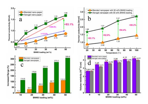
**Figure 8**. Blended nano-paper vs. aerogel nano-paper: (a) thermal conductivities with different BN loading content; (b) thermal conductivities at elevated temperatures with BN loading content of 50wt.%; (c) 3D framework' composite enhancement factor; (d) electrical volume resistivity[69].
