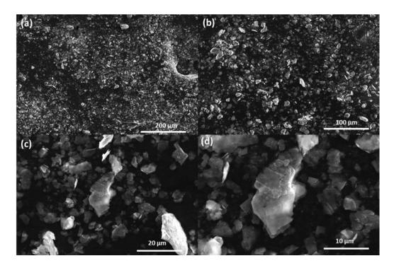
Figure 4. SEM images of pristine BN with an average particle size of  $\sim 10 \mu m$  at different magnifications (chapter 3).
