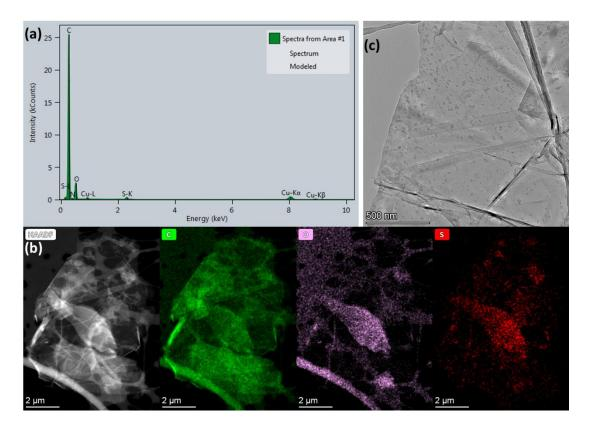
**Figure 5** (a, b): EDS compositional analysis of pristine GO and STEM-EDX elemental mapping images of C, O and S present in GO flakes (c) TEM characterization of GO flakes at high resolution
