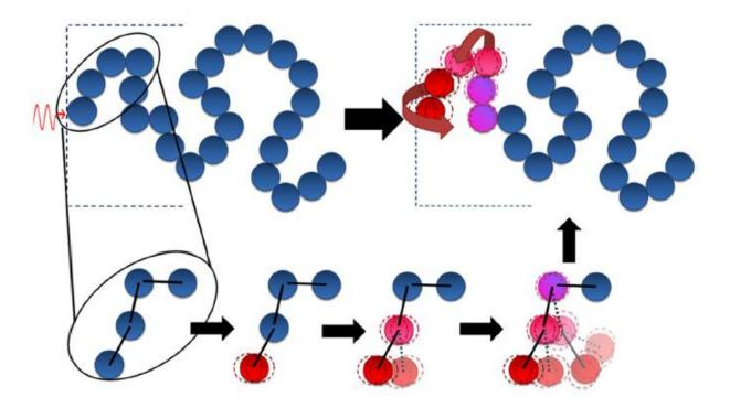
Figure 3. Thermal conductivity mechanism in an amorphous polymer. [32]
