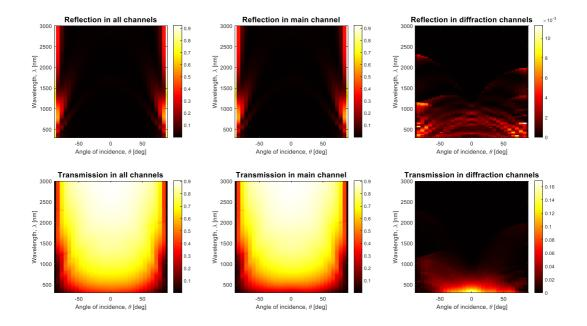
Figure 71. Reflection (upper row) and transmission (bottom row) of diatoms in main, diffraction and all channels. Incidence from the top.
