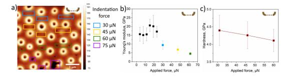
Figure 57. AFM indentation at specific points of a cleaned inner valve. a Inner surface of a frustule measured by the stiff probe after indentation at specific points by applying different indentation force, b Young's modulus calculated using the Derjaguin-Muller-Toropov (DMT) model at different applied forces after averaging over 10 points, c the dependence of hardness on the applied force.
