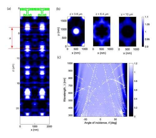
Figure 105. Electric energy distribution inside the diatom frustule calculated for the wavelength  $\lambda$ =450 nm: a) Vertical cross-section, b) Horizontal cross-sections at z=3.8  $\mu$ m, z=6.4  $\mu$ m, z=10  $\mu$ m. c) The dependence of wavelength of incident light on the angle of incidence.
