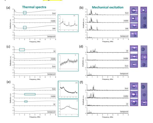
Figure 67. Thermal vibration spectra of diatoms with diameter: (a) 72  $\mu$ m, (c) 60  $\mu$ m, (e) 70  $\mu$ m, with enlarged view of peaks on the right. Externally modulated vibration spectra of the same diatoms. Optical microscopy images of the samples and positions of the laser spot are shown on the right.
