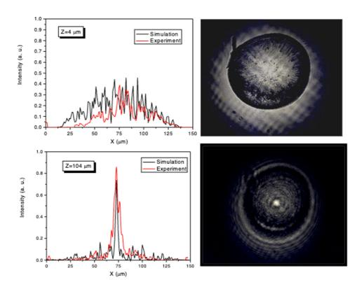
Figure 15. Left: The intensity distribution of the transmitted light at the distance (z) of 4 μm (top) and 104 μm (bottom): the red line is the experimental recorded one, the black line is the numerically estimated. Right: The corresponding images of the diatom surface recorded by a CCD at the two distances considered. Adopted from Ref.<sup>73</sup>. Reproduced with permission from Optica Publishing Group.
