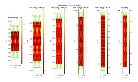
Figure 103. Electric field intensity calculated for P-polarization within vertical cross-sections of samples with height g=5, 10, 15, 20, 25  $\mu$ m in xz plane.
