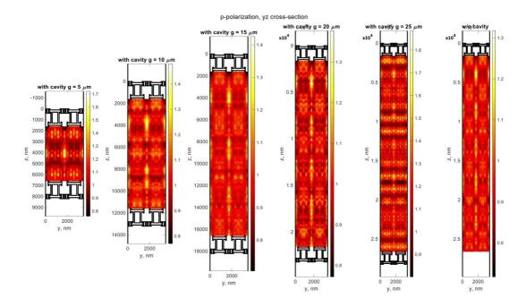
Figure 101. Electric field intensity calculated for P-polarization within vertical cross-sections of samples with height g=5, 10, 15, 20, 25  $\mu m$  in yz plane.
