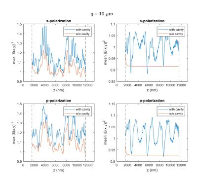
Figure 97. Maximal and mean electric energy distribution calculated for two model structures for distance between valves  $g=10~\mu m$  for S- and P- polarizations.
