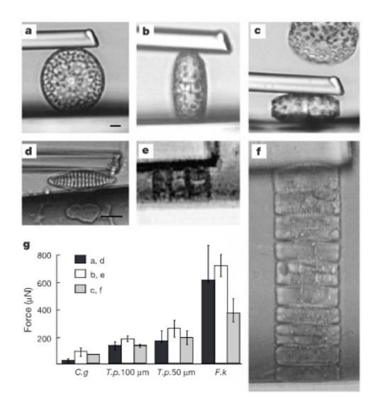
Figure 11. Glass needle tests: Live single cells of *T. punctigera* (a–c) and *F. kerguelensis* (d–f), in chains (e,f). Pressures applied along the girdle bands, (a,d), across the girdle bands (b,e), and across the centre of the valves (c,f). g) Forces necessary to break frustules. Scale bars, 10 μm. Adopted from Ref.<sup>48</sup>. Reproduced with permission from Springer Nature.
