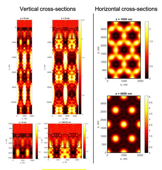
Figure 76. Electric energy density simulation at  $\lambda$ =420 nm,  $\theta$ =0°,  $\phi$ =0° on the surface of the frustule.
