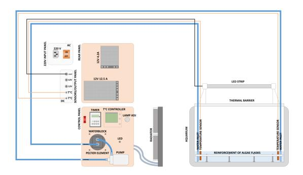
Figure 28. A scheme of the diatom algae incubator
