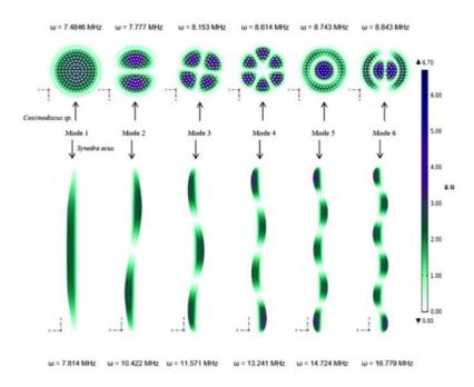
Figure 25. Mode shapes and natural frequencies of *Coscinodiscus* sp. (centric) and *Ulnaria acus* (pennate) observed in the simulation using COMSOL Multiphysics.
