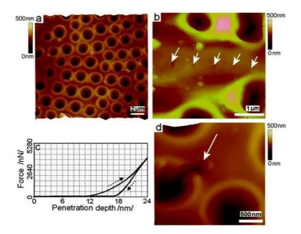
Figure 12. a) Low-resolution AFM image of the internal plate after nanoindentation. b) Series of indentation points (solid arrows) obtained using a force of 1.5-3 μN. c) Typical force penetration curve showing loading and unloading parts (dashed arrows). d) AFM image showing nanoindentation performed on an areola rib at higher applied load (12 μN). White scale bar is 10 μm. Adopted from Ref.<sup>45</sup>. Reproduced with permission from American Chemical Society.
