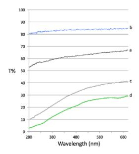
Figure 19. Transmittance spectra for: a - *Coscinodiscus concinnus*, cleaned frustules. b - *C. granii* cleaned frustules. c - *C. concinnus*, dried cells with cell content. d - *C. granii*, dried cells with cell content. Adopted from Ref. <sup>65</sup>. Reproduced with permission from Springer Netherlands.
