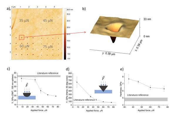
Figure 32. Calibration of a stiff diamond probe (k=400 N/m) on a fused silica reference sample. a) Topography, b) The stiff diamond cantilever, c) The DMT model, d The Hertz model), e) Hardness depending on the applied force. <sup>39</sup>
