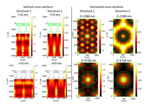
Figure 79. Left: Vertical cross-sections of intensity distribution for structure 1 (with cavity) and structure 2 (without cavity). Right: Horizontal cross-sections of intensity distribution at the coordinates z=2288 nm z=3738 nm for structure 1 (with cavity) and structure 2 (without cavity).
