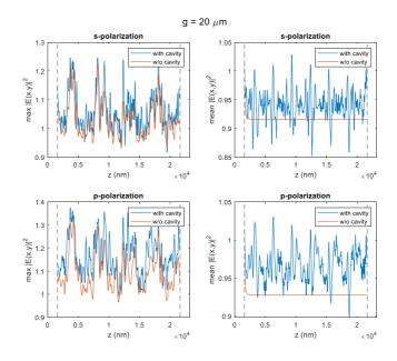
Figure 99. Maximal and mean electric energy distribution calculated for two model structures for distance between valves  $g=20~\mu m$  for S- and P- polarizations.
