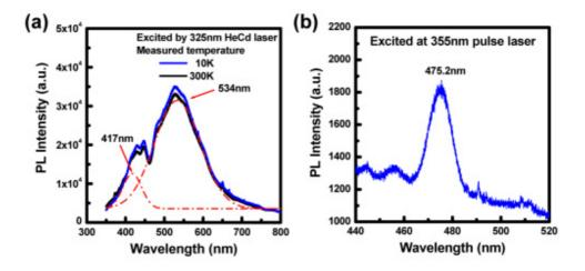
Figure 21. The micro-photoluminescence spectra of diatom frustule were measured by: a) 325 CW laser and b) 355nm pulse laser acted the excitation laser sources. Adopted from Ref.<sup>85</sup>. Reproduced with permission from Optica Publishing Group.
