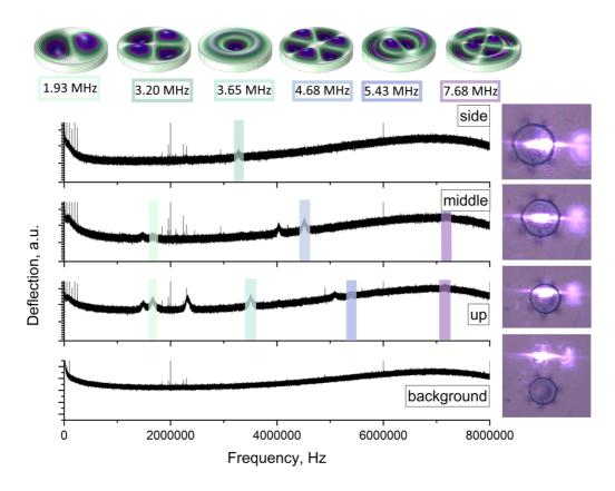
Figure 95. Raw spectra of frequencies of thermal vibrations of the diatom frustule collected at different spots.
