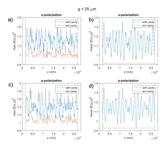
Figure 82. Maximal electric energy distribution calculated for two model structures for distance between valves g=25µm: a) S- and c) P- polarizations. Mean electric energy distribution calculated for: b) S- and d) P- polarizations.
