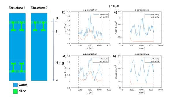
Figure 81. a) Two model structures: 1 - with cavity and 2 - without cavity for distance between valves g=5μm. Maximal electric energy distribution calculated for: b) S- and d) P- polarizations. Mean electric energy distribution calculated for: c) S- and e) P- polarizations.
