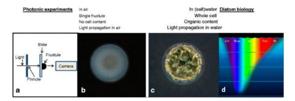
Figure 14. Overview of relevant features that differ between the diatom in its natural habitat and rinsed diatom valve measured using an optical setup (a). b) A diatom valve rinsed of organic material, c) A living diatom in water, d) A mapping showing how spectrum of transmitted light changes with depth. Adopted from Ref.<sup>65</sup>. Reproduced with permission from Springer Netherlands.
