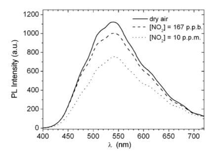
Figure 20. *Thalassiosira* photoluminescence spectrum in dry air (continuous line), in 167 ppb of NO<sub>2</sub> in dry air (dashed line) and in 10 ppm of NO<sub>2</sub> in dry air (dotted line). Adopted from Ref<sup>82</sup>. Reproduced with permission from Elsevier Ltd.
