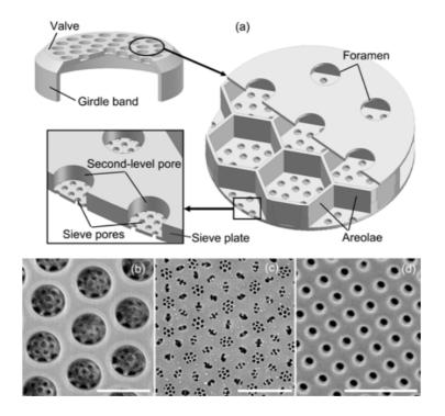
Figure 8. Typical structure of multilevel pores (Coscinodiscus sp.). a) 3D model; b) arrays of foramen and second-level pores, scale bar 1  $\mu$ m; c) array of sieve pores, scale bar 2  $\mu$ m; d) array of nanopores on girdle band, scale bar 1  $\mu$ m. Adopted from Ref.<sup>28</sup>. Reproduced with permission from Springer.
