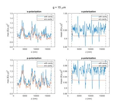
Figure 98. Maximal and mean electric energy distribution calculated for two model structures for distance between valves  $g=15~\mu m$  for S- and P- polarizations.
