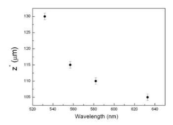
Figure 16. Distance z\* of maximum intensity of the transmitted spot as a function of the wavelength of the incoming light beam. Adopted from Ref.<sup>74</sup>.
