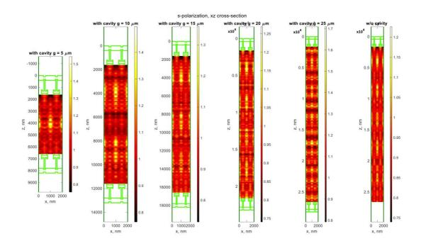
Figure 104. Electric field intensity calculated for S-polarization within vertical cross-sections of samples with height g=5, 10, 15, 20, 25  $\mu$ m in xz plane.
