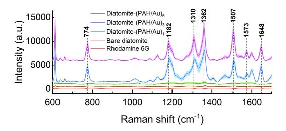
Figure 89. Surface-enhanced Raman spectra of Rhodamine 6G obtained using gold-coated diatomite hybrid materials with a different number of PAH/AuNPs bilayers.
