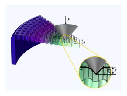
Figure 61. The deformation response of the frustule valve to local indentation
