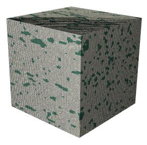
Figure 43 – Voxel model created with VoxTex software with green as fibre and white as matrix
