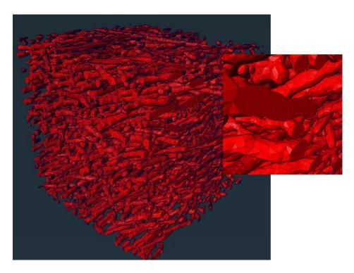
Figure 44 - FE model of fibres created using Avizo software
