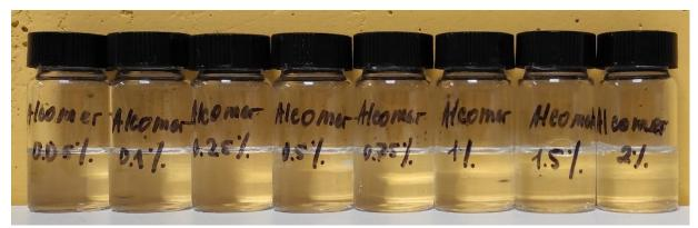
Appearance of surfactant solutions with the addition of Alcomer DP 1 after 14 days of heating at  $70^{\circ}$ C
