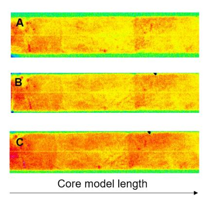
Figure 59. 2D fluid distribution in core model (a) after water flooding, (b) after surfactant flooding, (c) after 48-hour shutdown. Yellow – oil, red – water phase
