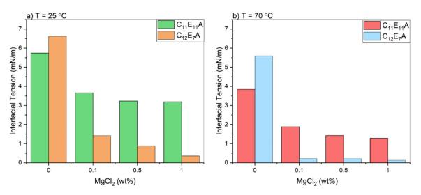
Figure 23. The interfacial tension as a function of MgCl<sub>2</sub> concentration for  $C_{12}E_7A$  and  $C_{11}E_{11}A$  at 25 (a) and 70°C (b)
