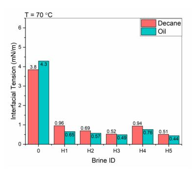
Figure 29. IFT of C<sub>11</sub>E<sub>11</sub>A (0.25 wt%) on the boundary with oil and n-decane at 70°C as a function of hard brine type. All brines are characterized in Table 5
