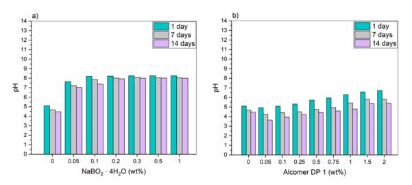
Figure 63. pH values of sodium metaborate tetrahydrate (a) and Alcomer DP 1 (b) in 1 wt% surfactant solution in brine
