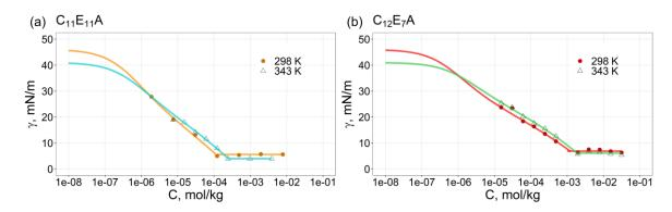
Figure 31. Experimental isotherms for  $C_{11}E_{11}A$  (a) and  $C_{12}E_{7}A$  (b) fitted with the RP model. Filled circles: T = 298 K; open triangles: T = 343K
