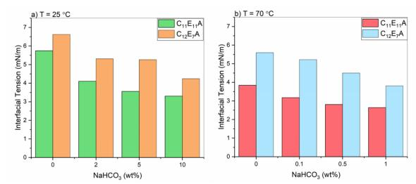
Figure 27. The interfacial tension as a function of NaHCO<sub>3</sub> concentration for  $C_{12}E_7A$  and  $C_{11}E_{11}A$  at 25 (a) and 70°C (b)
