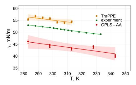
Figure 30. Validation of TraPPE-UA+TIP4P/2005 model and OPLS-AA+TIP3P water model by decane—water system, experimental data from
