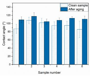
Figure 41. Contact angle values of initial core samples and aged in oil (rock-water-air contact, ambient conditions)
