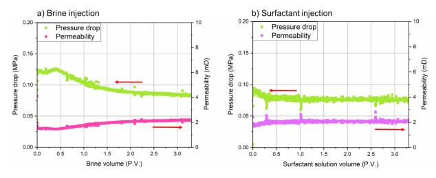
Figure 57. Pressure drop dynamics during oil displacement by (a) brine and (b) surfactant solution (Q = 0.1 mL/min)
