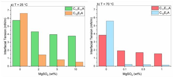
Figure 26. The interfacial tension as a function of MgSO<sub>4</sub> concentration for  $C_{12}E_7A$  and  $C_{11}E_{11}A$  at 25 (a) and 70°C (b)
