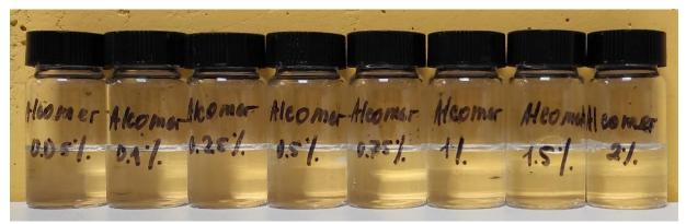
Appearance of surfactant solutions with the addition of Alcomer DP 1 after 14 days of heating at  $70^{\circ}\mathrm{C}$
