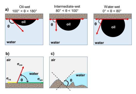
Figure 5. Wettability of reservoir rock based on contact angle measurements: (a) rock-water-oil contact; (b) rock-water-air contact; (c) contact line on a rough surface. Modified after [27,28,30,33]
