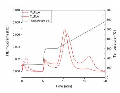
Figure 44. Pyrograms of surfactants on pure calcite (calcined at 550°C)
