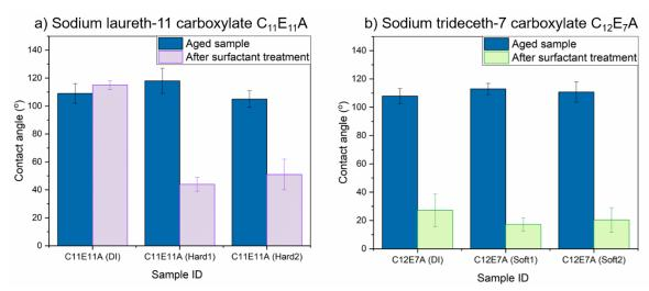
Figure 42. Contact angles values before and after treatment with surfactant compositions: (a)  $C_{11}E_{11}A$ , (b)  $C_{12}E_{7}A$  (rock-water-air contact, ambient conditions)
