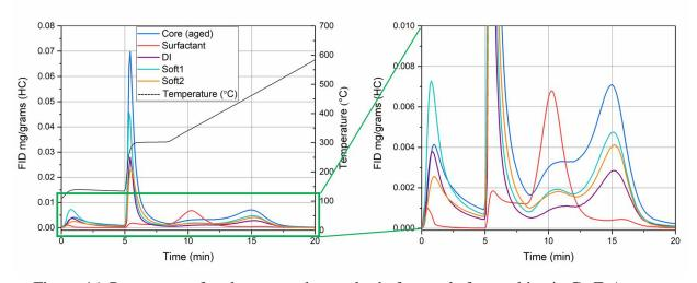
Figure 46. Pyrograms of carbonate rock samples before and after soaking in C<sub>12</sub>E<sub>7</sub>A surfactant solutions
