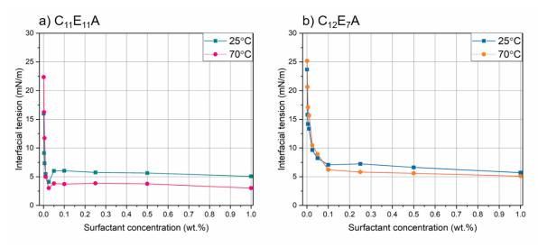
Figure 19. IFT profiles of (a) C<sub>11</sub>E<sub>11</sub>A and (b) C<sub>12</sub>E<sub>7</sub>A in DI water at 25 and 70°C
