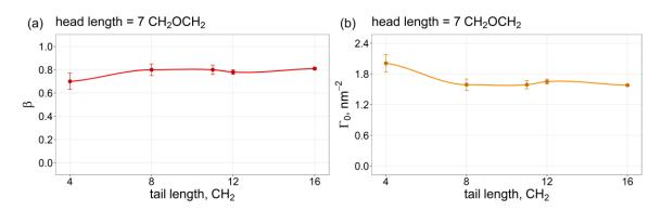
Figure 35. The dependence of the adsorption parameter  $\beta$  (a) and the adsorption limit  $\Gamma_0$  (b) on the hydrophobic alkyl tail length n of the AEC surfactants at constant ethyleneoxide segment length of 7 monomers
