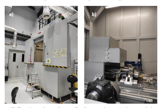
Figure 53. Experimental setup for core flooding experiment: (a) the general view, (b) core holder with X-ray scanner
