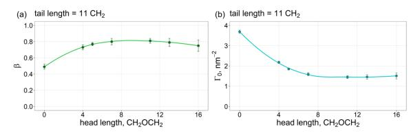
Figure 34. The dependence of the adsorption parameter  $\beta$  (a) and the adsorption limit  $\Gamma_0$  (b) on the hydrophilic ethyleneoxide segment m of the AEC surfactants with the same alkyl tail length ( $C_{11}$ ). The adsorbed monolayer becomes less compressible and the maximum adsorption decreases with m until the segment reaches approximately 8 ethyleneoxide monomers. At higher m, both  $\beta$  and  $\Gamma_0$  become independent of the segment length
