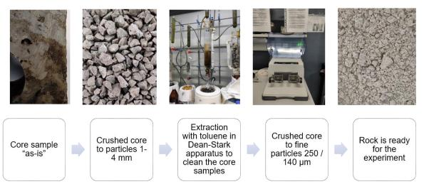
Figure 37. Methodology of limestone rock powder preparation
