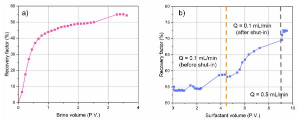
Figure 60. Brine (a) and surfactant (b) flooding RF profiles determined through X-ray saturation control
