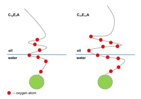
Figure 20. Schematic orientation of C<sub>12</sub>E<sub>7</sub>A and C<sub>11</sub>E<sub>11</sub>A on oil-water interface
