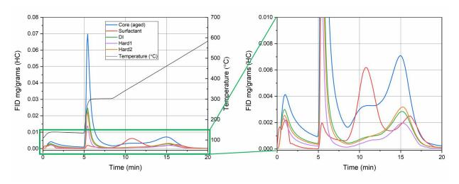
Figure 45. Pyrograms of carbonate rock samples before and after soaking in C<sub>11</sub>E<sub>11</sub>A surfactant solutions
