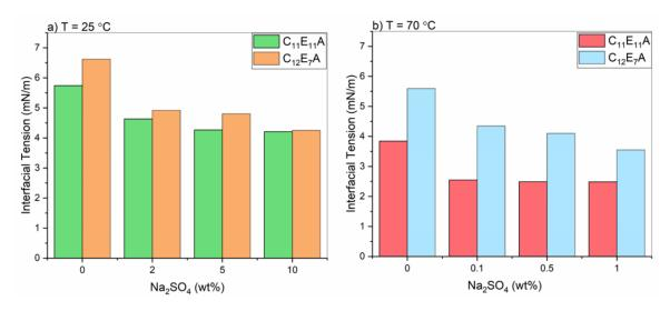
Figure 25. The interfacial tension as a function of  $Na_2SO_4$  concentration for  $C_{12}E_7A$  and  $C_{11}E_{11}A$  at 25 (a) and 70°C (b)
