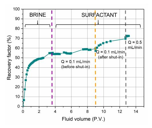
Figure 61. General RF determined through X-ray saturation control
