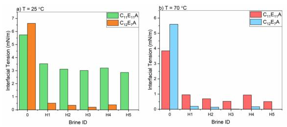
Figure 28. The interfacial tension as a function of hard brine type for C<sub>12</sub>E<sub>7</sub>A and C<sub>11</sub>E<sub>11</sub>A at 25 (a) and 70°C (b). All brines are characterized in Table 5
