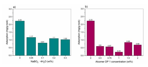
Figure 69. Static adsorption values of AEC surfactant in the presence of sodium metaborate tetrahydrate (a) and Alcomer DP 1 (b)
