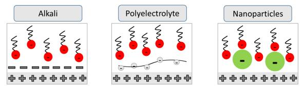
Figure 12. Mechanism of different adsorption inhibitors action
