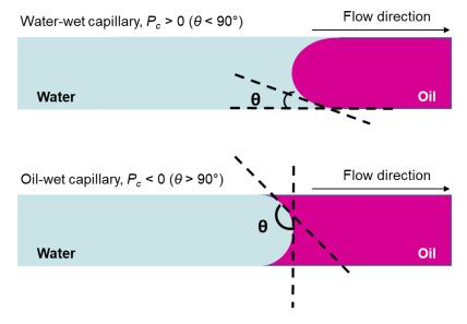
Figure 6. A simplified demonstration of water displacing oil in hydrophilic and hydrophobic channels. Modified after [36]
