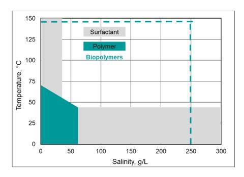
Figure 9. Salinity-temperature cross plot to compare conditions of offshore fields to market available surfactants and polymers. Redrawn from [57]
