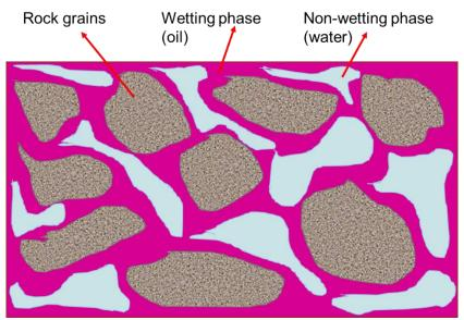
Figure 4. Pore cross section with distribution of wetting and non-wetting phase. Modified from [12]
