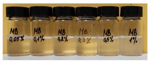
Appearance of surfactant solutions with the addition of sodium metaborate tetrahydrate after 14 days of heating at  $70^{\circ}$ C
