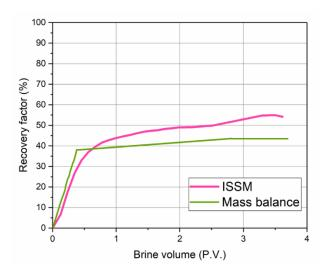
Figure 62. Comparison of recovery factor profiles obtained through ISSM and mass balance methods
