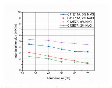
Figure 17. Interfacial tension of  $C_{11}E_{11}A$  and  $C_{12}E_{7}A$  on the boundary with n-decane as a function of temperature (the concentration of surfactant in each solution is 1 wt%)
