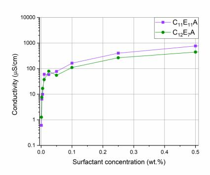
Figure 18. Conductivity versus surfactant concentration at room temperature
