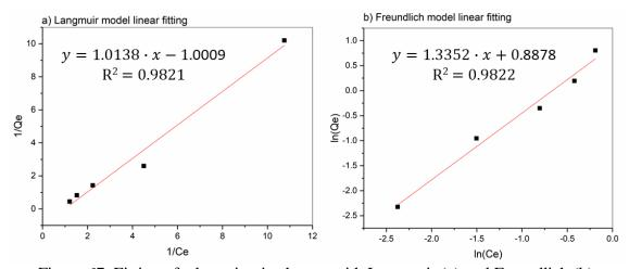
Figure 67. Fitting of adsorption isotherms with Langmuir (a) and Freundlich (b)
