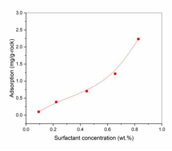
Figure 65. Adsorption isotherm of surfactant (Equilibrium adsorption profile)
