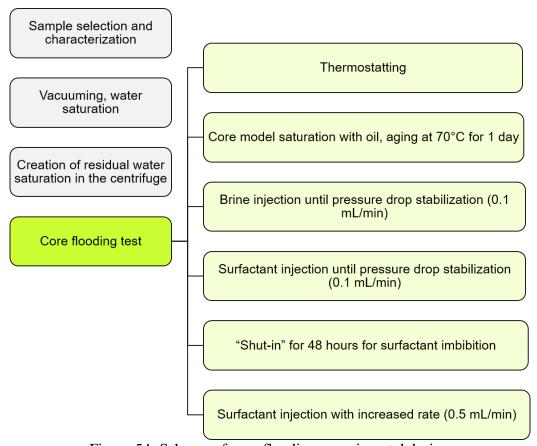
Figure 54. Scheme of core flooding experimental design
