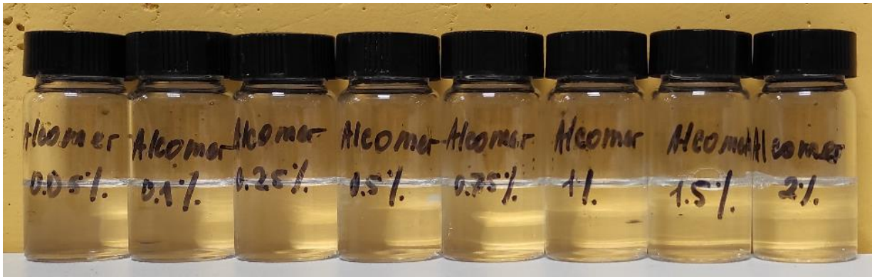
Appearance of surfactant solutions with the addition of Alcomer DP 1 after 14 days of heating at 70°C
